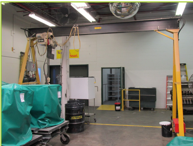
MTC 6000LB A-FRAME FREE STANDING CRANE W/ CUFFING 3-TON ELECTRIC CHAIN HOIST
