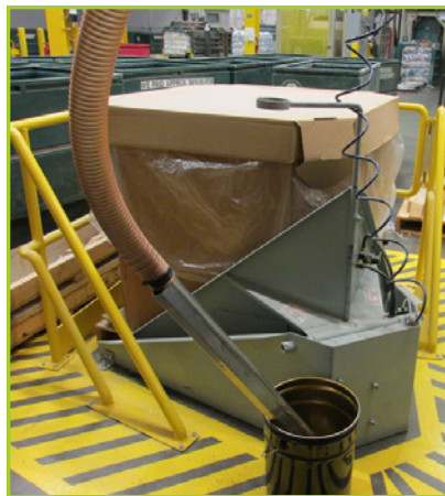
MOTAN PELLET TRANSPORT SYSTEM, W/ BOX TILTER, BLOWER, FEED HOPPER, BUSH MINK PUMP. YEAR 2011
