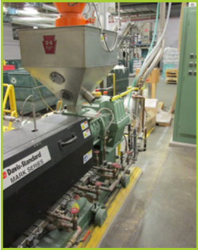
DAVIS-STANDARD MARK V WATER COOLED EXTRUDER, 75MM, 34:1 L/D, W/ DAVIS-STANDARD EPIC III CONTROLS, ADVANTAGE MAXIMUM 2000LE PORTABLE CHILLER. YEAR 2011
