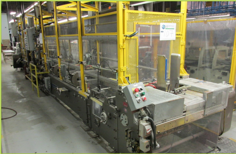
WESTERN SLOPES KF ROYAL 333 FLAME SEALER , LINE SPEED 1,500 BFPM, CARTON RANGE LENGTH 2.5" TO 33", CARTON RANGE WIDTH 7.25" TO 33". YEAR 2006
