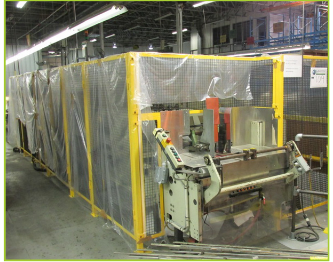
JAGENBURG 105-1U STRAIGHT LINE GLUER , LINE SPEED 1.300 BFPM, CARTON RANGE LENGTH 3" TO 48.25", CARTON RANGE WIDTH 2" TO 48.25". YEAR 1989
