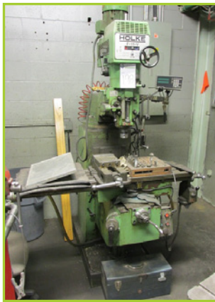
HOLKE F-11-V VERTICAL MILLING MACHINE, W/ACU-RITE CONTROLS
