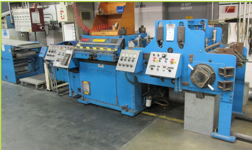
CHESNUT 150 ROTOGRAVURE PRINTING PRESS W/ IN-LINE ROTARY DIE CUTTER & KEMPSMITH PLATEN, CALIPER RANGE 30# PAPER - .024", 7" TO 15" MATERIAL RANGE, LINE SPEED 140 METERS/MIN (459 FT/MIN), MAX ROLL OD 60", CORE ID 12", 8-STATIONS, 2-REVERSIBLE STATIONS, ELECTROSTATIC STATIONS; 1,2,3,4,5,6,7 , CYLINDER REPEAT RANGE 10" TO 20", EXTENDED DRYER AFTER STATION 8 UV COATING CAP., 72" GAS OVEN, REGISTER CAP. P/P ± .008", P/C AND P/E ± .020", (REGISTRON S2000) MARTIN ROLLSTAND, ROTARY EMBOSING, BUTT SPLICER, CHESNUT SPARE PARTS, CHESTNUT ROLLS, CHESTNUT INK POTS & PARTS, PRIME UV DRYING SYSTEM. YEAR 1987
