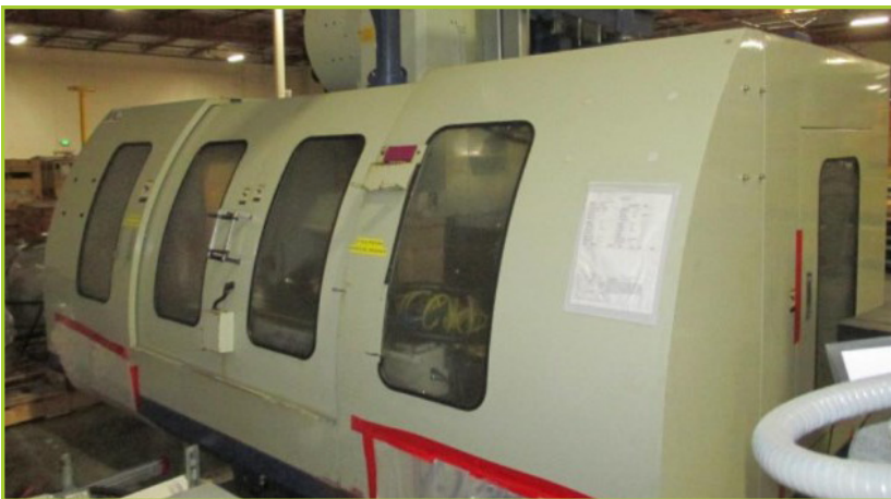
VIPER VMC-1230 CNC VERTICAL MACHINING CENTERS. SPECS: X-AXIS TRAVEL 50", Y-AXIS TRAVEL 25", Z-AXIS TRAVEL 25"; TOOL POSITIONS 20 ATC; SPINDLE SPEED 6000 RPM, SPINDLE TAPER 50 TAPER; HORSE POWER 20 HP; WGT. 23,700 LBS
