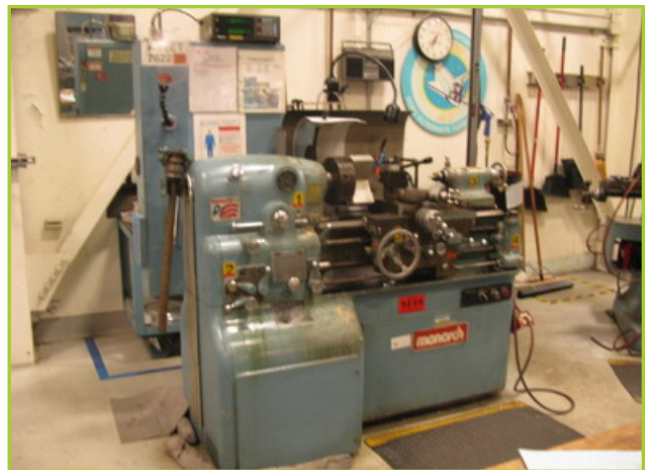
MONARCH 10EE TOOLROOM LATHE, 12-1/2" X 20", 460VAC, 3-PHASE, 60 HZ, 13 AMP, (1990)
