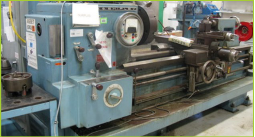
LODGE & SHIPLEY 2013/17 LATHE, 24" X 83", W/ SONY DIGITAL READOUT, 2 CHUCKS - 4-JAW & 3-JAW
