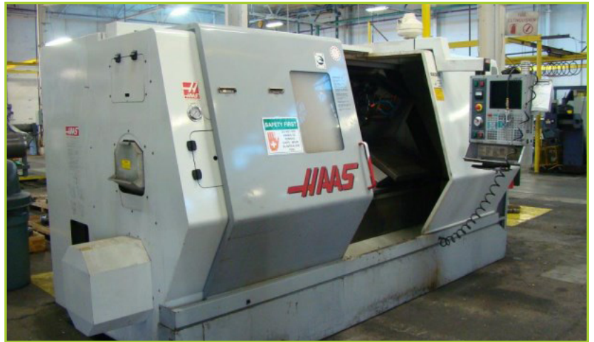
HAAS SL-40 HAAS 2-AXIS SLANT BED CNC LATHE, 15" MMK POWER CHUCK. AUTOMATIC CHIP CONVEYOR 10 STATION TURRET, DIMS 190" L X 92" W X 89" H, WGT 25,000 LBS. MFG 2001
