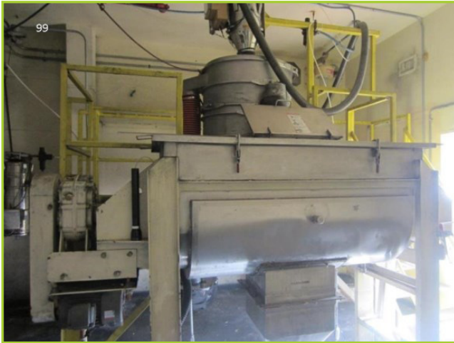
RIBBON BLENDER, STAINLESS STEEL. INSIDE MEASURES 2 FEET 2-1/16 INCHES WIDE BY 5 FEET 5-29/32 INCHES LONG
