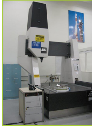
CINCINNATI MILACRON G80 LK MICROVECTOR BRIDGE TYPE CMM MACHINE, 3 AXIS
