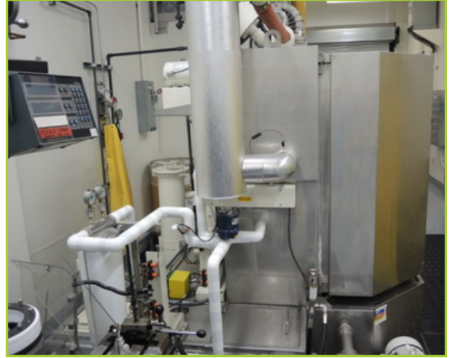
PROCECO LTD. PC 42X42-E-1000-2-RD-HBO-SS PARTS WASHER, TANK 1 VOLUME - 165 GAL, TANK 2 VOLUME - 45 GAL, 7'-6" W X 8'-3" L X 8'-3" H, 1000LB MAX. LOAD CAP, (2011)
