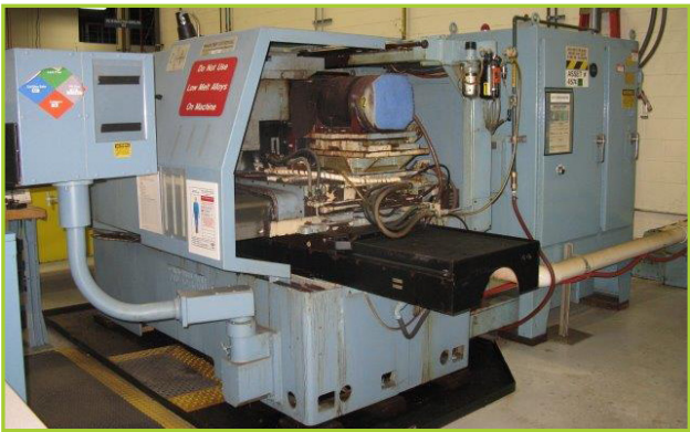
CINCINNATI MILACRON HEALD 2EF CINTERNAL CNC MULTI SURFACE GRINDER, SWING OVER TABLE 28", SWING W/ WORK HEAD @ 90 DEGREE- 17", GRINDING STROKE 17", TRAVEL 20", CROSS SLIDE 9", WORK SLIDE 16"
