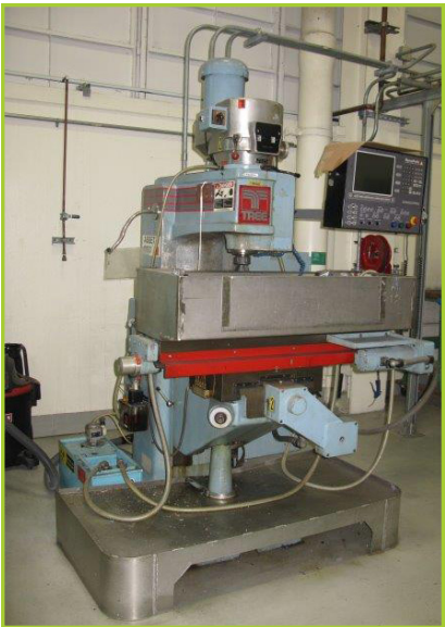
TREE MACHINE JOURNEYMAN 310 CNC TREE MILL- ING MACHINE, 3-AXIS, X-27", Y-14", Z-5", 10" X 44" TABLE,60-4200 RPM SPINDLE SPEED, (1995)
