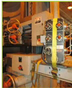
BULLARD 75 CUTMASTER 66" VERTICAL TURRET LATHE. CHUCK DIAMETER: 36", MAX SWING (SIDE HEAD DOWN): 45" / (SIDE HEAD UP) 39", TURRET TO TABLE: 46", MAIN MOTOR: 40HP, TABLE SPEED: 10-375 RPM; POWER: 480V / 3PH / 6HZ, APPRX DIMENSIONS: 9'X 9'X 13'H, APPRX WEIGHT: 38,000 LBS
