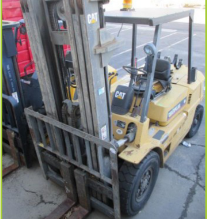
CATERPILLAR GP40 HEAVY DUTY GAS-POWERED FORKLIFT, TYPE G 6200LBS LOA
