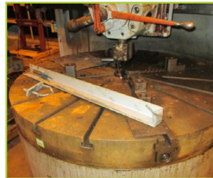
BULLARD 75 CUTMASTER 66" VERTICAL TURRET LATHE. CHUCK DIAMETER: 36", MAX SWING (SIDE HEAD DOWN): 45" / (SIDE HEAD UP) 39", TURRET TO TABLE: 46", MAIN MOTOR: 40HP, TABLE SPEED: 10-375 RPM; POWER: 480V / 3PH / 6HZ, APPRX DIMENSIONS: 9'X 9'X 13'H, APPRX WEIGHT: 38,000 LBS
