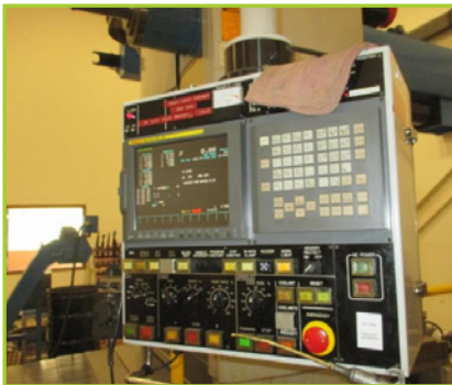
IKEGAI NB 130P CNC HORIZONTAL BORING MILL. MAIN AXIS: O130, MAIN MOTOR: AC22/18.5KW; 10T OF TABLE LOADING WEIGH; CAPACITY: 22,000 LBS., SPINDLE DIAMETER: 5.12", SPINDLE SPEED: 5-2,500 RPM, SPINDLE TORQUE: 2793 FT/LBS., AXIS TRAVEL: X - AXIS (CROSS) 137.8" / 98.42" / 63" / 27.5" / .001 (360,000); AUTOMATIC TOOL CHANGER CAPACITY: 60 TOOLS; MAX. TOOL DIA: 5.52", MAX TOOL LENGTH: 15.75", MAX TOOL WEIGHT: 55 LBS. MACHINE WEIGHT: 80,000 LBS; BUILT IN 2000. INCLUDES: FANUC SERIES 16I-M (4AXIS) CONTROL MODULE, 5-TON OVERHEAD CRANE AND CHIP CONVEYOR
