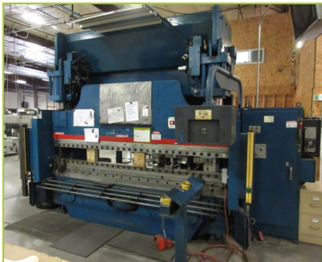
CINCINNATI 175 AF 8 175-TON X 10' AUTOFORM CNC PRESS BRAKE , (1996), STROKE LENGTH 254 MM, MAX. PRESSURE 24.82 MPA 36000 PSI, POWER CLAMP CONTROL, REMOTE MANUAL RAM POSITIONING AND GAGE CONTROL, TWO-HAND OPERATOR STAND, LIGHT CURTAIN, FOOT SWITCH
