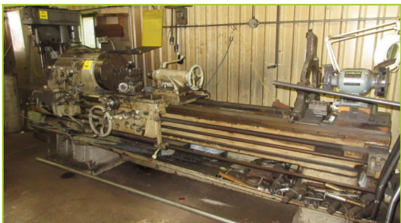
MONARCH 16" CW ENGINE LATHE , (1942), ACTUAL SWING 18.5, DISTANCE BETWEEN CENTERS 78"
