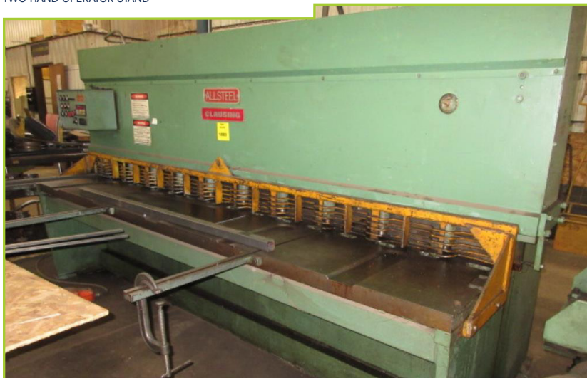
ALLSTEEL CLAUSING 1/4-10MAXI 10' SQUARING SHEAR , 15-HP, 1/4" CAPACITY MILD STEEL, 3/16" STAINLESS STEEL, MICRO-WIZ PROGRAMMABLE CONTROL, 72" SQUARING ARM, POWER BACK GAGE, FOOT SWITCH
