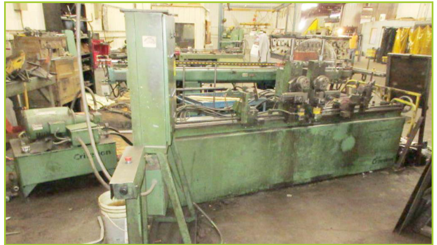
CRITERION HYDRAULIC BENDER, RACINE 20-HP HYDRAULIC UNIT, TOOLING NOT INCLUDED
