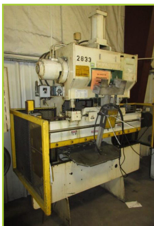
WYSONG H-2072 20-TON X 6' PRESS BRAKE , SHUT HEIGHT 9", STROKE 2-1/2", ADJUSTMENT 3", TWO-HAND OPERATOR STAND, STI OPTOSAFE LIGHT CURTAIN
