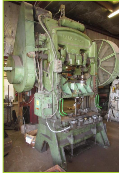
TOLEDO 92 1/2C PRESS, MAX SLIDE ADJUSTMENT 2 5/8, BED SIZE 48 X 32, AIR CLUTCH
