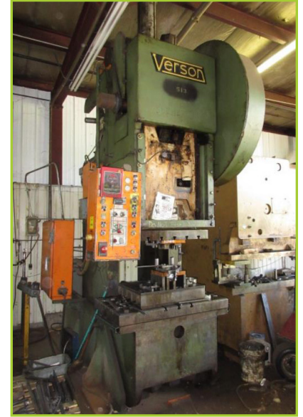
VERSON 150 150-TON OBI PUNCH PRESS, 8" STROKE, 45 SPM, SHUT HEIGHT 22, RAM ADJUSTMENT 6
