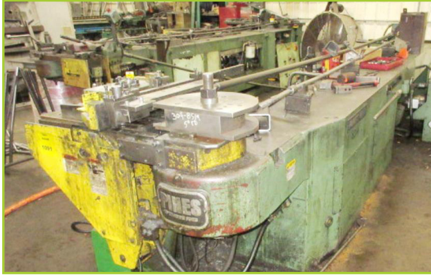
PINES NO. 2 HYDRAULIC BENDER, PROGRAMMABLE CONTROL WITH STAND
