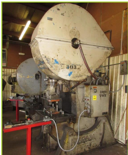
NIAGARA NO. A5 100-TON OBI PUNCH PRESS , BED SIZE 39 X 25, AIR CLUTCH, AIR CUSHION, GROUND INDICATOR, TWO-HAND OPERATOR STAND
