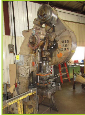
BLISS 5.5 50-TON OBI PUNCH PRESS, BED SIZE 30 X 19, GROUND INDICATOR, TWO-HAND OPERATOR STAND
