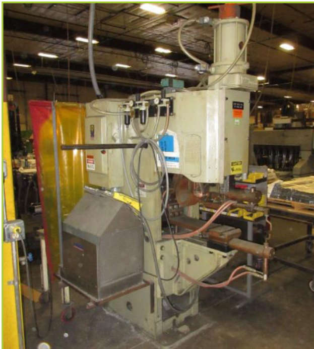
TAYLOR WINFIELD 100 KVA SPOT WELDER, THROAT 36", MODEL 108-2 WELD CONTROL
