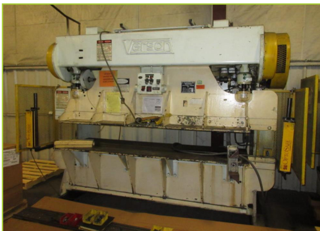
VERSOLLSTEEL 50-TON X 8' PRESS BRAKE , SHUT HEIGHT 12, STROKE OF RAM 2-1/2, ADJUSTMENT OF RAM 4, STI OPTOSAFE LIGHT CURTAIN
