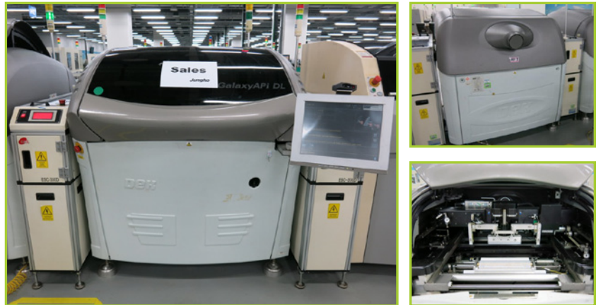
DEK GALAXY API DL SCREEN PRINTER, S/W VER. 09 SP06 P06; HAWKEYE CAMERA; INSPECTION: ADVANCED; SQUEEGEE: 200MM; USC: CYCLONE; VACUUM SUPPORT SYSTEM; DUAL LANE. MANUFACTURED IN 2008
