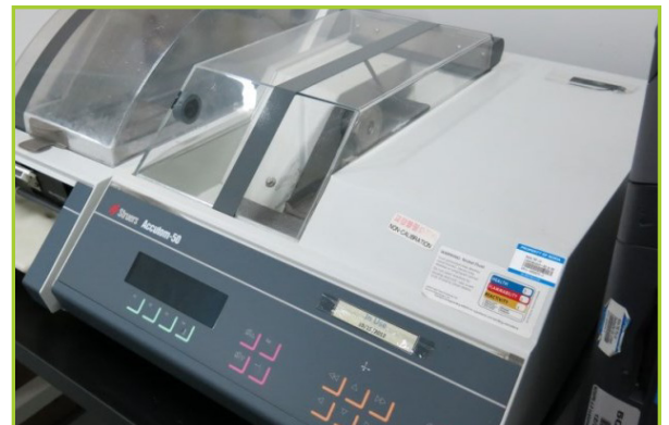
STRUERS ACCUTOM-50 PRECISION TABLE TOP CUT-OFF MACHINE AND GRINDING MACHINE FOR PRECISE AND DEFORMATION-FREE CUTTING, 2001
