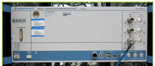
ROHDE & SCHWARZ CMW500 SOFTWARE OPTIONS: KB036 6GHZ ENABLING, KM011 IQ VS SLOT TX MEAS, KM012 MULTI EVAL LIST MODE, KM200 GSM TX MEAS / GSM R6 TX MEAS, KM400 WCDMA TX MEAS / WCDMA R99 TX MEAS, KM500 LTE FDD R8 TX MEAS, ; HARDWARE OPTIONS: CONTROLLER FMR9/5 H051F, 100457
