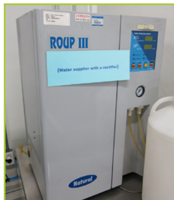
NATURAL ROUP III COMMON PURE WATER GENERATOR, 1999
