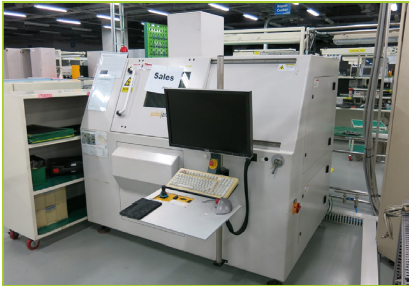
PHOENIX PCBA/ANALYSER 160 PHOENIX, X-RAY SYSTEMS PCBA ANALYSER 160 (2008) CE, 230 V 50/60HZ, 2000 VA, MAX. TUBE VOLTAGE: 160 KV MAX. OUTPUT: 320 W, DETAIL DETECTABILITY: UP TO 1 M, MIN. FOCUS-OBJECT-DISTANCE : 4.5 MM, GEOMETRIC MAGNIFICATION: (2D) UP TO 170-FOLD
