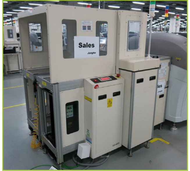
EUNIL ELD-500N MAGAZINE LOADER, LENGTH (MM) 380; MIN WIDTH 30 (MM); MAX WIDTH 250 (MM); SINGLE LANE, MANUFACTURED IN 2000
