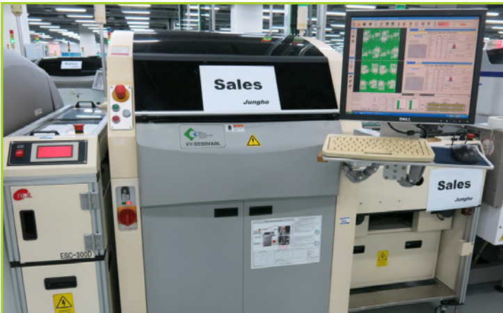
KOH YOUNG KY-3030VADL 3D IN-LINE SPI, S/W VER: 3.6.2301P25; RESOLUTION: 4M; PCB WIDTH (MM): 70-215; DUAL LANE, MANUFACTURED IN 2007
