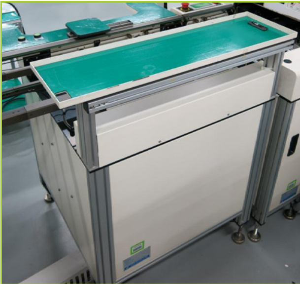
EUNIL EWT-100D INSPECTION CONVEYOR, LENGTH (MM) 850; MIN WIDTH 30 (MM); MAX WIDTH 205 (MM); DUAL LANE
