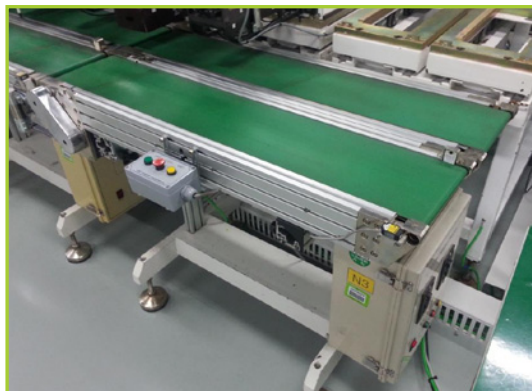
DAEHO TDK FLAT BELT CONVEYOR, LENGTH (MM) 1000; MAX WIDTH 180 (MM) ; DUAL LANE
