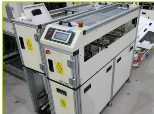
EUNIL ESC-300D SLIDER CONVEYOR, LENGTH (MM) 300; MIN WIDTH 30 (MM); MAX WIDTH 205 (MM); DUAL LANE, 2007
