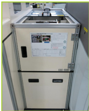
EUNIL ESC-300D LOADER CONVEYOR, LENGTH (MM) 530; MIN WIDTH 30 (MM); MAX WIDTH 205 (MM) ; DUAL LANE
