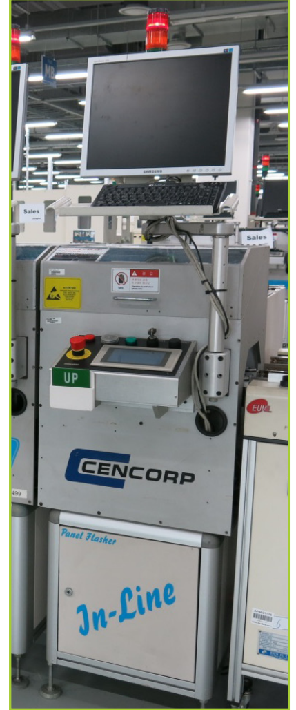
FLASH PROGRAMMER / IN-LINE TESTER CONFIGURED WITH ADVANTECH ACP 4000, 4 USB SLTS, PANEL/PCB ADAPTER, 2 SERIAL PORTS, JOT POWER SUPPLY, NORTEL 24 PORT SWITCH HUB, INCLUDES KEYPAD DISPLAY, K20-1140 RIGHT/WRONG DIRECTION SENSOR, PANEL FLAS
