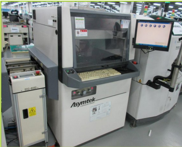
ASYMTEK X-1020 SOLDER PASTE DISPENSING; SV-100 SLIDER VALVE HEAD; TACTILE HEIGHT SENSOR; VISION SYSTEM; IMPINGEMENT HEAT CONVEYOR; PURGE, SCALE, DISPENSE CALIBRATION MODULE; DUAL LANE
