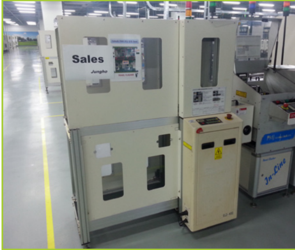
EUNIL ELD-400N MAGAZINE LOADER, LENGTH (MM) 380; MIN WIDTH 30 (MM); MAX WIDTH 250 (MM); SINGLE LANE
