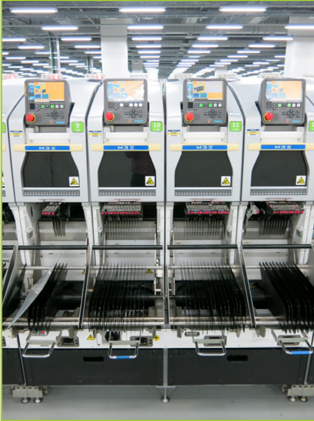
FUJI NXT 4M BASE W/ (4) M3S MODULES, S/W VER. V5.47; 4M INDEPENDENT BASE; PLACEMENT HEADS: (4) H12S; DUAL LANE; BUCKET TYPE FEEDER PALLET. S/N: 2958. MANUFACTURED IN 2006
