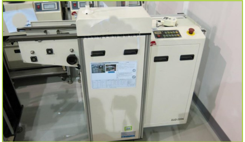
EUNIL EUD-200N MAGAZINE UNLOADER, LENGTH (MM) 530; MIN WIDTH 30 (MM); MAX WIDTH 250 (MM); SINGLE LANE, MANUFACTURED IN 2008
