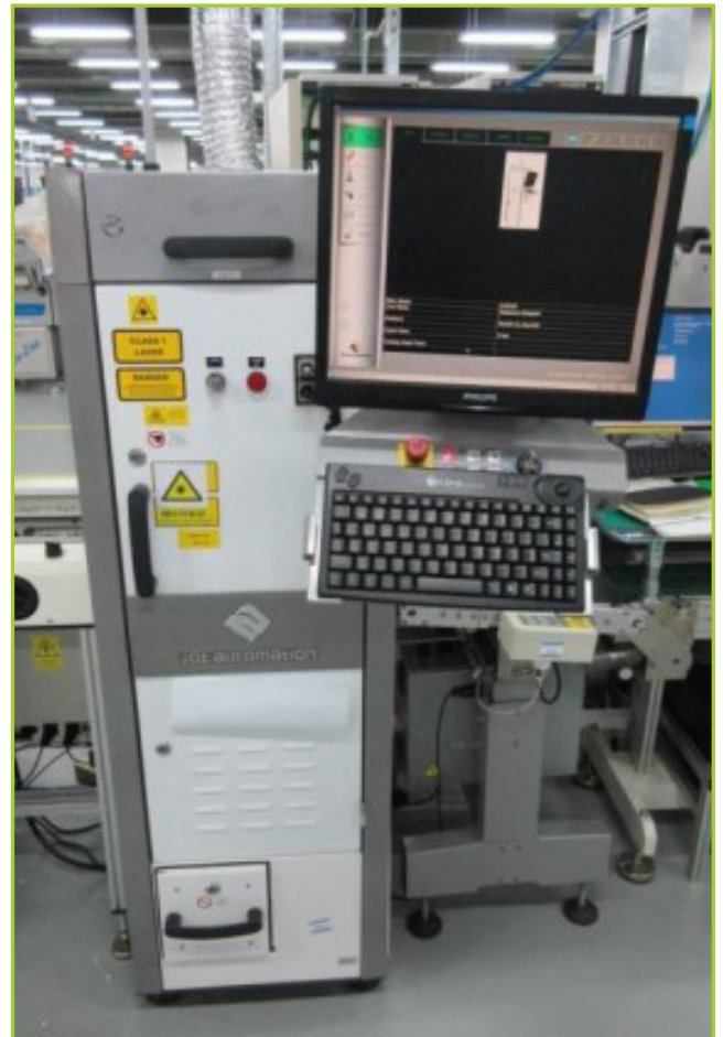
JOT 501-57.1/3 LASER DEPANELING CELL; CO2 LASER; SINGLE LANE; SMALL FOOTPRINT; HIGH OUTPUT; CUT/DEPANEL/SCRIBE BOARDS; UPGRADED WITH UPDATE KIT J005-785 IN NOV 2012
