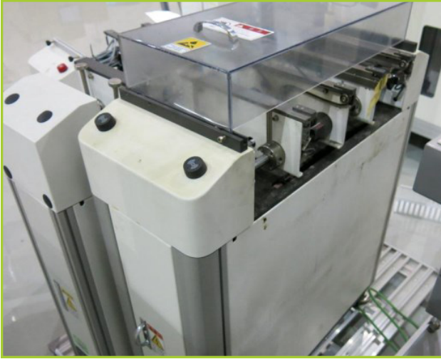
YOUNGJIN FA ACC-6CSD BUFFER CONVEYOR, LENGTH (MM) 200; MIN WIDTH 30 (MM); MAX WIDTH 230 (MM); DUAL LANE, MANUFACTURED IN 2011
