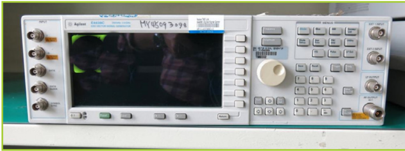
AGILENT E4438C SIGNAL GENERATOR, CHARACTERISTICS: 250 KHZ TO 1, 2, 3, 4, OR 6 GHZ (.01 HZ RESOLUTION) +17 DBM OUTPUT POWER, 160 MHZ RF MODULATION BANDWIDTH MODULATION AND SWEEP: AM, FM, \theta M, AND PULSE, ASK, FSK, MSK, PSK, QAM, CUSTOM I/Q, STEP, OR LIST, FREQUENCY
