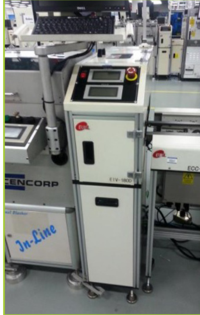
EUNIL EIV-180D INVERTER FLIP STATION, LENGTH (MM) 300; MIN WIDTH 30 (MM); MAX WIDTH 205 (MM); DUAL LANE, MANUFACTURED IN 2009
