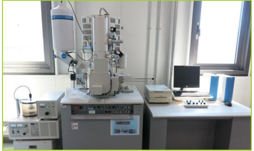
HITACHI S-4700 THE HITACHI S-4700 IS A FIELD EMISSION SCANNING ELECTRON MICROSCOPE (FE-SEM), UNDER OPTIMAL CONDITIONS, CAN MAGNIFY IMAGES UPWARDS OF 500,000 TIMES AND RESOLVE FEATURES TO 2 NANOMETERS. IN ADDITION, A CATHODOLUMINESCENCE DETECTOR, MANUFACTURED IN 2006.
