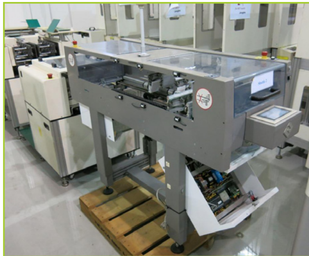
JOT SHUTTLE CONVEYOR, (MM) 500; MIN WIDTH 50 (MM); MAX WIDTH 205 (MM) ; TRIPLE LANE, MANUFACTURED IN 2008
