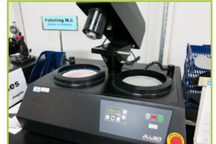
ALLIED DUALPREP 3 THE DUALPREP™ GRINDING/POLISHING MACHINES
