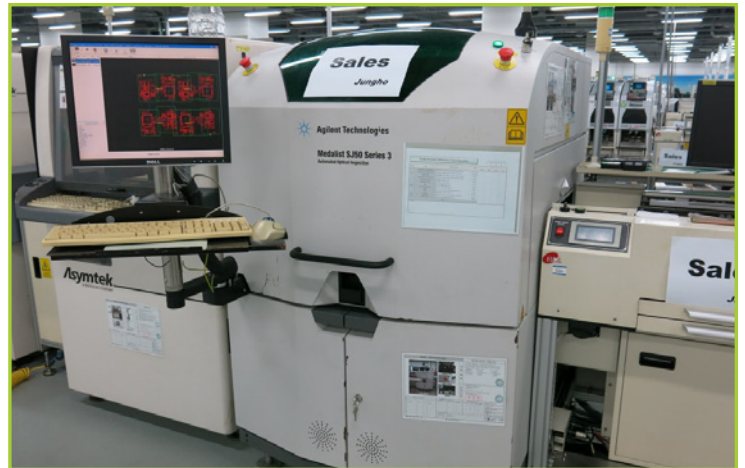
AGILENT SJ50 SERIES 3 IN-LINE AOI, S/W VER: 1.03.06; DUAL LANE, MANUFACTURED IN 2007
