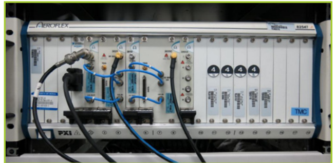
AEROFLEX 82547 18 SLOT PXI CHASSIS WITH MXI INTERFACE
