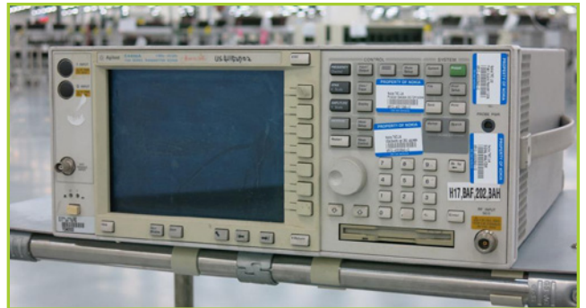
AGILENT E4406A FREQUENCY RANGE RF INPUT: 7 TO 314 MHZ AND 329 MHZ TO 4 GHZ, BASEBAND IQ INPUTS: 0 HZ TO 5 MHZ FREQUENCY SPANS: BASEBAND IQ INPUTS: 5 HZ TO 5 MHZ (BASEBAND I OR Q INPUTS) 10 HZ TO 10 MHZ (COMPOSITE I/Q), FREQUENCY SETTING RESOLUTION: 1 HZ RESIDUAL
