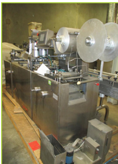
JIANGNAN PACKING DPP-250D II TYPE AUTOMATIC BLISTER PACKING MACHINE
