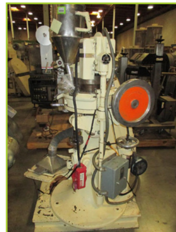
FJS ROTARY TABLET PRESS, 16 STATION
