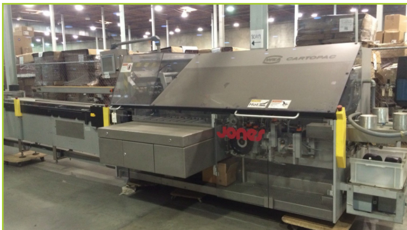
JONES / IWKA CARTOPACK SC4 HORIZONTAL CARTONER WITH BOTTLE KNOCK DOWN WHEEL, ALLEN BRADLEY 1500P VERSAVIEW, PLC, NORDSON VISTA GLUE SYSTEM
