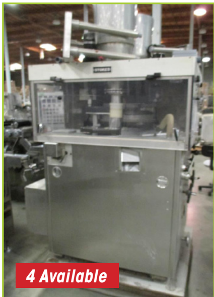
STOKES 328-1 ROTARY TABLET PRESS , 35 STATION, 10 TON COMPRESSION
