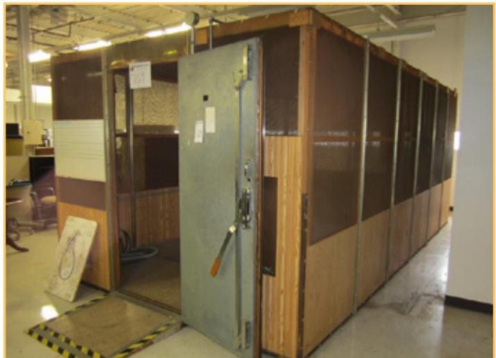
CUSTOM RF CAGE (FOR BLOCKING RF SIGNALS) 20' X 10'
