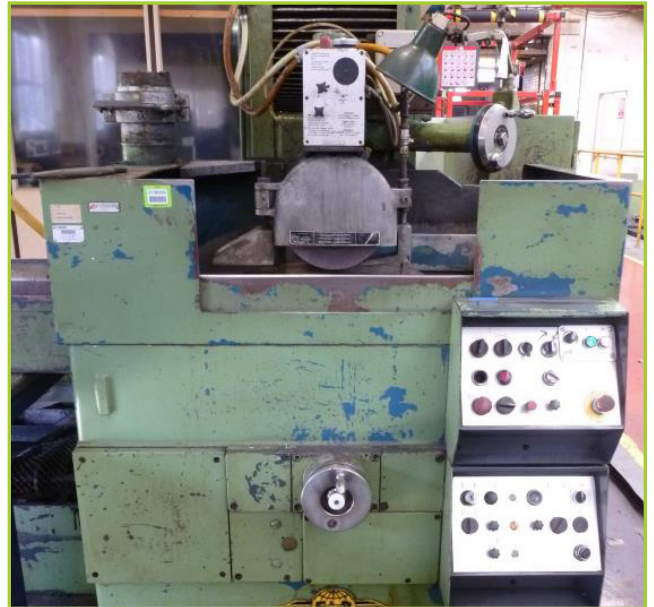
ELB SW240YAH HORIZONTAL SURFACE GRINDER WITH 500MM DIA MAG CHUCK, COOLANT PUMP & TANK
