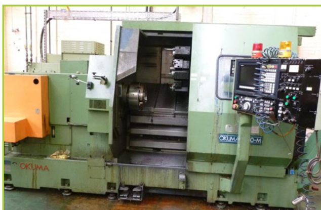
OKUMA LC40 M CNC TURNING CENTRE/LATHE 12 & 8 STATION TC, OKUMA ROBOT PANEL 5000S CONTROLS, TOUCH SETTER SENSOR CONTACT, SWARF CONVEYOR. TWIN TURRET WITH LIVE/DRIVEN TOOLS, (1) AUTO CHUCK
