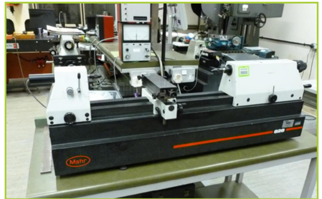
MAHR 828 CENTRES MEASURING MACHINE BENCH TYPE, 500MM BETWEEN CENTRES, HEIDENHAIN CONTROL & 2 X MAHR LENGTH MEASURING INSTRUMENTS
