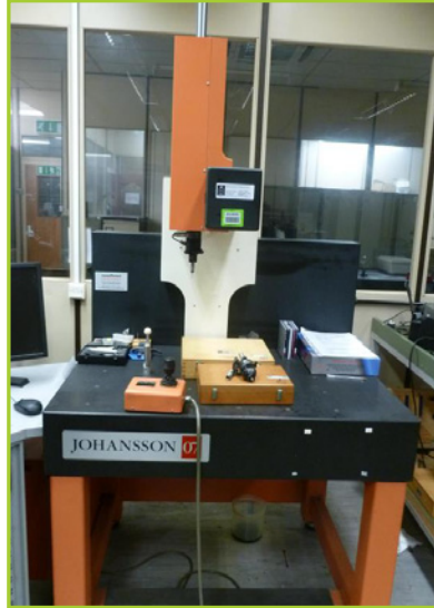
JOHANSSON 7 COORDINATE MEASURING MACHINE 681MM X 427MM X 295MM WITH JOYSTICK CONTROL
