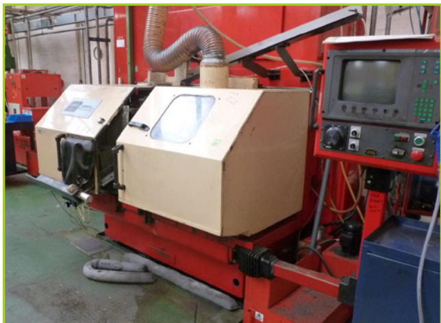
HEALD ATC ICF 91 CNC INTERNAL GRINDER INTERNAL CNC GRINDER FOR INTERNAL DIAMETERS RANGING FROM 7-100MM.
