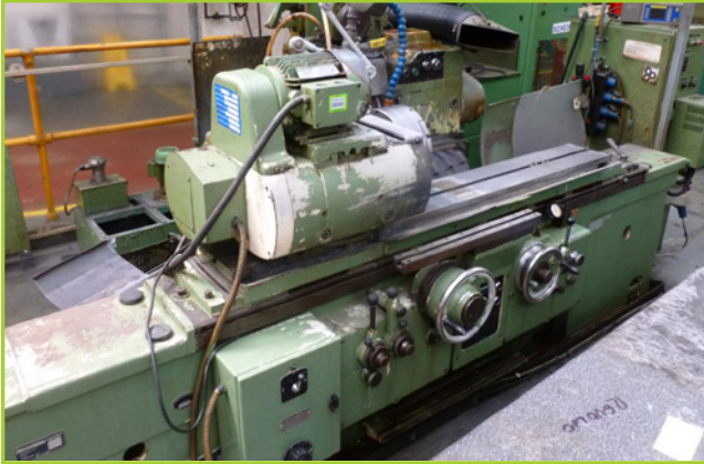
JOHANSSON 24-D EXTERNAL CYLINDRICAL GRINDER SBS BALANCE SYSTEM, 300MM MAG CHUCK, 1100MM BED, FSE 100LPM COOLANT MANAGEMENT SYSTEM, USED FOR DIAMETERS RANGING FROM 100MM - 400MM
