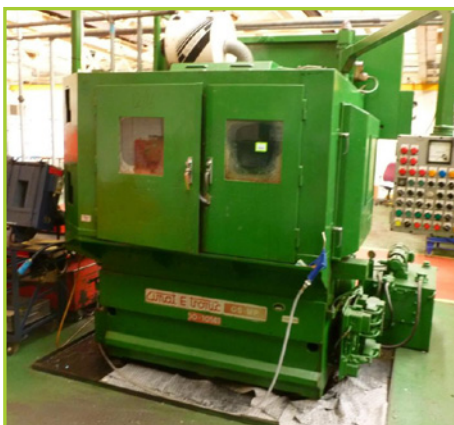
CIMAT E TRONIC EXTERNAL GRINDER EXTERNAL BALL RACE, GRINDING RADIUS OF 5-25MM AND DIAMETERS OF 12MM-150MM
