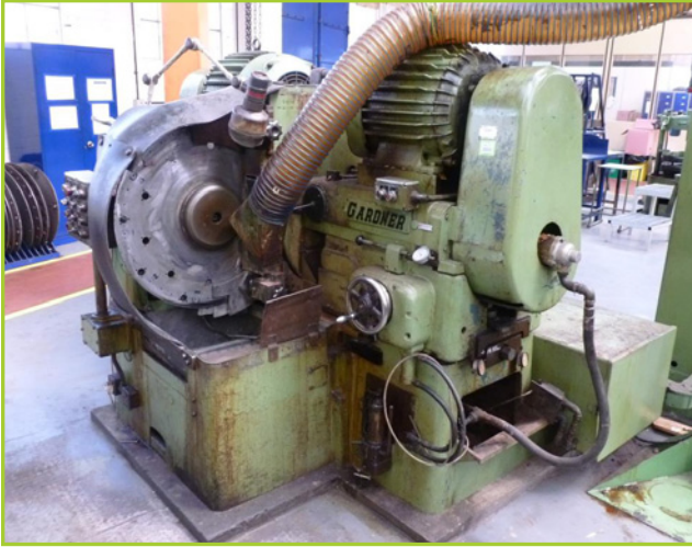
GARDNER VERTICAL END GRINDER 750MM WITH FILTRATION & COOLANT SYSTEM USED FOR GRINDING ROLLER FACES WITH DIAMETERS RANGING FROM 5MM- 30MM
