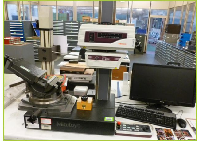
MITUTOYO CONTRACER CV4100 SURFACE CONTOUR MEASURING INSTRUMENT WITH C-4000 HEAD, REMOTE BOX, 24" X 18" GRANITE SURFACE TABLE
