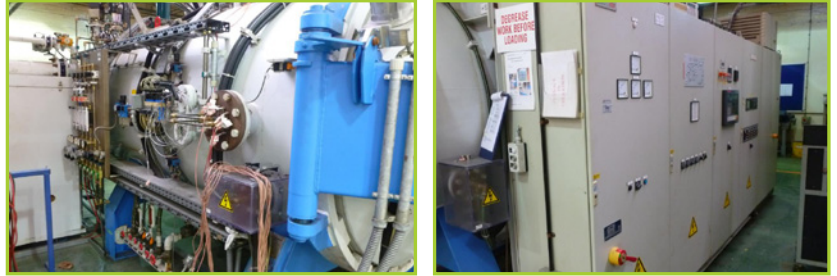
ALD VKNQ-PC60/60/90 VACUUM HARDENING FURNACE 5270 LITRE IN VESSEL, 515 LITRE IN DOUBLE JACKET, -1 BAR TO +20 BAR IN VESSEL, +1.5 BAR IN JACKET, NOMINAL TEMP 150DEGC, 1300DEGC MAX, CONTROL CABINETS & PANELS, CHART RECORDER, STANGE SE404 DIGITAL MONITORING PANEL
