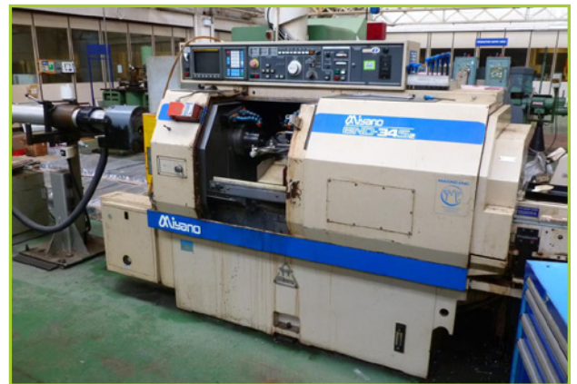
MIYANO BND 34S2 CNC LATHE FANUC SERIES O-T CONTROLS, 8 STATION TOOL CHANGER, LNS HYDROBAR TYPE 6.36 HS-4.8 5 METRE 6 SPINDLE AUTO BAR FEED. TWIN CHUCK, BACK WORKING CAPACITY, PARTS CATCHER & CONVEYOR, 34MM CAP
