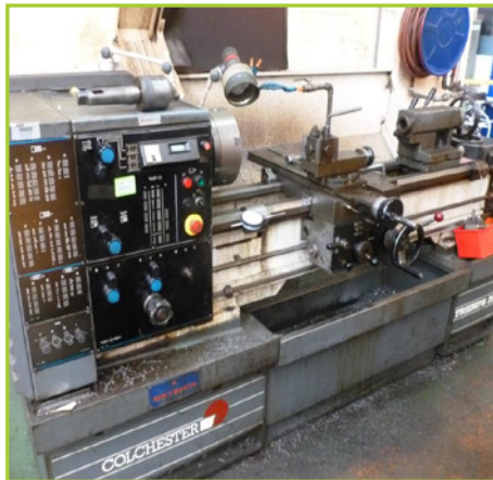
COLCHESTER TRIUMPH 2500 GAP BED CENTRE LATHE MAX 20" X 48" BC, 3 JAW CHUCK, CENTRE STEADY
