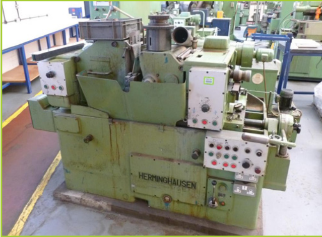
HERMINGHAUSEN SR3 CENTRELESS GRINDER COOLANT FILTRATION USED FOR GRINDING OUTSIDE DIAMETERS RANGING FROM 10MM -100MM DIAMETERS
