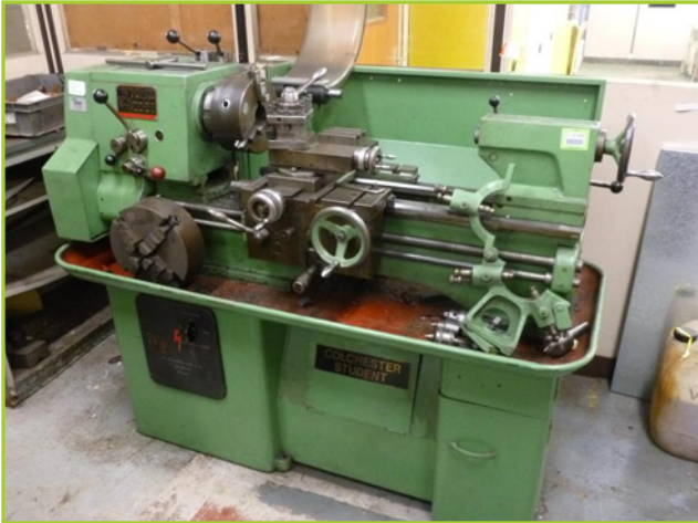
COLCHESTER STUDENT GAP BED CENTRE LATHE 13"OB X 24" BC, SS & SC, 8 SPINDLE SPEEDS, 54-1200RPM WITH 3 & 4 JAW CHUCKS & FIXED STEADY.
