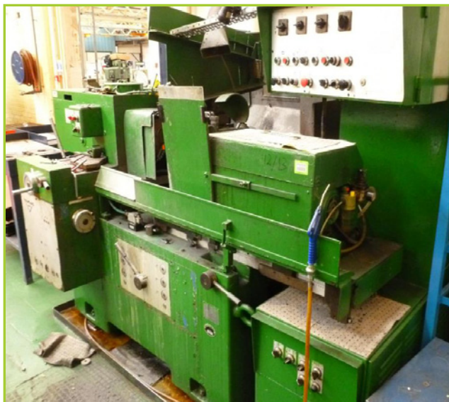
YOUMARD 52 ACE INTERNAL BORE GRINDER INTERNAL PARALLEL BORE GRINDER FOR DIAMETERS RANGING FROM 20MM - 150MM
