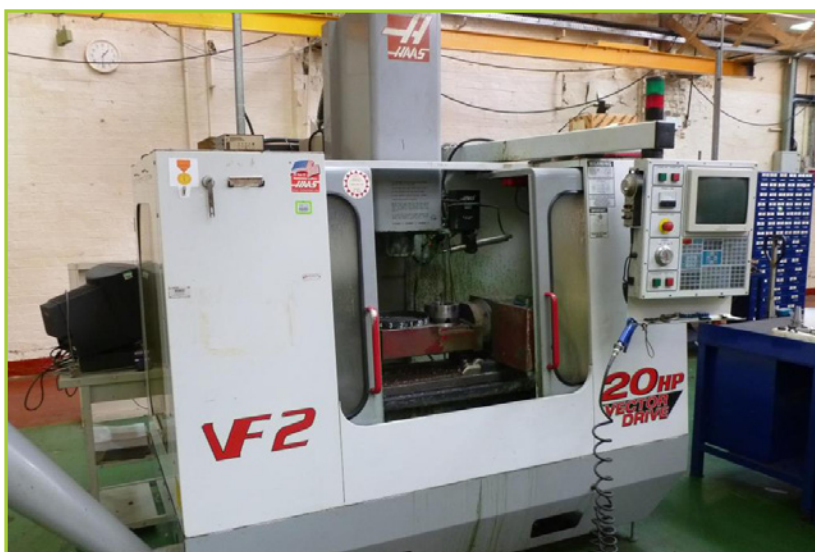
HAAS VF2 20 HP VECTOR DRIVE VERTICAL CNC MACHINING CENTRE 20 STATION TOOL CHANGER (4 FITTED), HAAS PROGRAMMABLE COOLANT NOZZLE, HAAS DIGITAL SERVO CONTROLS & OPERATORS PENDANT, 1999. INCLUDES 4TH AXIS & ADDITIONAL 5TH AXIS WITH HAAS CONTROL, TOOL WEAR GAUGE, RENISHAW M112 MACHINE INTERFACE
