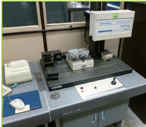
TAYLOR HOBSON SERIES 2 LASER FORM & SURFACE MEASURING MACHINE JOYSTICK CONTROL, GRANITE T SLOTTED TABLE
