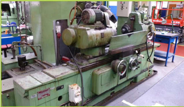
JOHANSSON 2U-D EXTERNAL CYLINDRICAL GRINDER FILTER MIST UNIT, USED FOR DIAMETERS RANGING FROM 100MM - 450MM
