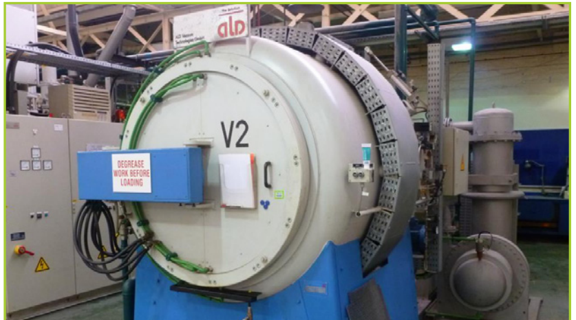
ALD VKNQ-PC60/60/90 VACUUM HARDENING FURNACE 5270 LITRE IN VESSEL, 515 LITRE IN DOUBLE JACKET, -1 BAR TO +20 BAR IN VESSEL, +1.5 BAR IN JACKET, NOMINAL TEMP 150DEGC, 1300DEGC MAX, CONTROL CABINETS & PANELS, CHART RECORDER, STANGE SE404 DIGITAL MONITORING PANEL
