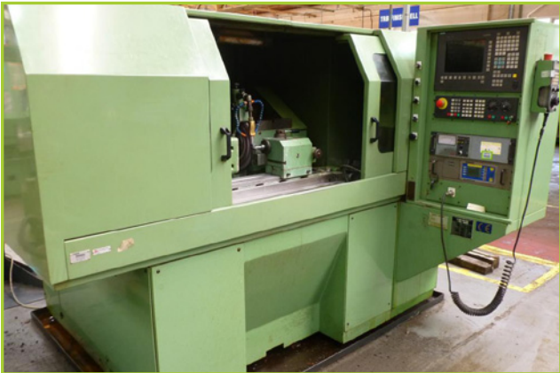
TSCHUDIN HTG 12 E14 400 CNC GRINDER TYPE 341 , 1997 REBUILT 2002. SIEMENS SINUMERIK SB5 BALANCE, FILTRATION/SWARF MANAGEMENT, MULTIFUNCTIONAL EXTERNAL CNC GRINDER FOR DIAMETERS RANGING FROM 10MM -150MM
