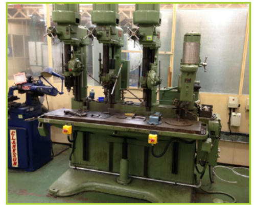
HERBERT PILLAR DRILL TAPPING MACHINE 3 GANG PILLAR DRILL & NO2 FLASH TAPPER
