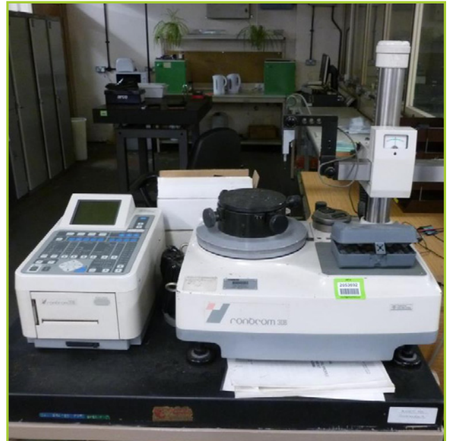
TOKYO SEIMITSU RONCOM 30B ROUNDNESS & CYLINDRICAL PROFILE TEST INSTRUMENT WITH MODEL E-MD-R134A DIGITAL CONTROL UNIT
