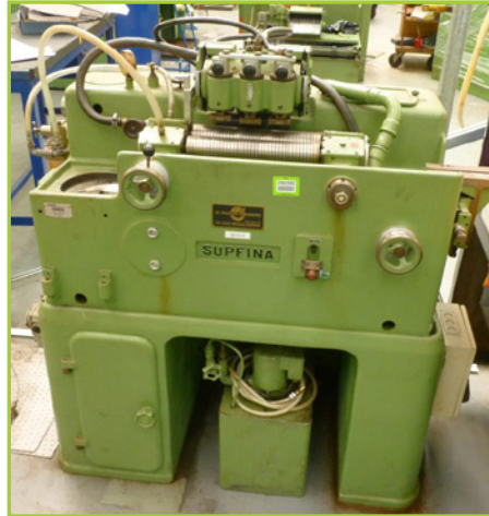
SUPFINA SM53 SUPER FINISHER/PARALLEL HONER USED WITH OSCILLATING HONING STONES.
