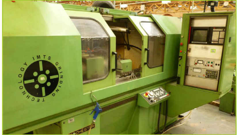
TSCHUDIN HTG 650 CNC EXTERNAL GRINDER NUM CONTROLS, MULTIFUNCTIONAL EXTERNAL CNC GRINDER FOR DIAMETERS RANGING FROM 10MM - 150MM
