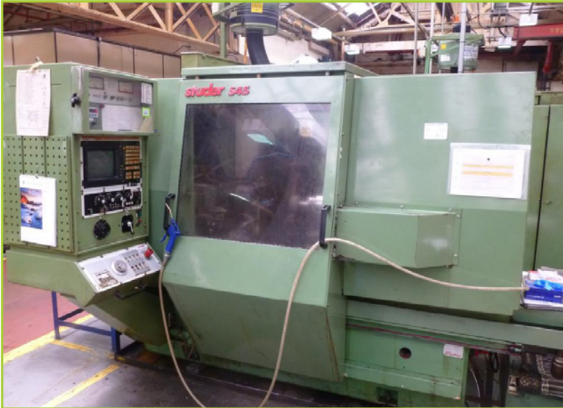
STUDER S45-6 CNC GRINDER SINUMERIK SYSTEM 3 CONTROLS, SWARF CONVEYOR, EXTERNAL & INTERNAL MULTIFUNCTION CNC GRINDER FOR PRODUCT RANGING FROM 50MM - 250MM OUTSIDE DIAMETERS
