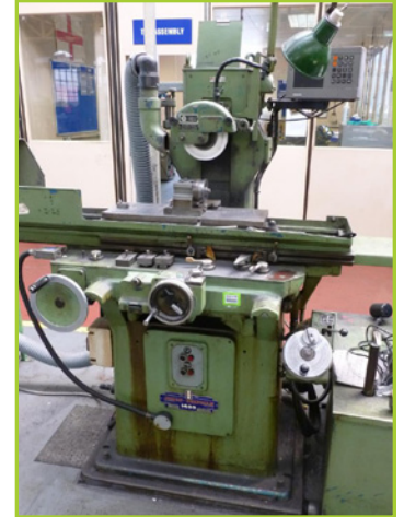
JONES & SHIPMAN 1400 SURFACE GRINDER 24" X 8" CAP, MAG CHUCK, HEIDENHAIN XY DRO
