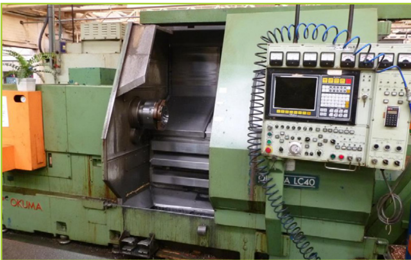
OKUMA LC40 2ST CNC TURNING CENTRE/LATHE 23.62" MAX SWING OB, 21.65" MAX TD, 28.74" MAX TL, OKUMACONTROLS & PENDANT, SWARF CONVEYOR, 12 STATION TC, STATION TC, TWIN TURRET
