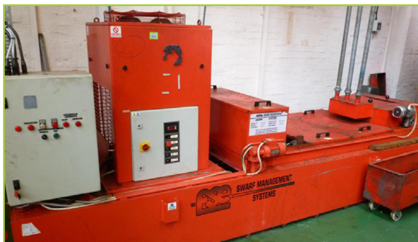
FSE CHIP/COOLANT MANAGEMENT SYSTEM 2200 LITRE CAP, 300LPM
