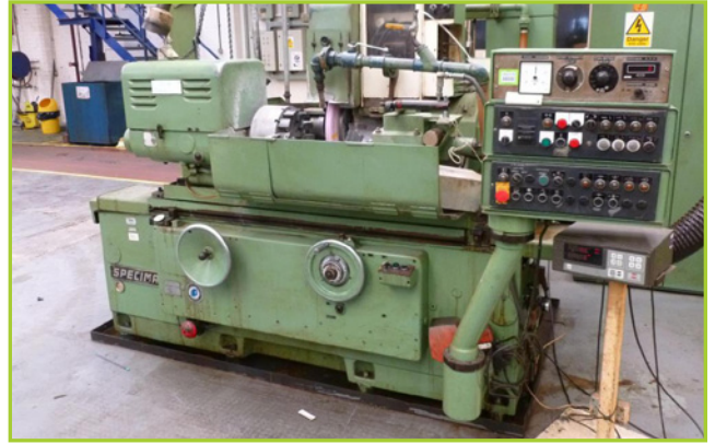
SPECIMA EXTERNAL CYLINDRICAL BALL RACE GRINDER SBS CONTROLLER, 2500 BALANCE SYSTEM & DRO, FILTERMIST & COOLANT FILTRATION, INNER RING FOR GRINDING RADIUS OF 5-50MM AND DIAMETERS OF 70MM-450MM
