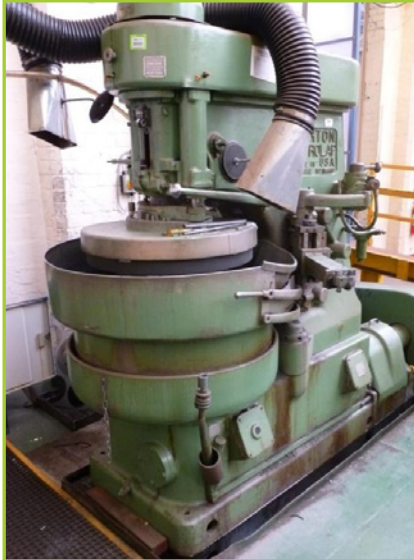
NORTON HYDROLAP FACE LAPPING MACHINE 700MM, FOR PRODUCT WITH DIAMETERS OF 15MM - 200MM
