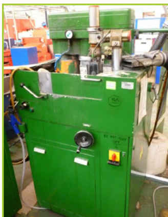
GMN MPS2 R300 ROTARY SURFACE GRINDER ROTARY SURFACE GRINDER FOR GRINDING SIDE FACES
