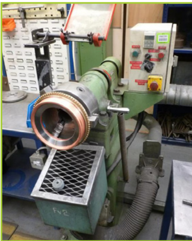
SINGLE HEAD POLISHING MACHINE WITH EXTRACTION DUCTING
