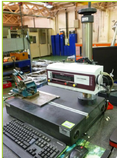
MITUTOYO CONTRACER CV-2000 SURFACE CONTOUR MEASURING SYSTEM WITH SINE VICE & PC
