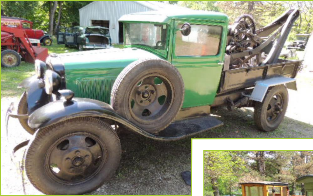
1930 MODEL A FORD WRECKER HAND CRANK, MFG. SASGEN DERRICK CO. CHICAGO, 4 SPEED TRANSMISSION W/ PTO
