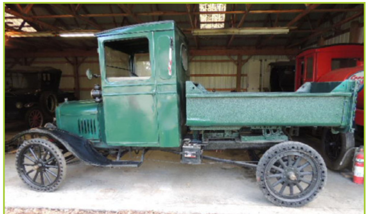
DUMP TRUCK, VIN 15000692, ENGINE RUNS GOOD, RUNS ON MAG. NEW BATTERY, SOLID TIRES, VAPORIZER NEEDS WORK, HAND CRANKED DUMP BODY
