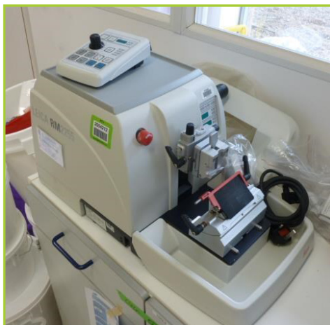
LEICA RM2255 AUTOMATED ROTARY MICROTOME JOYSTICK CONTROL, DRO & ACCESSORIES
