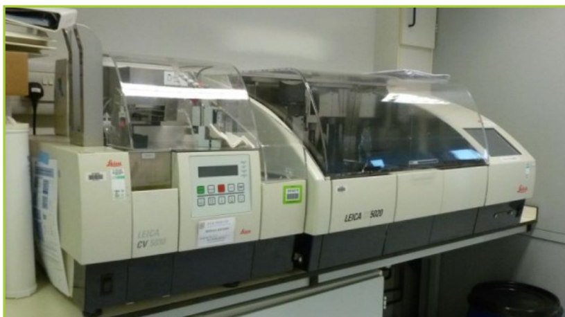
LEICA ST5020 WITH CV5030 ROBOTIC COVER SLIPPER SLIDE STAINING SYSTEM
