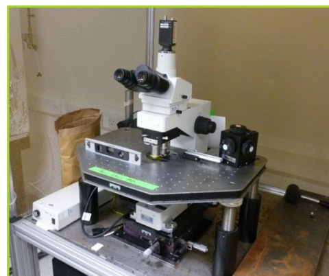
NIKON F600FN TRINOCULAR SCOPE, SER NO. 831261, 2 X LENS, DAGE MTI CAMERA, GIBRALTAR BURLEIGH BASE & SLICE PLATFORM
