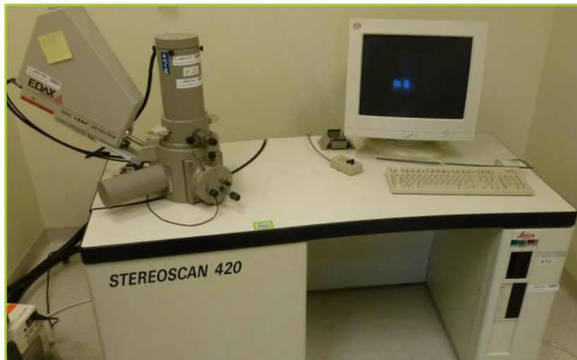
LEICA 420 WITH EDAX CDU LEAP DETECTOR & EMAX DX-4 DATA RECORDER ON WORKSTATION WITH REMOTE
