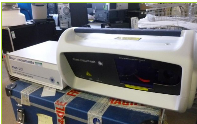
MOORLDI 5552 LARGE AREA DOPPLER IMAGING BLOOD FLOW LASER SYSTEM, HIGH RESOLUTION LASER UNIT
