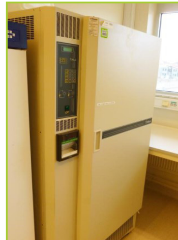
TERMA KBP6395F CLIMATOC CHAMBER, DRO & CHART RECORDER, PROGRAMMABLE LCD UNIT
