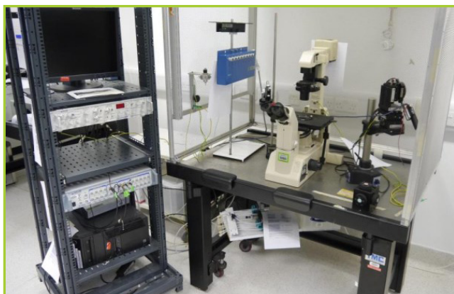
NIKON DIAPHOT 200 3 LENS, SCIENTIFICA ARTICULATED ROBOTIC MANIPULATOR, CONTROL PENDANT, INTRACELL EVH-9 MONITOR & CONTROL, AXON AXOPATCH CLAMP 200B
