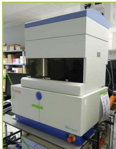
THERMO SCIENTIFIC HIGH CONTENT ANALYSIS SCREENING SYSTEM CELLOMICS VTI HCS LIQUID HANDLING
