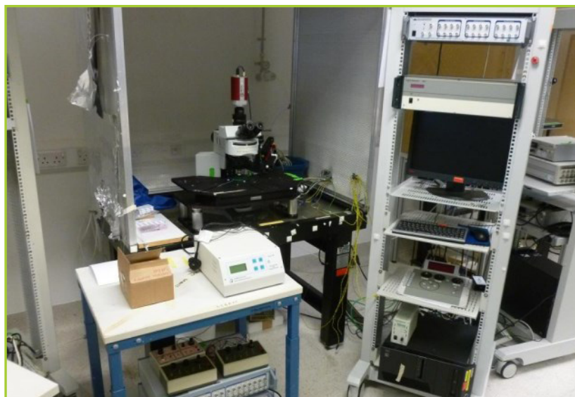
OLYMPUS BX51WI OPTICAL SCOPE, SER NO. 8M7125, IMAGING FITTED CAMERA, SCIENTIFICA SLICE PLATFORM WITH ROBOTIC MANIPULATOR, CAMPDEN INSTRUMENTS 7800 VISUAL PATCHING & IMAGING CHAMBER, AXON 700A MULTI CLAMP, AXON CNC DIGI DATA 1440A LOW NOISE DATA ACQUISITION UNIT, 2 X DIGITIMER DS2 ISOLATING STIMULATORS, 1 X DS3 ISOLATING STIMULATOR, 1 X PENDANT CONTROL, OLYMPUS TH4-200 CAMERA LIGHT CONTROL
