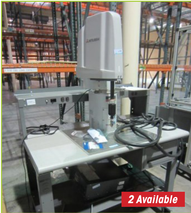
MITSUBISHI RH-6FH3520-D1 , WITH MITSUBISHI CR750 D CONTROLLER, MACHINE CLASS STANDARD, PROTECTION DEGREE IP 20, STRUCTURE - HORIZONTAL MULTIPLE-JOINT TYPE, 4 AXIS, DRIVE SYSTEM AC SERVO, MAX LOAD CAPACITY 6 KG, REACH ARM LENGTH (NO 1-125MM NO 2- 225 MM) MAX REACH 350MM, OPERATING RANGE AXIS 1 - 340 DEG, AXIS 2 - 290 DEG, AXIS 3 - 340 MM, AXIS 4 - 720 DEG, AXIS SPEED AXIS 1 - 400 DEG/SEC, AXIS 2 - 670 DEG/ SEC, AXIS 3 - 2400 MM/SEC, AXIS 4 - 2500 DEG/SEC, MAX COMPOSITE SPEED 6900 DEG/SEC POSITION REPEATABILITY X-Y +/- 0.10MM. INCLUDES STAND
