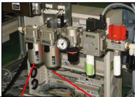
Air Filter (Dust & liquid is collected)
