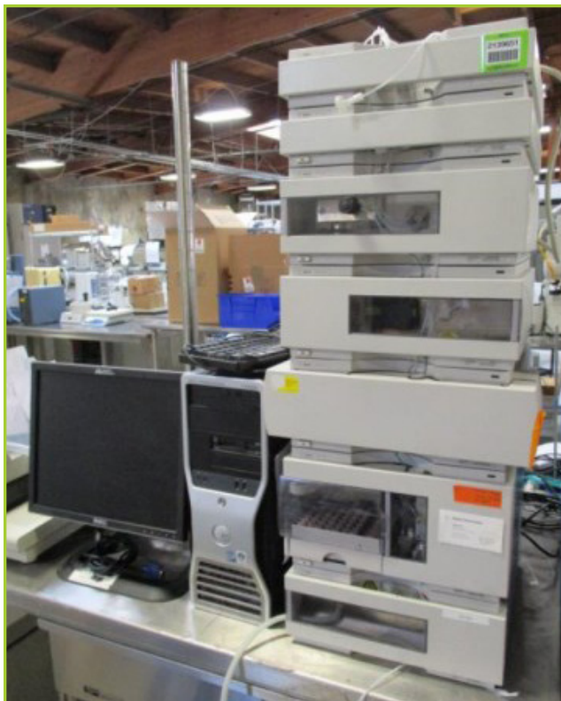
HPLC SYSTEM (6 MODULES): AGILENT 1100-SERIES (6-MODULES-TOTAL) HPLC SYSTEM. [WITH MODULES: AGILENT 1100/G1365B MULTIPLE WAVELENGTH DETECTOR S/N-DE33202334 ; AGILENT 1100/G1311A QUATPUMP S/N-DE33224159 ; AGILENT 1100/G1329A AUTOSAMPLER DE33211350 ; AGILENT 1100/G1330B AUTOSAMPLER THERMOSTAT S/N-DE33211350 ; AGILENT 1100/G1316A COLCOM S/N-DE33235139 ; AGILENT 1100/G1379A DEGASSER S/N-JP13210661. ALSO AGILENT 1100-SERIES REAGENT TRAY] [WITH DELL PRECISION-T3400 COMPUTER, 17" MONITOR AND KEYBOARD]
