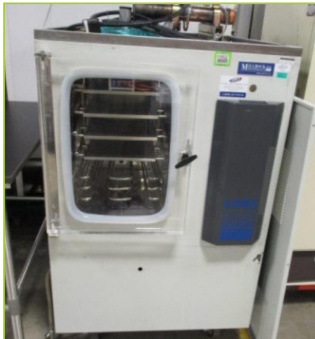
MILLROCK TECH LD85-B3 LYOPHILIZER S/N-LD850906007B3. WITH LEYBOLD TRIVAC #D8B VACUUM PUMP
