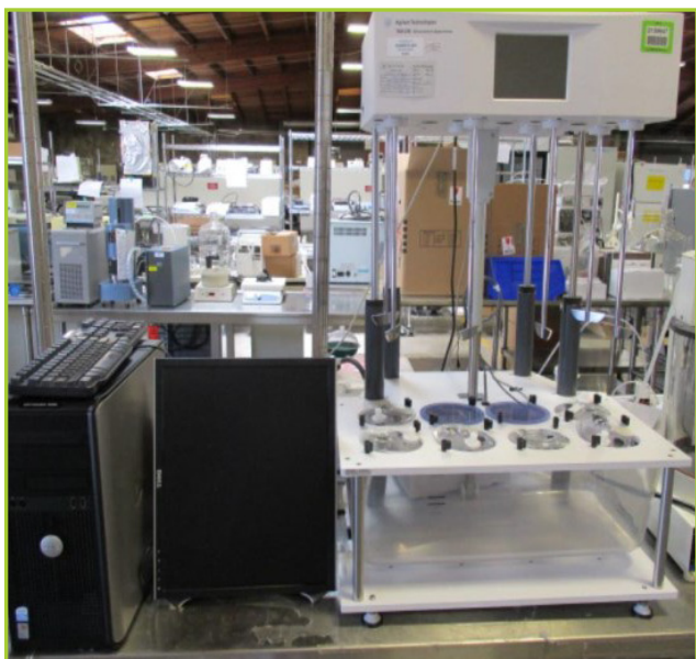
AGILENT 708-DS DISSOLUTION APPARATUS (AGILENT MODEL#G7910A P/N-G7910-60423 ; S/N-MY15278304) (8-POSITION CONFIGURATION/BUT 6-POSITION TESTING ; 1L, MOTORIZED LIFT) (WITH AGILENT #G7986A PUMP). WITH DELL OPTIPLEX-330 COMPUTER, 19" MONITOR AND KEYBOARD
