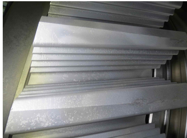
Fig. 21. Row 4 Wheel dovetail - Pitting
