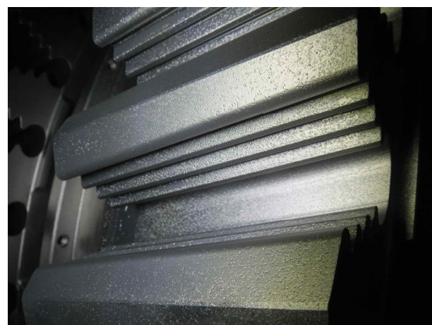
Fig. 14. Row 2 Wheel dovetail - Pitting
