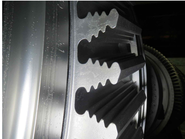
Fig. 10. Row 1 Wheel dovetail - Pitting
