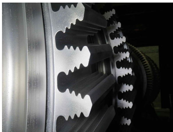
Fig. 13. Row 2 Wheel dovetail - Pitting
