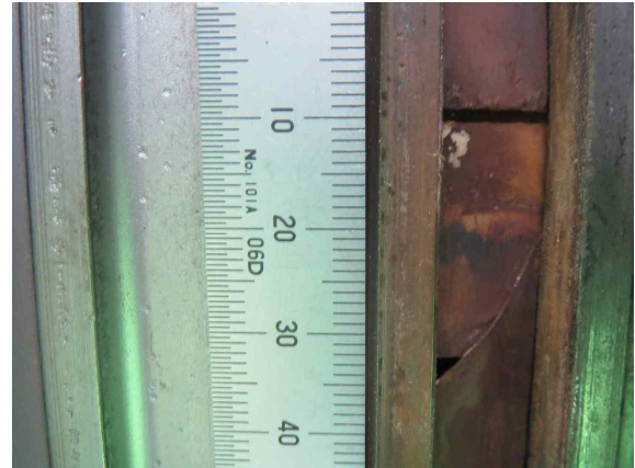
Figure 7. Row 1-2 Belly Band Fracture
