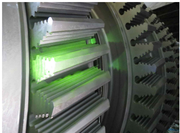
Fig. 9. Row 4 Wheel dovetail MPI
