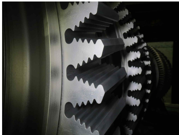
Fig. 16. Row 3 Wheel dovetail - Pitting
