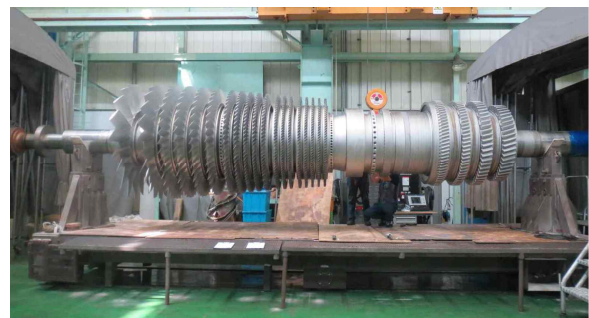
Figure 3. Unit Rotor Blast Cleaning status
