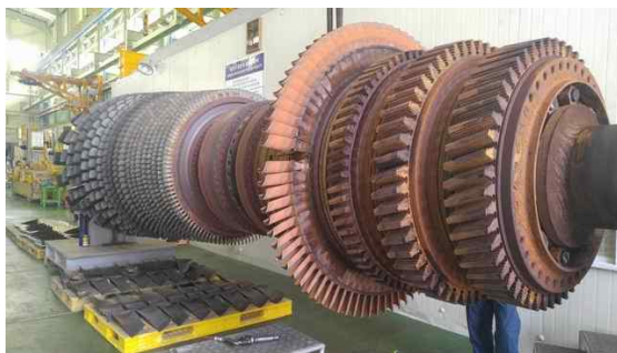
Figure 2. Turbine Blades Withdrawal
