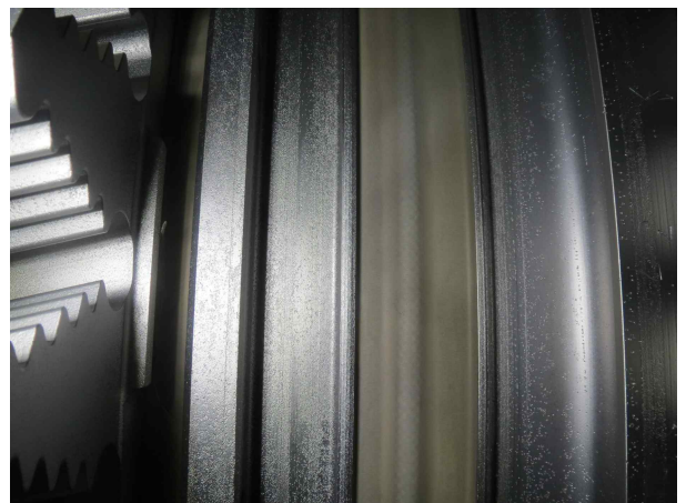
Fig. 18. Row 3 Wheel dovetail - Pitting
