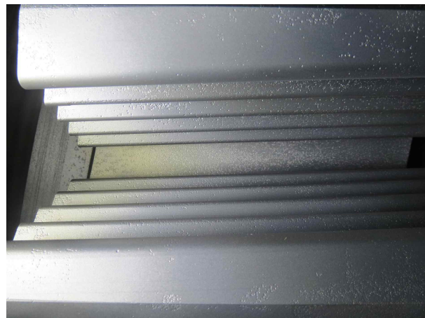
Fig. 17. Row 3 Wheel dovetail - Pitting
