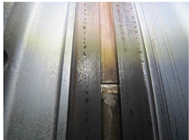
Fig. 24. Row 3 Bally bend - No linear indication
