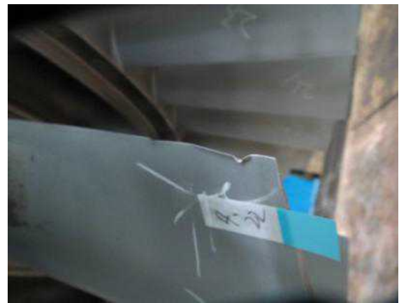
Figure 9. Compressor Blade Dent
