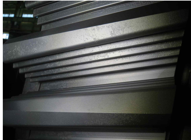
Fig. 20. Row 4 Wheel dovetail - Pitting
