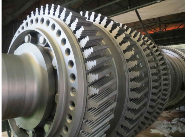
Fig. 19. Row 4 Wheel dovetail - Pitting
