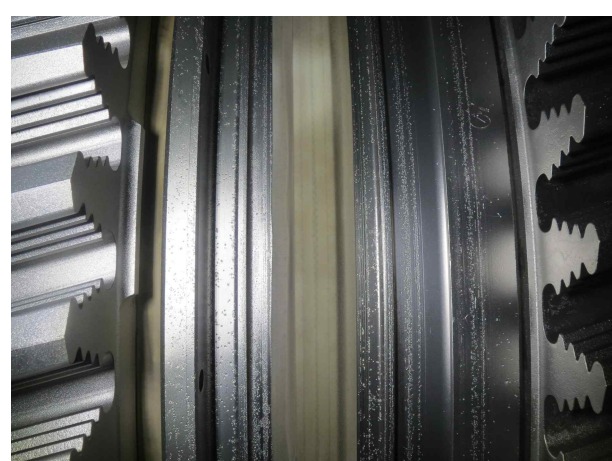
Fig. 15. Row 2 Wheel dovetail - Pitting
