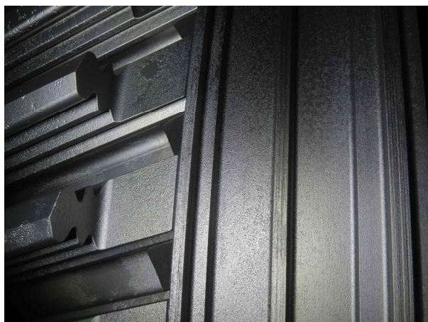
Fig. 12. Row 1 Wheel dovetail - Pitting
