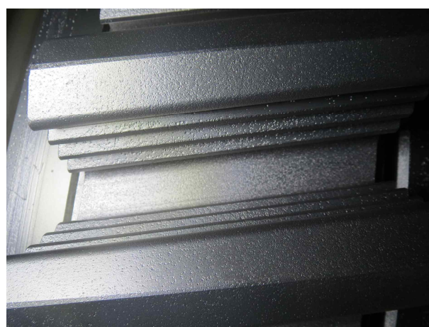
Fig. 14. Row 2 Wheel dovetail - Pitting
