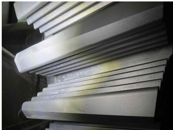
Fig. 20. Row 4 Wheel dovetail - Pitting
