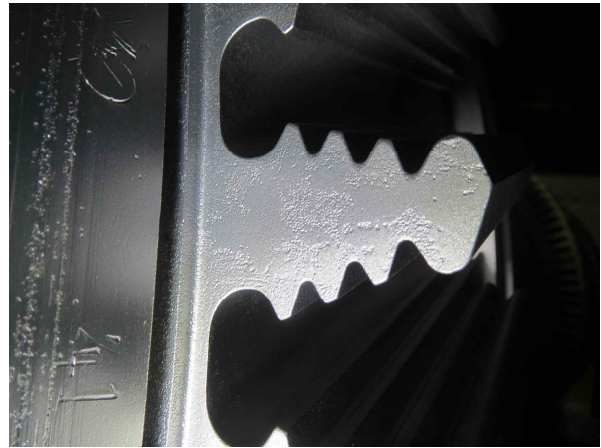
Fig. 10. Row 1 Wheel dovetail - Pitting
