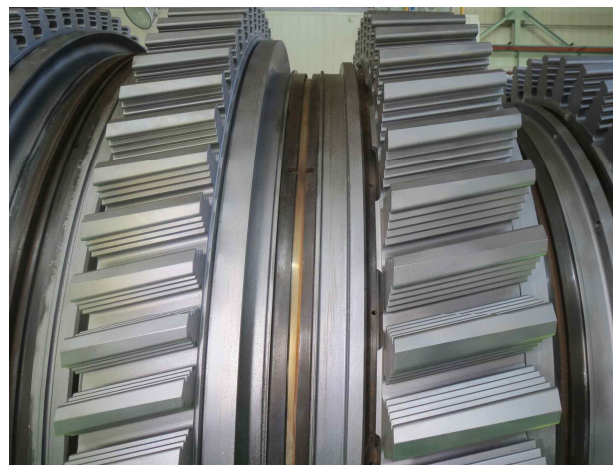
Fig. 23. Row 2 Bally bend - No linear indication
