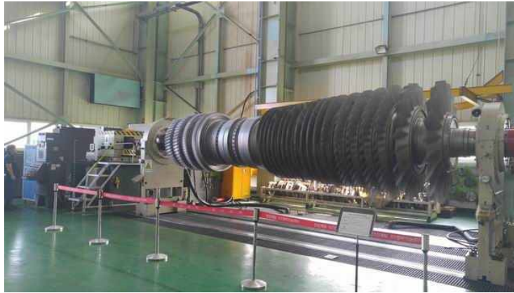
Figure 13. Unit Rotor Shop Balancing
