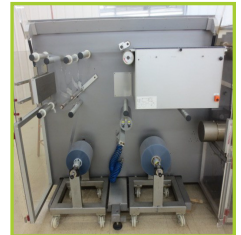
KLOCKNER CP-1200, P-3000 BLISTER MACHINE AND CARTONER PACKAGING LINE . CAPABLE OF THERMOFORMING, COLDFORMING AND CARTONING AT SPEEDS UP TO 400 BLISTER PACKS/MIN AND 300 CARTONS/MIN. WITH HASKRIS CHILLER, GREYDON MDL. 01SBM053 PRINTER S/N 325BPP. WITH MANUALS. WITH 3 CRATES OF ADDITIONAL RAILS.
