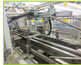
SCHROEDER MACHINES 2600 CASE PACKER , THIS MACHINE WILL PACK UP TO 12 CASES PER MINUTE AND IS ADJUSTABLE TO ACCOMMODATE A RANGE OF CASE AND PRODUCT SIZES. WITH NORDSON GLUE PUMP. SN# 5599
