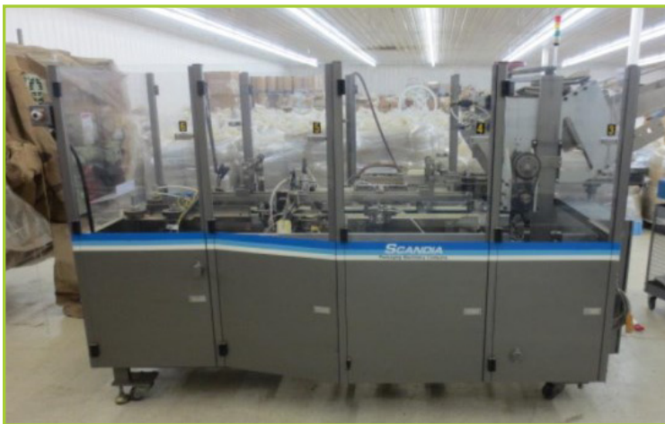
SCANDIA PACKAGING MACHINE CO. ALIM CARTONER, QUICK PANEL JR. CONTROL. PLUS 500 SRS PROGRAMMABLE LIMIT SWITCH ELECTRO CAM. 4" CONVEYOR. 460V. SN# 4558.
