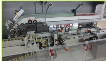
KLOCKNER CP-1200, P-3000 BLISTER MACHINE AND CARTONER PACKAGING LINE . CAPABLE OF THERMOFORMING, COLDFORMING AND CARTONING AT SPEEDS UP TO 400 BLISTER PACKS/MIN AND 300 CARTONS/MIN. WITH HASKRIS CHILLER, GREYDON MDL. 01SBM053 PRINTER S/N 325BPP. WITH MANUALS. WITH 3 CRATES OF ADDITIONAL RAILS.
