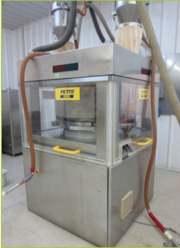
FETTE 3200 TABLET PRESS , COMPUTER CONTROLLED, HIGH-PERFORMANCE, DOUBLE-SIDED ROTARY TABLET PRESS WITH INTERCHANGEABLE DIE TABLE. WITH 2- FETTE GRATEX FEEDERS, 1- ELECTRICAL PANEL, 1- CONTROL STATION, VACUMAX CONVEYING SYSTEM. WITH MANUALS, DIE KIT, AND TOOL BOX. SN# 659
