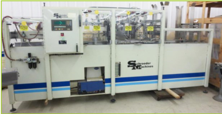
SCHROEDER MACHINES 2600 CASE PACKER , THIS MACHINE WILL PACK UP TO 12 CASES PER MINUTE AND IS ADJUSTABLE TO ACCOMMODATE A RANGE OF CASE AND PRODUCT SIZES. WITH NORDSON GLUE PUMP. SN# 5599
