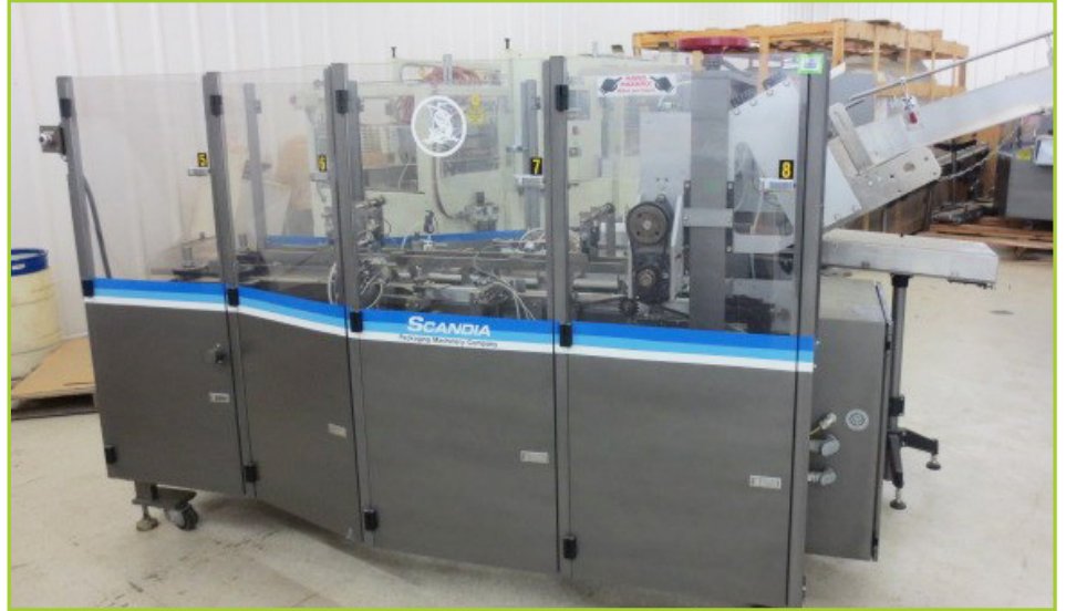
SCANDIA PACKAGING MACHINE CO. ALIM CARTONER, QUICK PANEL JR. CONTROL. PLUS 500 SRS PROGRAMMABLE LIMIT SWITCH ELECTRO CAM. 4" CONVEYOR. 440V. SN# 4566
