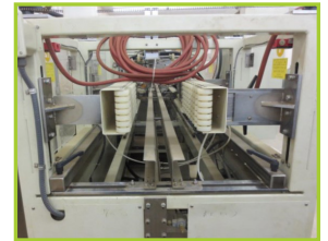
SCHROEDER MACHINES 2600 CASE PACKER , THIS MACHINE WILL PACK UP TO 12 CASES PER MINUTE AND IS ADJUSTABLE TO ACCOMMODATE A RANGE OF CASE AND PRODUCT SIZES. WITH NORDSON GLUE PUMP. SN# 5599
