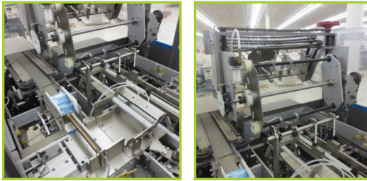
SCANDIA PACKAGING MACHINE CO. ALIM CARTONER, QUICK PANEL JR. CONTROL. PLUS 500 SRS PROGRAMMABLE LIMIT SWITCH ELECTRO CAM. 4" CONVEYOR. 440V. SN# 4566
