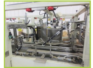
SCANDIA PACKAGING MACHINE CO. ALIM CARTONER, QUICK PANEL JR. CONTROL. PLUS 500 SRS PROGRAMMABLE LIMIT SWITCH ELECTRO CAM. 4" CONVEYOR. 440V. SN# 4566
