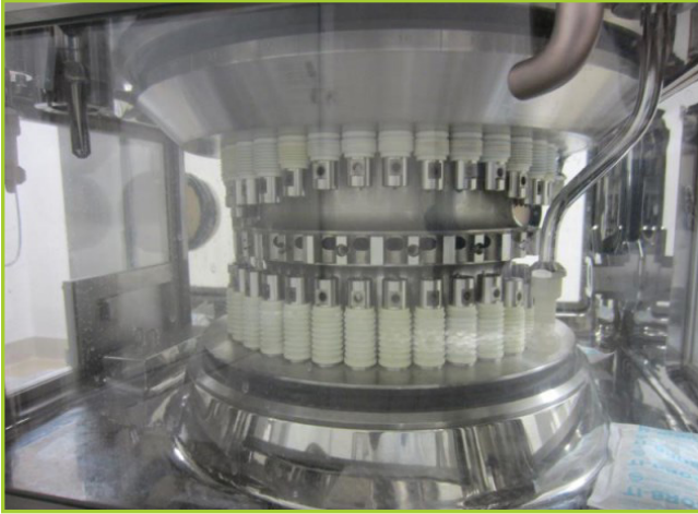
IMA COMPRIMA 300 TABLET PRESS. 36 STATION TURRET, 5 MM - 16 MM ROUND MAX TABLET DIAMETER, 5 MM - 17 MM OBLONG TABLET SIZE, TURRET MOUNTED IN GLOVE BOX ISOLATOR WITH TOTE TABLET PRESS MAIN DISCHARGE ISOLATOR ALL STAINLESS STEEL 316L & 304 CONSTRUCTION WITH KRAMER C810 CONTROLLER TYPE E2100-1250 DEDUSTER CH-8303, SAFELINE METAL DETECTION, CONTROL PANELS TRANSFORMER, FRISTAM PUMP. (1) SKID VARIOUS SS CHUTES, GUIDES, (1) ERWEKA TABCHECK 3 WITH METTLER TOLEDO AB54 BALANCE IN A TOTE 2 GLOVE BOX ENCLOSURE. SN# 85048
