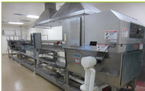
SANDVIK ROTOFORM 3000 BELT WIDTH 32", BELT SPEED 20- 120 FPM, COOLER LENGTH 33' 9", COOLING SECTION LENGTH 24', ALLEN BRADLEY PANELVIEW, ELECTRICAL PANEL WITH PLC, HONEYWELL DIGITAL READOUTS, ALLEN BRADLEY PROGRAMMABLE TERMINALS, (2) KEES INC. STAINLESS STEEL HOODS & (1) SS CABINET WITH SPARE PARTS
