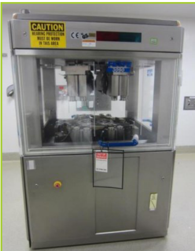
FETTE P3090 IC TABLET PRESS. 49 STATION ROTARY TABLET PRESS , TURRET IN STORAGE STAND WITH ELECTRICAL PANEL MAIN CONTROL PANEL. ALL CABLES, RATED UP TO 700,000 TABLETS PER HR, METRO RACK WITH ASSORTED PARTS, YR 1999. SN# 29 264
