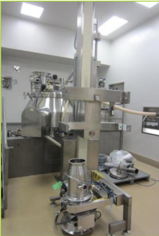
NIRO PMA 800 HIGH SHEAR GRANULATOR . STAINLESS STEEL CONSTRUCTION, 800 LITER DESIGN, JACKETED BOWL WITH 100 GAL. SOLUTION TANK, EASTON MIXER MODEL FRG-5CM, ACTUATOR, WITH SERVO O LIFT BIN LIFT FOR A 38" BIN, BIN ACTUATOR VALVES, CHUTES, 1 SKID ASSORTED SEALS, STAINLESS STEEL CHUTES. S/N 99160.0001
