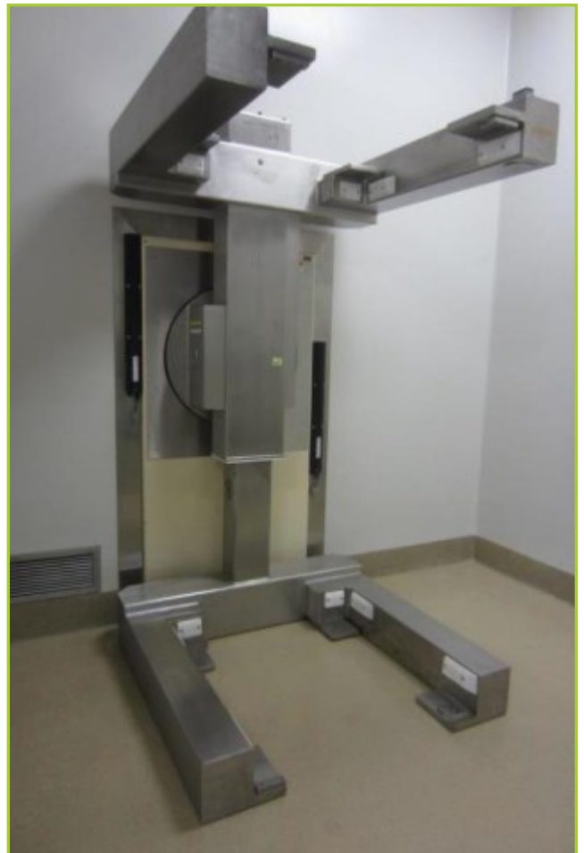
SERVO LIFT BIN BLENDER. 1250KG / 2750LB CAPACITY, 1336 DRIVE, AB PLC, AB 1305 DRIVE, FOR APPROX. 38" X 66" BIN WITH SAFETY LIGHT CURTAINS. S/N 10079
