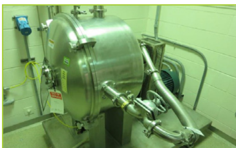
CORNELL MACHINE COMPANY D-26LH VERSATOR , 25HP MOTOR. S/N-1943
