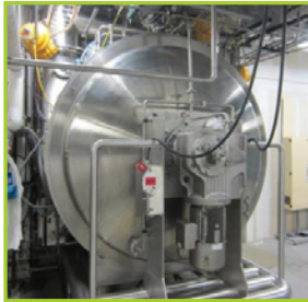
THOMAS ENGINEERING COATING PAN. SPECTRUM COATER FOR CONTAINMENT, PACE SIZE PF-18 AF SWSI AIR HANDLER, ALLEN BRADLEY 1336 PLUS DRIVES, (2) STAINLESS STEEL PRESSURE VESSELS WITH CLEVELAND EASTON MIXER MODEL FRG3M AND (1) SKID ASSORTED PARTS.
