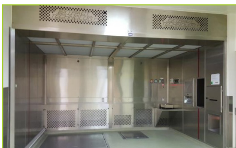
EXTRACTTECHNOLOGY DX/6R/8/126 DOWN FLOW BOOTH . 12 FILTERS, CONTROLS. GLEASON HOSE REEL UH28MTR-24-1610, ROSEMOUNT SENSORS, BOOTH INSIDE DIMENSIONS 9'D X 13'W X 95"H. 460V 3PH
