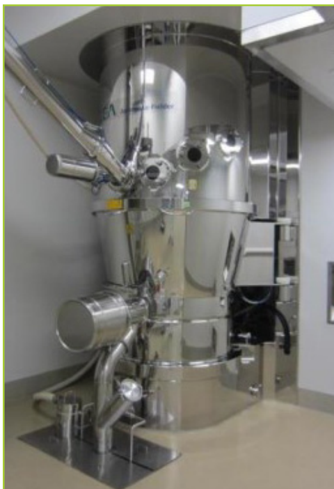
GEA NIRO AEROMATIC FIELDER P7-F1 FLUID BED DRYER / GRANULATOR . 10 BAR MACHINE, RATED FOR SOLVENTS. BOWL SIZE J7 WITH PACE AIR HANDLER, CARGOCAIRE HONEYCOMB DEHUMIDIFIER, ALLEN BRADLEY CONTROLS AND SERVO LIFT. BIN LIFT 2750LB CAPACITY. ALSO INCLUDES (1) METRO CART WITH ASSORTED PARTS & 2 SPARE SPRAY NOZZLES
