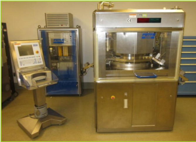
WILHELM FETTE GMBH 3090 DOUBLE SIDETABLET PRESS, (2001) , 50-STATION TURRET ASSEMBLY CURRENTLY INSTALLED, MAX. PRESSURE FORCE: 100 (120) KN, MAX. PREPRESSURE FORCE 100 (120) KN, PITCH CIRCLE DIAMETER: 680 MM, TOP PUNCH INSERTION DEPTH: 2-4 (8/12) MM, INCLUDES INCHING BOX, FREE STANDING OPERATOR CONSOLE & CONTROL CABINET, POWER CONSUMPTION 16/21 KW, 400VAC, 50/60HZ, 3PH
