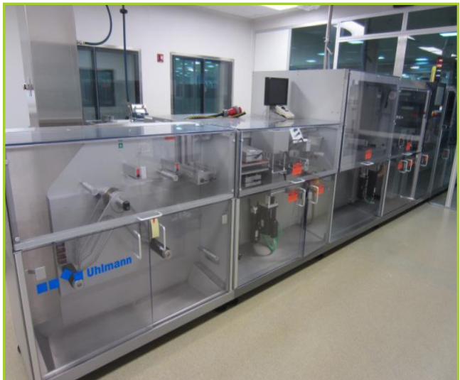
UHLMANN TYPE BEC 105 BLISTER PACK EXPRESS. WITH SIMTAP 600S3 DISCHARGE FEEDER, UHLMANN VISIOPRINT SN# 057105-1, UHLMANN VISIOMARK, BLISTER PAK DETECTOR, MODEL 2065 CARTONER, YR 2001, WITH (3) TOOLING CARTS CONSISTING OF PUNCHING TOOL, SINGLE STROKE INDEX, UPPER SEALING TOOL, LOWER SEALING TOOL, FORMING TOOL, DECURLER, LOWER COOLING PLATE, GUIDE PLATES, SINGLE STROKE INDEX, LOWERATOR, 55" DIA TURN TABLE, CABINET WITH PARTS FOR CARTONER, THERMO NESLAB MODEL HX150 RECIRCULATING CHILLER, (2) LOADING CARTS & (1) INDUSTRIAL CABINET WITH CHANGE OVER PARTS. ALSO, INCLUDES VISON SYSTEM, CSTAT PRINTER AND LEAFLET INSERTER
