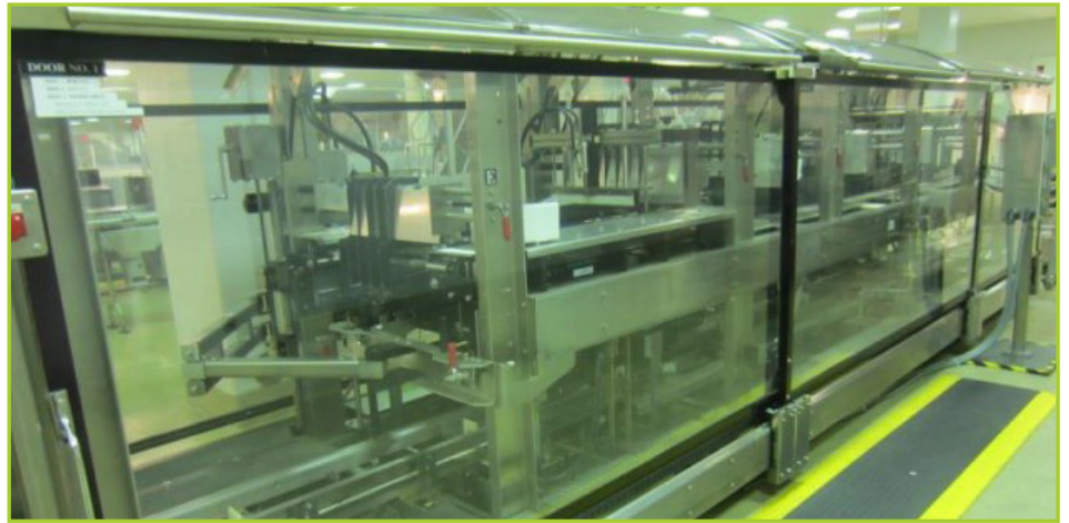
HARTNESS INTERNATIONAL CASE PACKER. AUTOMATED CASE PACKER , HARDNESS INTERNATIONAL READOUT, XYCOM TOUCH SCREEN, 16" MAX BOX WIDTH, CAN FEED 4 BOTTLES. 16" X 9" BOX ENTRY CONVEYOR, 6" X 77" ENTRY BOTTLE CONVEYOR. DORNER 3 3/4" X 32" SAMPLE CONVEYOR. SN# 28-095
