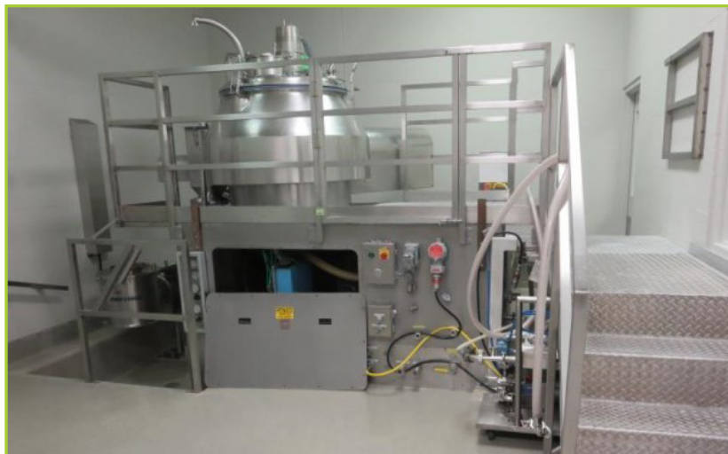
NIRO PMA 800 HIGH SHEAR GRANULATOR STAINLESS STEEL CONSTRUCTION, 800 LITER DESIGN, JACKETED BOWL, QUADRO COMIL U30, G & H SANITARY ROTARY PUMP MODEL GHP-601, ALLEN BRADLEY PANEL VIEW 1200 & REDI PANEL, INGERSOLL-RAND 550LB CAPACITY AIR HOIST, ALUMINUM PLATFORM, (3) CARTS WITH ASSORTED SS CHUTES, & HOSES, (1) CART WITH BRANSON 8200 ULTRA SONIC CLEANER & DRYER, (1) 4 DRAWER STANLEY VIDMAR CABINET WITH ASSORTED HOSES & CLAMPS
