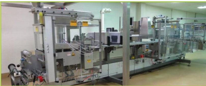
UHLMANN UPS4 THERMOFORMER BLISTER PACK SYSTEM, AYLWARD ENTERPRISE TABLET FEEDER MODEL XYZ S/N 2759, VISION SYSTEM VA 350-1 COLOR VISION, TISMA MACHINERY CORP MODEL TC -100 S/N 1351, ARGUS 4 BAR CODE SCANNER, RAMSEY ICORE AUTOCHECK 9000 PLUS CHECK WEIGHER, PNEUMATIC SCALE MODEL 2000-W CASE PACKER S/N 20001-1, LASERLINK CORP. Z CODE MANNING LASER SYSTEM MODEL Z-CODE SMARTLASE S/NA-5426, (3) CONVEYOR BELTS 10" WIDE, 11" WIDE & 12" WIDE & (1) RECEIVER TANK
