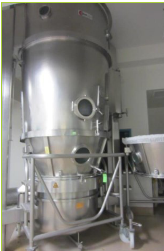
GLATT GPCG300 POWDER COATER GRANULATOR. GENTLE COATING WITH VERSATILITY, ALL STAINLESS STEEL CONSTRUCTION. RATED AT 3 BAR. CAPACITY: 300KG. CONSISTING OF (2) BOWLS, ALLEN BRADLEY PANEL VIEW 1200, POST HOIST LIFT & TILT, 1 SKID OF PARTS, PACE AIR HANDLER, CARGOCAIRE HONEYCOMBE DEHUMIDIFIER, PHELPS FAN VRH-261 X.8, & DURO FLOW ROTARY BLOWER
