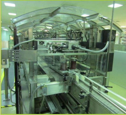
HARTNESS INTERNATIONAL CASE PACKER. AUTOMATED CASE PACKER , HARDNESS INTERNATIONAL READOUT, XYCOM TOUCH SCREEN, 16" MAX BOX WIDTH, CAN FEED 4 BOTTLES. 16" X 9" BOX ENTRY CONVEYOR, 6" X 77" ENTRY BOTTLE CONVEYOR. DORNER 3 3/4" X 32" SAMPLE CONVEYOR. SN# 28-095
