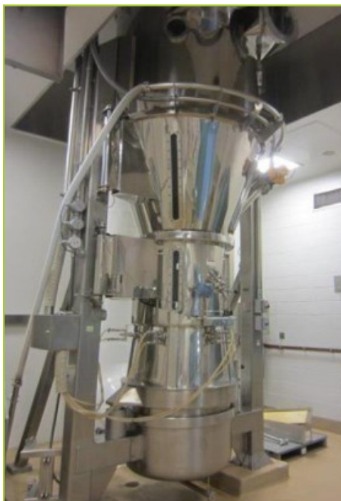
GLATT AIR TECHNOLOGIES GPCG120 FLUID BED GRANULATOR . COMPRESSED AIR PRESSURE BAR 6, STEAM PRESSURE 3U BAR, WURSTER COLUMNS (3) PERISTALTIC PUMPS WITH EASY LOAD, ROSE MOUNT PRESSURE & TEMPERATURE TRANSMITTERS, ALLEN BRADLEY PANEL VIEW PLUS 1500, CHILLER WATER & STEAM AIR HANDLER, YR 1985. SN# 4208
