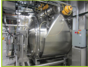
THOMAS ENGINEERING COATING PAN. SPECTRUM COATER FOR CONTAINMENT, PACE SIZE PF-18 AF SWSI AIR HANDLER, ALLEN BRADLEY 1336 PLUS DRIVES, (2) STAINLESS STEEL PRESSURE VESSELS WITH CLEVELAND EASTON MIXER MODEL FRG3M AND (1) SKID ASSORTED PARTS.
