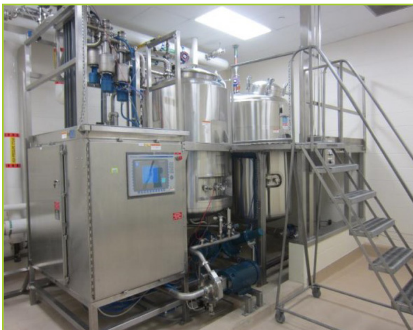
DOBER GROUP CIP SKID. (1) 500 GAL JACKETED VESSEL (TANK) MAEP 40PSI @ 300° F(1) 250 GAL JACKETED VESSELS, SS ALLEN BRADLEY PANEL VIEW PLUS 1500 TOUCH SCREEN, SS PUMP WITH 15HP MOTOR, (2) MTS SENSORS, (4) ROSEMOUNT SENSORS, (4) TUCHENHAGEN VALVES 10BAR MAX, (2) MICRO PUMPS, INCLUDES PLATFORM
