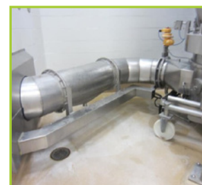
GLATT GPCG300 POWDER COATER GRANULATOR. GENTLE COATING WITH VERSATILITY, ALL STAINLESS STEEL CONSTRUCTION. RATED AT 3 BAR. CAPACITY: 300KG. CONSISTING OF (2) BOWLS, ALLEN BRADLEY PANEL VIEW 1200, POST HOIST LIFT & TILT, 1 SKID OF PARTS, PACE AIR HANDLER, CARGOCAIRE HONEYCOMBE DEHUMIDIFIER, PHELPS FAN VRH-261 X.8, & DURO FLOW ROTARY BLOWER
