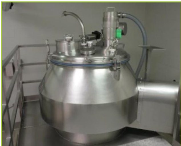
NIRO PMA 800 HIGH SHEAR GRANULATOR STAINLESS STEEL CONSTRUCTION, 800 LITER DESIGN, JACKETED BOWL, QUADRO COMIL U30, G & H SANITARY ROTARY PUMP MODEL GHP-601, ALLEN BRADLEY PANEL VIEW 1200 & REDI PANEL, INGERSOLL-RAND 550LB CAPACITY AIR HOIST, ALUMINUM PLATFORM, (3) CARTS WITH ASSORTED SS CHUTES, & HOSES, (1) CART WITH BRANSON 8200 ULTRA SONIC CLEANER & DRYER, (1) 4 DRAWER STANLEY VIDMAR CABINET WITH ASSORTED HOSES & CLAMPS
