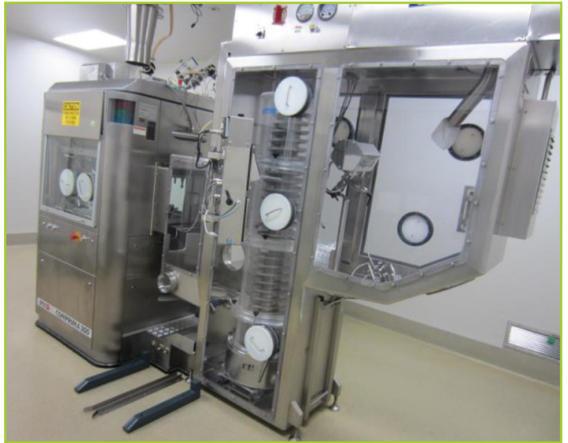
IMA COMPRIMA 300 TABLET PRESS. 36 STATION TURRET, 5 MM - 16 MM ROUND MAX TABLET DIAMETER, 5 MM - 17 MM OBLONG TABLET SIZE, TURRET MOUNTED IN GLOVE BOX ISOLATOR WITH TOTE TABLET PRESS MAIN DISCHARGE ISOLATOR ALL STAINLESS STEEL 316L & 304 CONSTRUCTION WITH KRAMER C810 CONTROLLER TYPE E2100-1250 DEDUSTER CH-8303, SAFELINE METAL DETECTION, CONTROL PANELS TRANSFORMER, FRISTAM PUMP. (1) SKID VARIOUS SS CHUTES, GUIDES, (1) ERWEKA TABCHECK 3 WITH METTLER TOLEDO AB54 BALANCE IN A TOTE 2 GLOVE BOX ENCLOSURE. SN# 85048
