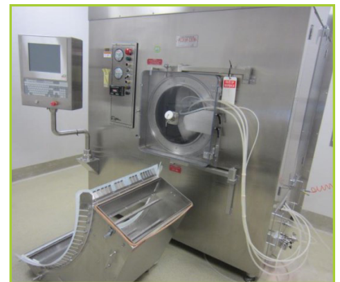
THOMAS ENGINEERING 60DXL TYPE SPECTRUM COATER , DEEP PERFORATED PAN, 6 SPRAY GUNS, 53"D X 60"DIA., PAN LOAD RATING 1000LBS, ALL STAINLESS STEEL CONSTRUCTION, ALLEN BRADLEY 1336 PLUS DRIVE, ROSEMOUNT SENSORS, ACCELA SCOOP. 54" PAN DEPTH
