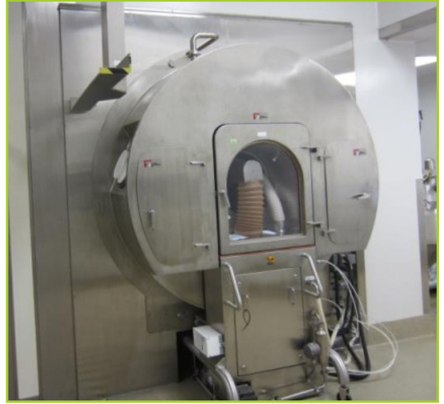
THOMAS ENGINEERING COATING PAN. SPECTRUM COATER FOR CONTAINMENT, PACE SIZE PF-18 AF SWSI AIR HANDLER, ALLEN BRADLEY 1336 PLUS DRIVES, (2) STAINLESS STEEL PRESSURE VESSELS WITH CLEVELAND EASTON MIXER MODEL FRG3M AND (1) SKID ASSORTED PARTS.
