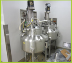
THOMAS ENGINEERING COATING PAN. SPECTRUM COATER FOR CONTAINMENT, PACE SIZE PF-18 AF SWSI AIR HANDLER, ALLEN BRADLEY 1336 PLUS DRIVES, (2) STAINLESS STEEL PRESSURE VESSELS WITH CLEVELAND EASTON MIXER MODEL FRG3M AND (1) SKID ASSORTED PARTS.
