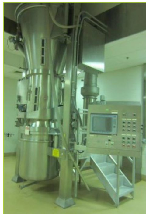
GLATT AIR TECHNOLOGIES GPCG120 FLUID BED GRANULATOR . COMPRESSED AIR PRESSURE BAR 6, STEAM PRESSURE 3U BAR, WURSTER COLUMNS (3) PERISTALTIC PUMPS WITH EASY LOAD, ROSE MOUNT PRESSURE & TEMPERATURE TRANSMITTERS, ALLEN BRADLEY PANEL VIEW PLUS 1500, CHILLER WATER & STEAM AIR HANDLER YR 1991. SN# 5244
