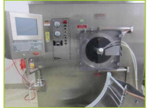
THOMAS ENGINEERING 60DXL TYPE SPECTRUM COATER , DEEP PERFORATED PAN, 6 SPRAY GUNS, 53"D X 60"DIA., PAN LOAD RATING 1000LBS, ALL STAINLESS STEEL CONSTRUCTION, ALLEN BRADLEY 1336 PLUS DRIVE, ROSEMOUNT SENSORS, ACCELA SCOOP. 54" PAN DEPTH
