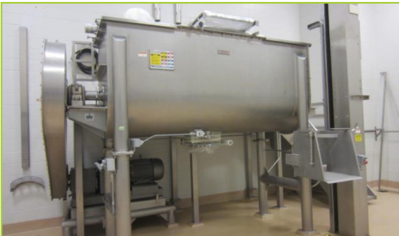
DAY MIXING HORIZONTAL RIBBON BLENDER. 120 CU. FT, 40HP MOTOR WITH MATERIALS TRANSPORTATION COMPANY H-LO-1 DRUM DUMPER, 800LB CAPACITY WITH SS CHUTE, AIR ACTUATOR, VALVE & STAND. SN# 1524
