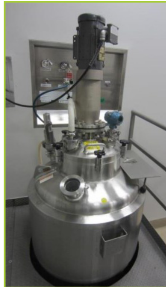
NIRO PMA 800 HIGH SHEAR GRANULATOR . STAINLESS STEEL CONSTRUCTION, 800 LITER DESIGN, JACKETED BOWL WITH 100 GAL. SOLUTION TANK, EASTON MIXER MODEL FRG-5CM, ACTUATOR, WITH SERVO O LIFT BIN LIFT FOR A 38" BIN, BIN ACTUATOR VALVES, CHUTES, 1 SKID ASSORTED SEALS, STAINLESS STEEL CHUTES. S/N 99160.0001
