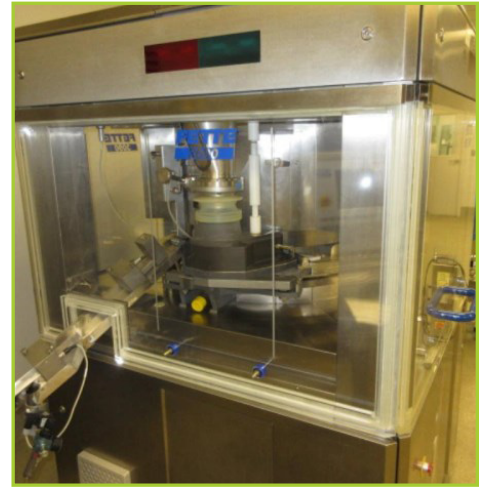
WILHELM FETTE GMBH 3090 DOUBLE SIDETABLET PRESS, (2001) , 50-STATION TURRET ASSEMBLY CURRENTLY INSTALLED, MAX. PRESSURE FORCE: 100 (120) KN, MAX. PREPRESSURE FORCE 100 (120) KN, PITCH CIRCLE DIAMETER: 680 MM, TOP PUNCH INSERTION DEPTH: 2-4 (8/12) MM, INCLUDES INCHING BOX, FREE STANDING OPERATOR CONSOLE & CONTROL CABINET, POWER CONSUMPTION 16/21 KW, 400VAC, 50/60HZ, 3PH
