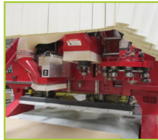
CMS SPEED-2-TAVOLE TWIN-TABLE CNC ROUTER [S/N-3254 ; YEAR-2003]. WITH GE FANUC PANEL #1 CNC CONTROL ; (ALSO INCLUDES EXTERNAL IBM MT-M-9964-ABU PC COMPUTER, DELL 17" MONITOR AND HP 1020 PRINTER) ; 18-HP ; 6,000-RPM ; 40-TAPER SPINDLE ; (2 TOTAL WORK TABLES) FRONT TABLE WORKING AREA 64"X142" AND BACK TABLE WORKING AREA 81"X142" ; CARTER LASER INDICATOR ; 52 STATION TOOL CHANGER AND 13 RESTING PODS ; APPROXIMATELY 5-HP VACUUM PUMP ; COOLANT SYSTEM WITH PUMP
