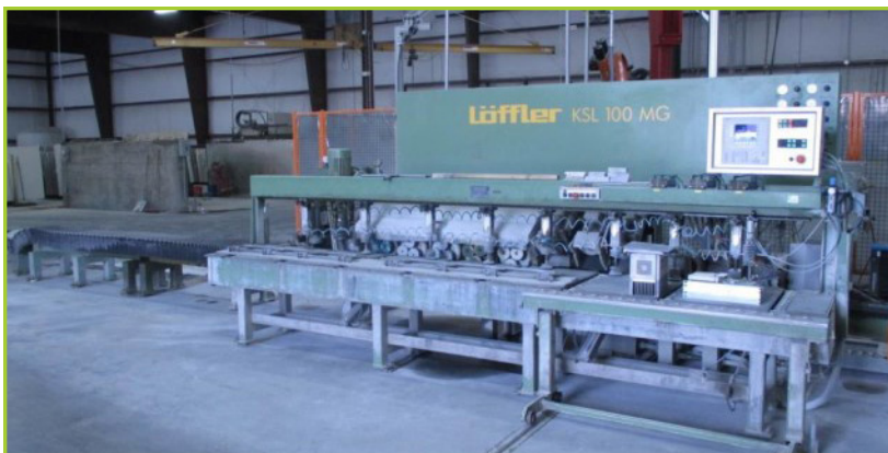
LÖFFLER KSL 100MG CNC TRAVELING EDGE POLISHER WITH SIEMENS SIMATIC C7 CNC CONTROL, (3) UPPER & (3) LOWER CHAMFERING HEADS EACH WITH APPROXIMATELY 2.6-HP WORK HEADS, (5) APPROXIMATELY 5-HP FACE POLISHING HEADS, 15' X 27.5" WORK TABLE WITH (8) HOLD-DOWNS & (8) ROLLER BED STRIPS, APPROXIMATELY 45' OVERALL TABLE TRAVEL, 9.84" MAXIMUM WORK THICKNESS. YR 2003
