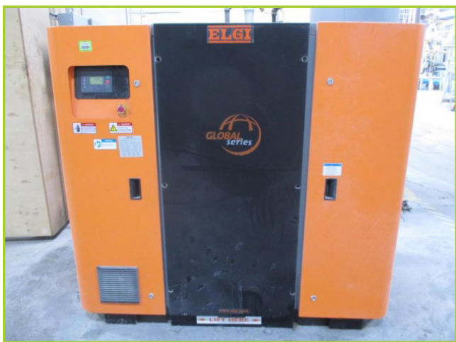
ELGI E37-125 50-HP AIR-COOLED SCREW TYPE AIR COMPRESSOR , (2013), WITH (2) APPROX. 1-HP BLOWERS, PROGRAMMABLE LOGIC CONTROL, 4,021-HOURS REPORTED, ALSO WITH STEEL FAB VERTICAL 250 GAL AIR TANK AND AURORA 2.5 HP REFRIGERATED AIR DRYER MODEL RDV0250-04
