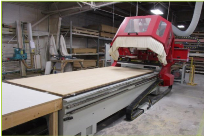
ANDERSON GROUP STRATOS/PRO BRIDGE-TYPE CNC ROUTER [S/N-FAANCST04161 ; YEAR-2015]. [10- POSITION AUTO TOOL CHANGER ; MULTI-FUNCTION ; MAX SPINDLE SPEED 24,000-RPM ; 61" X 145" TABLE ; CONTROLLER CABINET WITH INTERNAL WINDOWS BASED PC CONTROL ; (ALSO INCLUDES EXTERNAL DELL OPTIPLEX-3010 PC COMPUTER AND DELL 22" MONITOR) ; TOSOKU PENDANT CONTROL ; WITH OPTIONAL FEED BELT CONVEYOR SECTION- 67" X 117" ; (2) BECKER 10-HP VACUUM PUMP
