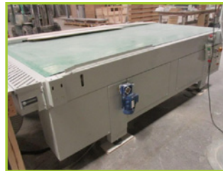
ANDERSON GROUP STRATOS/PRO BRIDGE-TYPE CNC ROUTER [S/N-FAANCST04161 ; YEAR-2015]. [10- POSITION AUTO TOOL CHANGER ; MULTI-FUNCTION ; MAX SPINDLE SPEED 24,000-RPM ; 61" X 145" TABLE ; CONTROLLER CABINET WITH INTERNAL WINDOWS BASED PC CONTROL ; (ALSO INCLUDES EXTERNAL DELL OPTIPLEX-3010 PC COMPUTER AND DELL 22" MONITOR) ; TOSOKU PENDANT CONTROL ; WITH OPTIONAL FEED BELT CONVEYOR SECTION- 67" X 117" ; (2) BECKER 10-HP VACUUM PUMP
