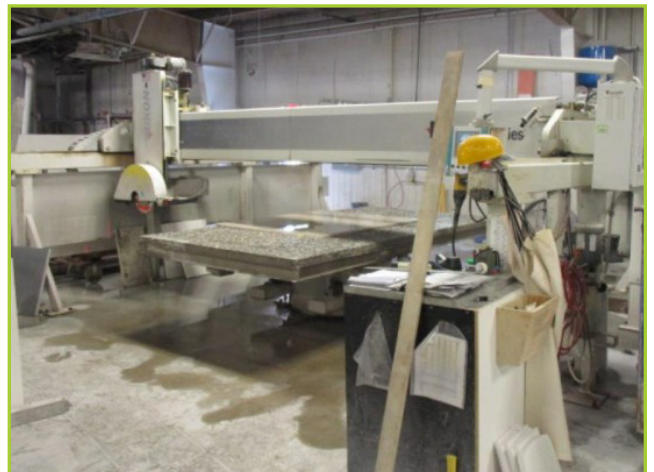
PARK INDUSTRIES YUKON PROGRAMMABLE BRIDGE SAW [S/N-3-04-1570 ; YEAR-2004]. WITH SIEMENS SIMATIC TOUCH-SCREEN PROGRAMMABLE LOGIC CONTROL ; 20-HP SAW HEAD MOTOR ; 24" MAXIMUM BLADE CAPACITY ; 6' X 11' PNEUMATIC TILTING WORK TABLE WITH MANUAL ROTATION ; 12' SAW HEAD CROSS TRAVEL ; 12' GANTRY TRAVEL . APPROXIMATELY 3-HP CROSS TRAVEL & GANTRY TRAVEL MOTORS, SIDE-MOUNTED LASER INDICATOR
