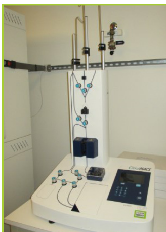
MILTENYI BIOTEC CLINIMACS PLUS MAGNETIC CELL SEPARATOR REAGENT SYSTEM. POWER: 100-240V, 50/60HZ, 180VA. INCLUDES: TUBING SETS, SEPARATION COLUMNS; MANUAL
