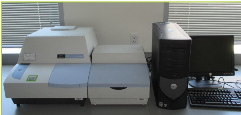
PERKIN ELMER VICTOR3 1420-032 MULTILABEL PLATE READER WITH LIQUID INJECTOR. FLUORESCENCE POLARIZATION: 400-850* NM, TIME-RESOLVED FLUORESCENCE (TRF): DUAL WINDOW TRF, DUAL EMISSION MEASUREMENTS; LUMINESCENCE: GLOW, FLASH AND DUAL LUMINESCENCE; ABSORBANCE: 340-800 NM, UV ABSORBANCE: 260 NM/280 NM. INCLUDES: DELL CELERON TOWER COMPUTER [HARDDRIVE WIPED], 14" MONITOR, KEYBOARD
