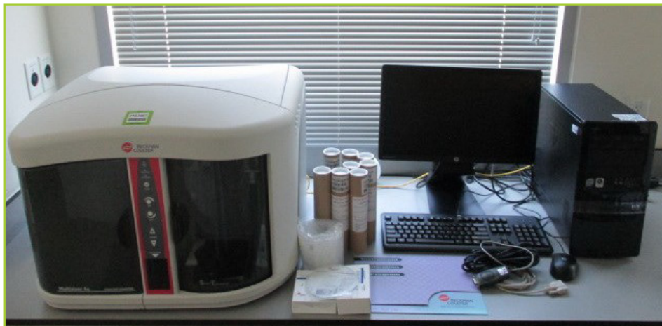
BECKMAN COULTER MULTISIZER 4E PARTICLE SIZE ANALYZER. PARTICLE SIZE RANGE: 0.2 UM TO 1600 UM IN DIAMETER. 0.033 FL TO 2.145 X 109 FL OR UM3 IN VOLUME; APERTURE DIAMETER: 10 UM TO 2000 UM APERTURES (NOMINAL DIAMETERS); POWER: 100-240V, 50/60HZ, 210W. INCLUDES: HP COMPAQ CORE2 DUO TOWER COMPUTER [HARDDRIVE WIPED], 19" MONITOR, KEYBOARD AND MOUSE.
