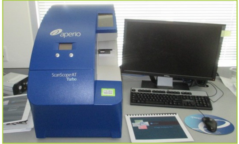
LEICA / APERIO SCANSCOPE AT TURBO DIGITAL PATHOLOGY SLIDE SCANNER. FEATURES: SCANS UP TO 400 1X3" TISSUE SLIDES UNATTENDED, 20X AT AN AVERAGE RATE OF 33 SLIDES PER HOUR, 40X AT AN AVERAGE RATE OF 12 SLIDES PER HOUR; E-SLIDES ARE 24-BIT COLOR WITH GIGAPIXEL RESOLUTION, SCAN SINGLE 2X3" SLIDES ONE AT A TIME. INCLUDES: TECHNIQUIP ILLUMINATOR; HP Z600 TOWER COMPUTER [HARDDRIVE WIPED], 24" MONITOR, KEYBOARD AND MOUSE.
