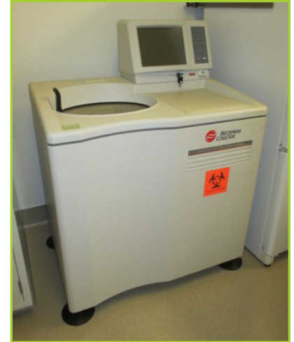
BECKMAN COULTER OPTIMA L-100 XP FLOOR MODEL REFRIGERATED /VACUUM ULTRACENTRIFUGE WITH (4) ROTORS. INCLUDES: (1) SW 32 TI 6-PLACE TUBE; (1) SW 40 TI 6-PLACE TUBE; (1) 100 TI 8-PLACE FIXED-ANGLE
