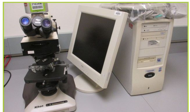
NIKON OPTIPHOT-2 TRINOCULAR RESEARCH MICROSCOPE. FEATURES: 5-POSITION NOSEPIECE WITH THE FOLLOWING OBJECTIVES: (1) PLAN APO 60X/1.40 OIL 160/0.17, (1) PLAN APO 40X/0.95 160/0.11-0.23, (1) PLAN 20X/0.50 160/0.17, (1) E 10X/0.25 PH1 DL 160/-, (1) PLAN 4X/0.13 DL 160/-, (2) CFWN 10X/20 EYEPIECES; ACHR-APL CON.A 1.4 UNIVERSAL CONDENSER, DIAPHRAGM SHUTTER; XY KNOB STAGE, Z-AXIS CONTROLS, UPPER AND LOWER 12V 100W HALOGEN LAMPS; SPECTRAL IMAGING SD000302A CAMERA. INCLUDES: P4 TOWER COMPUTER [HARDDRIVE WIPED], 17" MONITOR, KEYBOARD
