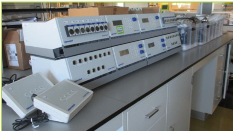
EPPENDORF DASGIP BENCHTOP BIOREACTOR SYSTEM. INCLUDES: (2) MP8 MULTI PUMP MODULES, (2) PH4P04 PH MONITORS, (2) TC4SC4 TEMPERATURE AND AGITATION CONTROLLERS, (2) MX4/4 GAS MIXERS, (2) EGC4 PELTIER EXHAUST CONDENSERS; (4) TOTE BINS OF PROBES, CABLES, AND BOTTLES; CONTROL COMPUTER, 17" MONITOR, KEYBOARD AND MOUSE.
