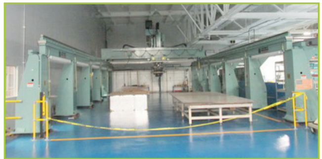
CINCINNATI MILACRON 5-AXIS FLAT TAPE CNC LAYER MACHINE, 26' X 61', AB 975 CONTROLS, TRAVEL: X-AXIS 648", Y-AXIS 200", Z-AXIS 36", ROTATION C-AXIS +/- 190 DEGREE, CUTTER ANGLE D-AXIS +1 TO 181 DEGREE, CUTTER TRAVEL V-AXIS 6" & 12" TAPE 14.25", LONG/TRANSVERSE FEED RATE 0.1 TO 1800IN/MIN, VERTICAL FEED 0.1 TO 600IN/MIN, C-AXIS 0.1-9000 DPM, D-AXIS 0.1-10,800DPM, V-AXIS 0.1 - 1200IN/MIN, U-AXIS 0.1-1800IN/ MINZ2TRACK 150N/MIN, WORK SURFACE 648" X 200", WORK HEIGHT 27" TO 63", 8-SPINDLE.
