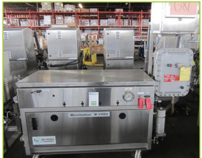
MICROFLUIDICS CORP 210 EH HIGH SHEAR HIGH PRESSURE LIQUID MIXER. 316 S/S CONTACT PARTS, NOMINAL FLOW RATE OF 1 TO 1.5 GPM. OPERATING PRESSURES 2,500 TO 12,000 PSI, 15 HP HAZARDOUS LOCATION RATED MOTOR, EXPLOSION PROOF DISCONNECT, EXPLOSION PROOF POWER CONTROL UNIT. SN# 200089. YEAR: 2000
