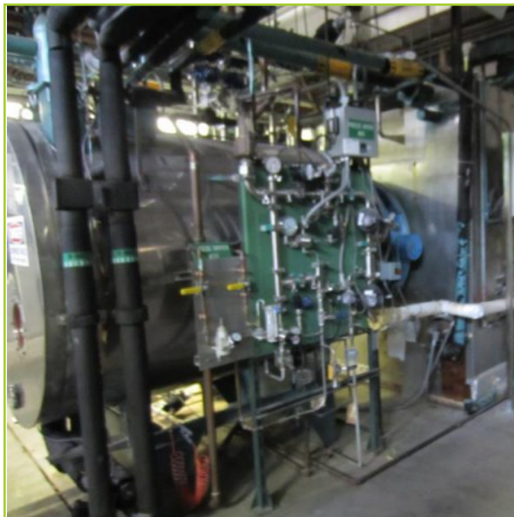
STOKES 360 SQ FT. FREEZE DRYER. REBUILT IN 2008. CHAMBER MAWP 18PSI @ 260°F, MDMT -20°F @ 18PSI, 2 SKIDS, CONDENSER YR 2003 & REFRIGERATION. UP GRADED CONTROLS WITH OLD CONTROLS FOR BACKUP
