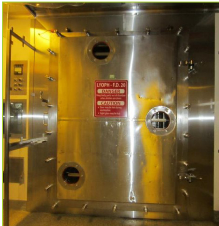
STOKES 360 SQ FT. FREEZE DRYER. REBUILT IN 2008. CHAMBER MAWP 18PSI @ 260°F, MDMT -20°F @ 18PSI, 2 SKIDS, CONDENSER YR 2003 & REFRIGERATION. UP GRADED CONTROLS WITH OLD CONTROLS FOR BACKUP
