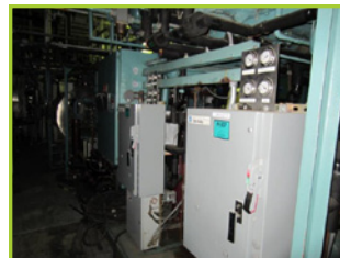
STOKES 264 SQ FT. FREEZE DRYER. REBUILT IN 2008. 2 SKIDS, CONDENSER & REFRIGERATION. UP GRADED CONTROLS WITH OLD CONTROLS FOR BACKUP
