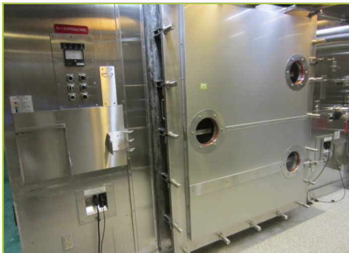
STOKES 264 SQ FT. FREEZE DRYER. REBUILT IN 2008. 2 SKIDS, CONDENSER & REFRIGERATION. UP GRADED CONTROLS WITH OLD CONTROLS FOR BACKUP
