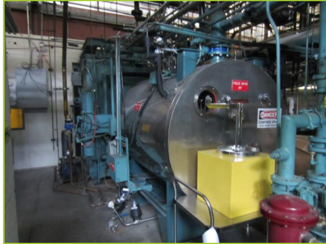
STOKES 264 SQ. FT. FREEZE DRYER. CHAMBER MAWP 18PSI @ 260°F, MDMT -20°F @ 18PSI 2 SKIDS, REBUILT IN 2008, CONDENSER YR 2003 & REFRIGERATION (2) COPELAND 6TM1-2000-TSK-800 COMPRESSORS. UP GRADED CONTROLS WITH OLD CONTROLS FOR BACKUP.
