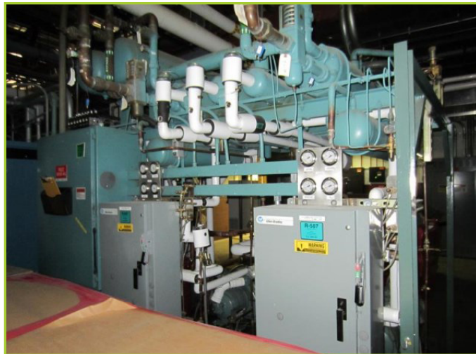
STOKES 264 SQ. FT. FREEZE DRYER. CHAMBER MAWP 25PSI @ 300°F, MDMT -40°F @ 25PSI 2 SKIDS CONDENSER YR 2004 & REFRIGERATION. REBUILT IN 2008, UP GRADED CONTROLS WITH OLD CONTROLS FOR BACKUP
