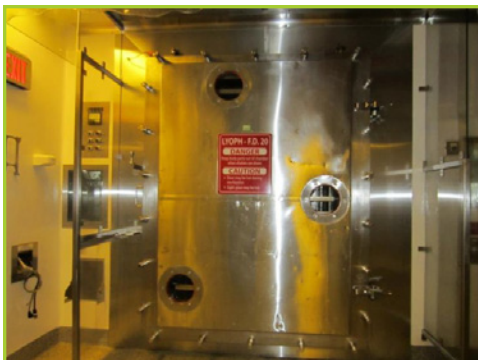
STOKES 360 SQ. FT. FREEZE DRYER. REBUILT IN 2008. CHAMBER MAWP 18PSI @ 260°F, MDMT -20°F @ 18PSI, 2 SKIDS, CONDENSER YR 2003 & REFRIGERATION. UP GRADED CONTROLS WITH OLD CONTROLS FOR BACKUP
