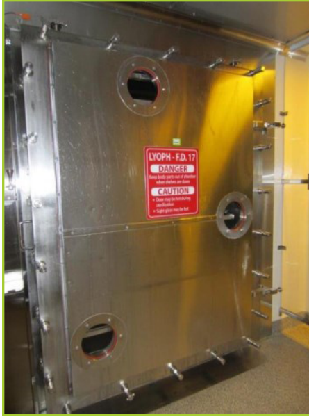
STOKES 264 SQ. FT. FREEZE DRYER. CHAMBER MAWP 18PSI @ 260°F, MDMT -20°F @ 18PSI 2 SKIDS, REBUILT IN 2008, CONDENSER YR 2003 & REFRIGERATION (2) COPELAND 6TM1-2000-TSK-800 COMPRESSORS. UP GRADED CONTROLS WITH OLD CONTROLS FOR BACKUP.
