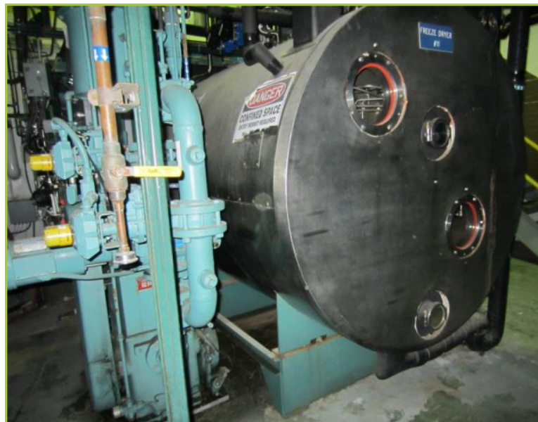
STOKES 264 SQ FT. FREEZE DRYER. REBUILT IN 2008. 2 SKIDS, CONDENSER & REFRIGERATION. UP GRADED CONTROLS WITH OLD CONTROLS FOR BACKUP
