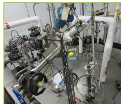
16,500 LITER STAINLESS STEEL TANK. VESSEL VOLUME 5000GAL, VESSEL M.A.W.R.50-15 PSI @350°F, NATIONAL BOARD # 4627. 8'6" DIA X 11' .500THK 316L STEEL YR 2000 NON JACKETED.YEAR: 2000
