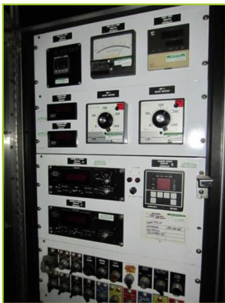
STOKES 264 SQ FT. FREEZE DRYER. REBUILT IN 2008. 2 SKIDS, CONDENSER & REFRIGERATION. UP GRADED CONTROLS WITH OLD CONTROLS FOR BACKUP
