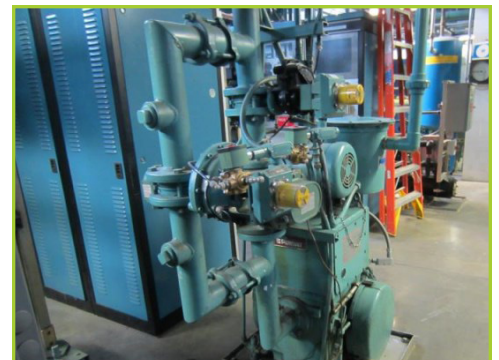
STOKES 360 SQ. FT. FREEZE DRYER. REBUILT IN 2008. CHAMBER MAWP 18PSI @ 260°F, MDMT -20°F @ 18PSI, 2 SKIDS, CONDENSER YR 2003 & REFRIGERATION. UP GRADED CONTROLS WITH OLD CONTROLS FOR BACKUP
