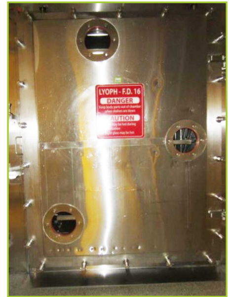
STOKES 264 SQ. FT. FREEZE DRYER. CHAMBER MAWP 18PSI @ 260°F, MDMT -20°F @ 18PSI 2 SKIDS, REBUILT IN 2008, CONDENSER YR 2003 & REFRIGERATION (2) COPELAND 6TM1-2000-TSK-800 COMPRESSORS. UP GRADED CONTROLS WITH OLD CONTROLS FOR BACKUP.
