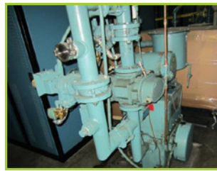
STOKES 264 SQ. FT. FREEZE DRYER. CHAMBER MAWP 25PSI @ 300°F, MDMT -40°F @ 25PSI 2 SKIDS CONDENSER YR 2004 & REFRIGERATION. REBUILT IN 2008, UP GRADED CONTROLS WITH OLD CONTROLS FOR BACKUP
