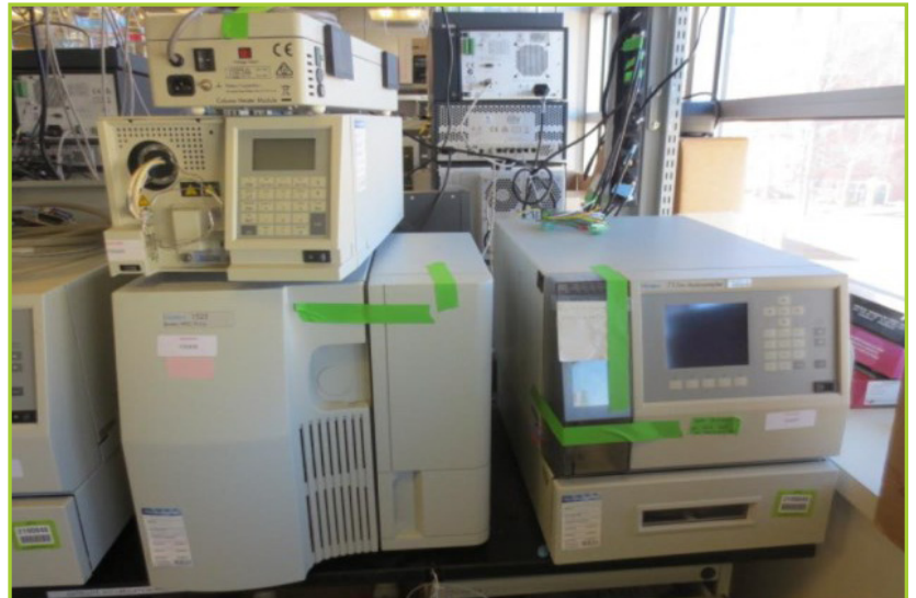
WATERS 717+, 1525, 2489, CHM CONSISTING OF: 1 - 717+ AUTOSAMPLER S/N C0871P714M, 1- 1525 BINARY HPLC PUMP S/N A0825P158A, 1- 2489 UV / VISIBLE DETECTOR S/N D0887E045M, 1- CHM S/N K08CHM664M 223
