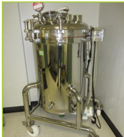
FELDEMEIER MOBILE MEDIA VESSEL, (2001), MAWP 50, PSI @ 300, MIN. DESIGN METAL TEMPERATURE -20 @ 50 PSI, INCLUDES NOVASEPTIC GMP500 AGITATION DRIVE UNIT, HEAVY-DUTY CASTORS
