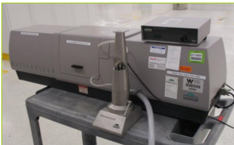
MALVERN MSS/MASTERSIZER PARTICLE SIZE ANALYZER INSTRUMENT, WITH MAM2045 DRY POWDER FEEDER, AND DIF2021 SMALL VOLUME SAMPLE DISPERSION UNIT WITH CONTROLLER
