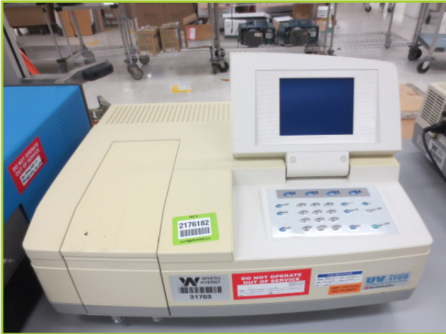
SHIMADZU UV-1700 PHARM SPEC A11024336527 UV/VISIBLE SPECTROPHOTOMETER
