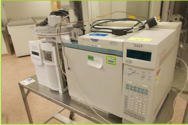
AGILENT SYSTEM COMPLETE W/ G2613A INJECTOR, G2614A AUTOSAMPLER TRAY, AND TRIPLE AXIS DETECTOR
