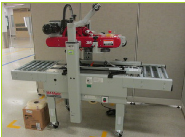
3M MATIC 700A ADJUSTABLE CASE SEALER, W/TAPE, 115V, 3.8 A 60 HZ, 440W, 1-PHASE, (2010)
