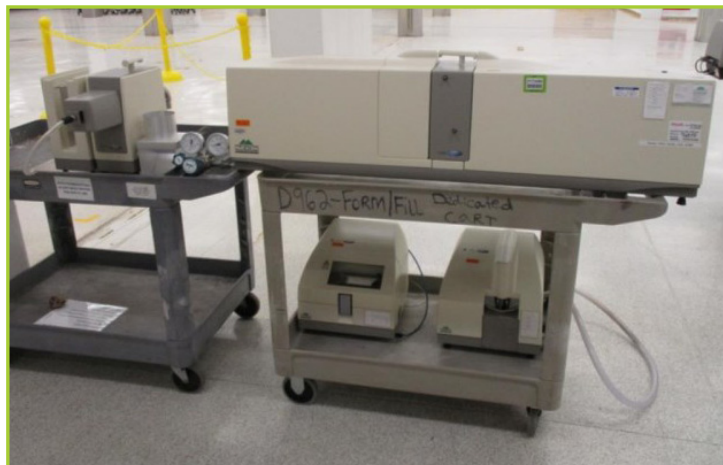
MALVERN APA2000/MASTERSIZER-2000 PARTICLE SIZE ANALYZER INSTRUMENT, WITH ADA2000/ SCIRROCCO-2000 DRY POWDER FEEDER AND AWA2001/HYDRO-2000S LIQUID ANALYSIS WET SAMPLE DISPERSION UNIT. SYSTEM S/N-MAL101788 ; YEAR 2005
