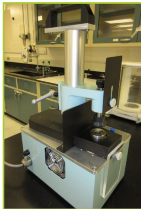
ISAI APK01-S BENCHTOP VIAL LIQUID INSPECTION MACHINE
