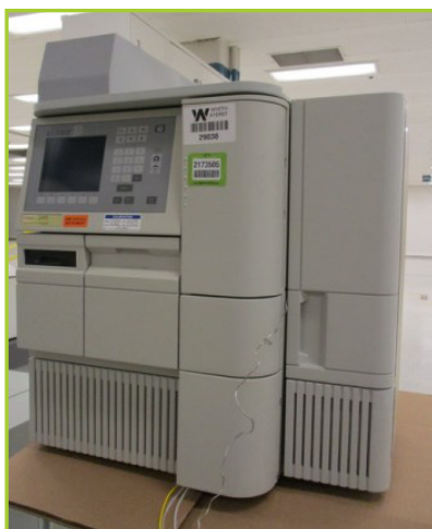
WATERS ALLIANCE-2695 (CODE SM4) SOLVENT AND SAMPLE MANAGEMENT, HPLC SEPARATIONS MODULE
