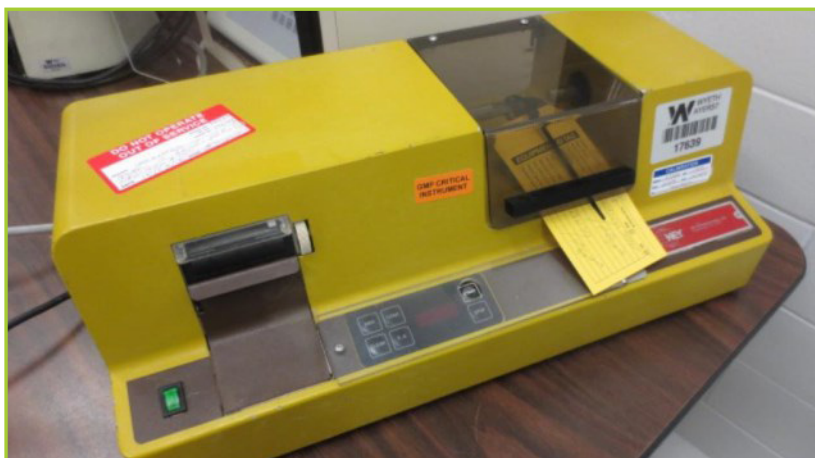
KEY PTB501 H-2335/J TABLET HARDNESS TESTER
