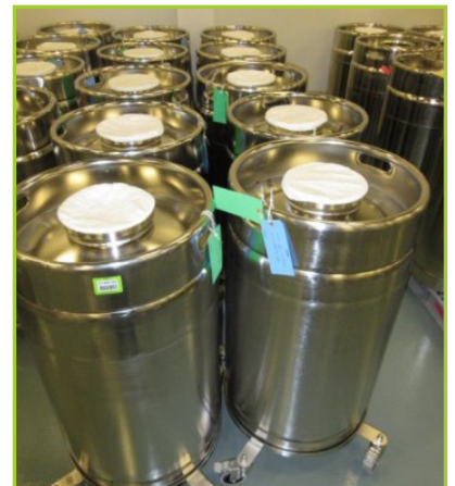
LOT OF (10) ALFRED BOLZ 200L FORMULATION VESSELS, 316 STAINLESS STEEL CONSTRUCTION, PRESSURE/TEMPERATURE -1/4 BAR / -35/+150 C
