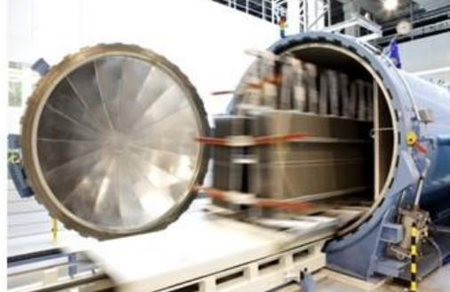
**10:** Encapsulation / Autoclave
