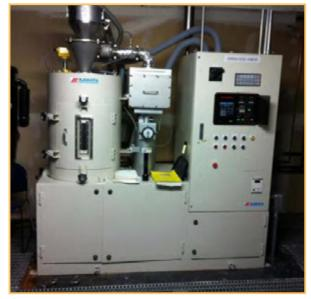
PC DRYER Kawata CDA-150 208 V 100A; 330 liter hopper capacity
