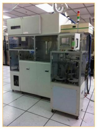
ORIGIN ELECTRIC COMPANY HARD COATER Model # CD-2UCL Manufacture Date: March 1995. Converted lacquer coater. For hard coating read-side of CD or DVD media
