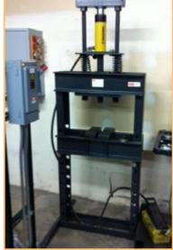
DAYTON 25 TON BENCH PRESS 5M468 25 Ton all hydraulic bench press. Manual Operation
