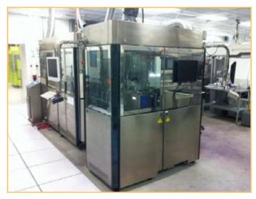
**STEAG HAMATECH 3503 DVD-R STEAG 3503 PRODUCTION LINE:** including: dual cathode SteagTaurus metalizer, 2 ETA disc scanners; 2 Netstal 600 DJ-600-70 hybrid molding machines (2004) (1) AWM ver3.4 mold (1) AWM ver6.1 mold.This line is capable of producing DVD-R, DVD+R, DVD ROM with 1 or 2 reflective layers @ 4 second cycle
