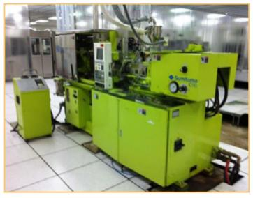
4 -SUMITOMO SD-30, 30TON ALL HYDRAULIC INJECTION MOLDING MACHINES 2-1997, 2-1996, Screw diameter: 25 mm Shot size: 25 cm Screw stroke: 50 mm
