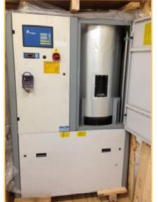
**PIOVAN 6.6KW PC DRYER SYSTEM** The CDN1/2 Drying Units combine the dryer with a drying hopper and conveying unit to create a fully integrated system in one mobile assembly
