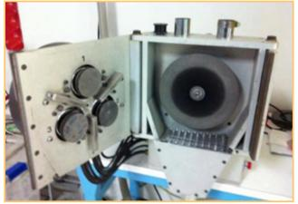
WEXIT SB-2 STAMPER BACKSANDER 110/208 VAC 8.8/4.4A 50/60 Hz3 rotating sanding pads. Rotating stamper holder. Vacuum Port for removing dust.
