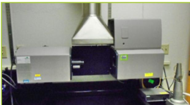
MALVERN MASTERSIZER-S (MSS) LASER PARTICLE SIZE ANALYZER
