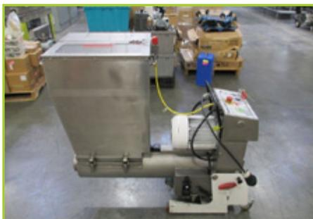
PLASTIC RECYCLING MACHINERY MGK 400/175TL RESIN GRINDER
