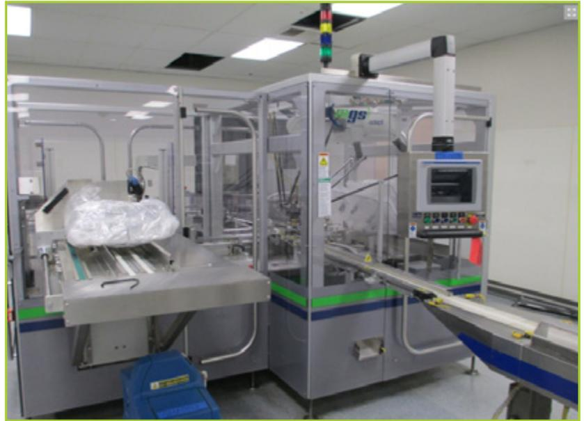
MGS MODEL TLC PICK AND PLACE ROBOTIC PACKAGING MACHINE
