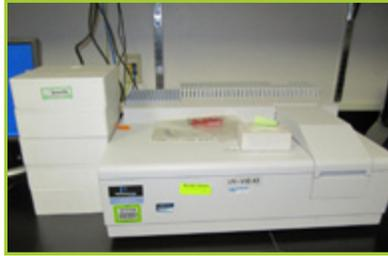
PERKIN ELMER LAMBDA 25 UV/VIS SPECTROMETER
