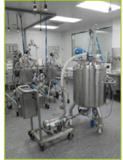
**ALLEGHENY BRADFORD CORP. DIMPLE JACKETED 316 L STAINLESS STEEL 150 LITER CAPACITY BUFFER VESSEL**
