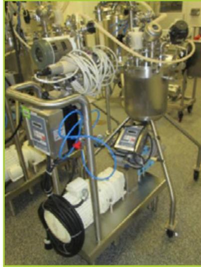
**AMERICAN ALLOY JACKETED 80 PSI 16 LITER CAPACITY 316 L STAINLESS STEEL VESSEL WITH SPRAY BALL**
