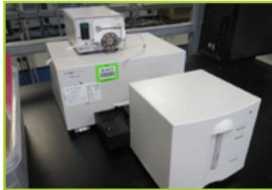
AGILENT 8453 UV-VISIBLE SPECTROSCOPE
