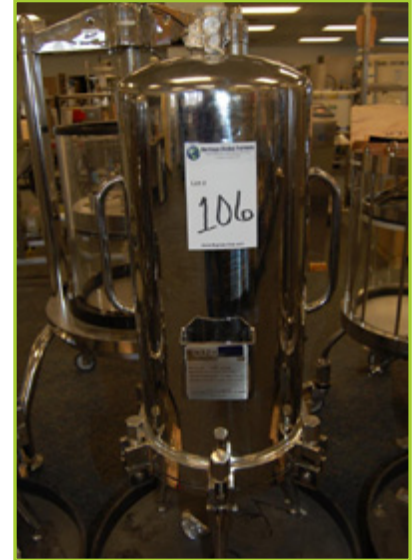
ALLEGHENY BRADFORD CORP. DIMPLE JACKETED 316 L STAINLESS STEEL 150 LITER CAPACITY BUFFER VESSEL
