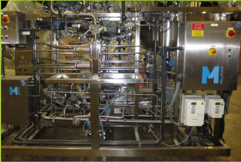
BIOPHARM ENGINEERED SYSTEMS/MILLIPORE 40 SQ-M-MF FILTER SKID SYSTEM
