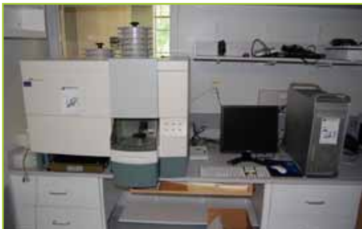
BECTON DICKINSON FACS CALIBUR W/FACS LOADER, ELECTRONICS, MAC PRO MOD. A1289 PC
