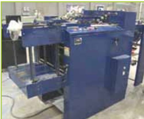
L HERMITE EA4 BOOKLET HOLE PUNCHING MACHINE. W/ 34-HOLE PUNCH STATION, CHAIN TYPE FEED TABLE, DOUBLE STRAND BELT DELIVERY TABLE, LEESON SPEEDMASTER CONTROLLER AND SUPPORTS
