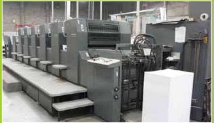
HEIDELBERG SPEEDMASTER SM 74-6-P3-L 6 COLOR SHEET FED OFF SET PRINTING PRESS. SEMI-AUTOMATIC 20.5" X 29.1". (2) TRESU ROYCE, INC. DAMPENING WATER CIRCULATING UNITS; (4) ROYSE SPACE SAFER CIRCULATING UNITS; 6 COLOR L LUSTER COATER. INFRARED DRYER. CHILLING UNIT. PLATE BENDER. ATLAS COPCO OIL FREE AIR COMPRESSOR. ASSOCIATED PUMPS, DUCTWORK, CONTROLS AND SUPPORTS, 137,660,326 AS 16 JULY 2014 IMPRESSIONS INDICATED
