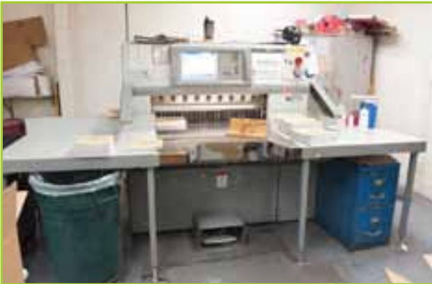
MOHR POLAR 92X PAPER CUTTER; 36.25" CUTTING WIDTH, YEAR OF MFG. 2007
