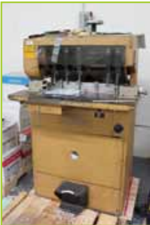
CHALLENGE MS-10A PAPER DRILL, 5-HEADS, 10 HOLE MAX, 1/2" MAX
