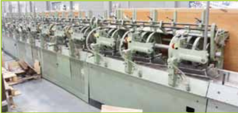
MULLER MARTINI SIDE STITCH LINE, 12-POCKET WITH PERFECT BINDER' INCLUDING BUT NOT LIMITED TO: (4) HANS MULLER MARTINI GATHERERS MODEL TYPE 201 S/N'S 108379, 114959, 114956, 113349. W/ FEED TABLE, APPROX. 4'L; GRAPH A (1) DOUBLE HEAD WIRE STAPLE STATION MODEL SH S/N 62569, W/ EXIT CONVEYOR SECTION, APPROX. 10'L; (1) MULLER MARTINI PERFECT BINDER MODEL PANDA 1530 L4 S/N 945870 C850, W/ FEED TABLE, PLASTIC BELT TYPE, APPROX. 1'W X 42'L, TRANSFER CONVEYOR SECTION, APPROX. 6'L. DOUBLE STRAND FEED BELT CONVEYOR SECTION, APPROX. 4'L; PLASTIC FEED BELT CONVEYOR SECTION, APPROX. 12'W X 8'L, U-SHAPED; ASSOCIATED BLOWERS, SUPPORTS AND CONTROLS. CONVEYOR CONTROLS ARE IN COMMON FREE STANDING CONTROL STATION
