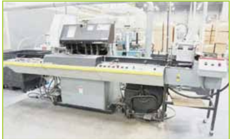
DEXTER-LAWSON PRODUCTS LTD. CLASSIC H/DCHR PAPER DRILLING MACHINE 5 HP, W/ MATERIAL HANDLER. MODEL 18CV S/N 18CV/6097. CONFIGURED FOR 2 BOOKS WITH 3 DRILLS EACH AT A TIME.
