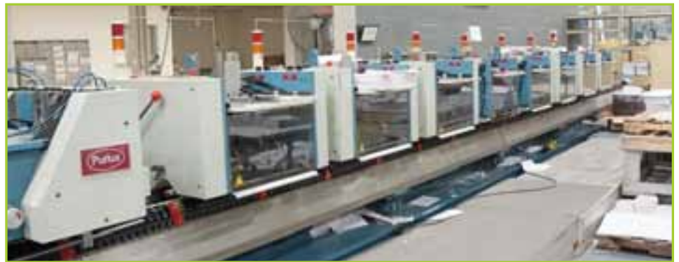
PURLUX/VIJUK LQD8E SADDLE STITCH LINE, 8-POCKET. INCLUDING BUT NOT LIMITED TO: (8) PURLUX VIJUK FEEDERS WITH RAILS MODEL DYQ440E. (1) COVER FEEDER MODEL ZYDY440E. (1) WIRE BONDING MODULE MODEL DDQ8E, W/ (2) HOHNER M50/8 STITCHING HEADS AND STATION INDICATOR LIGHT PANEL; (1) CONTROL CONSOLE MODEL LQD8. (1) FOLDING STATION MODEL N/A. (1) THREE-KNIFE TRIMMER MODEL QS8E, W/ FEED CONVEYOR TABLE AND HOOD; (1) LINEAR DELIVERY TABLE MODEL SZQ440, ASSOCIATED VACUUM PUMPS, BLOWERS, DUCTWORK, CONTROLS AND SUPPORTS, YEAR OF MFG. 2005.
