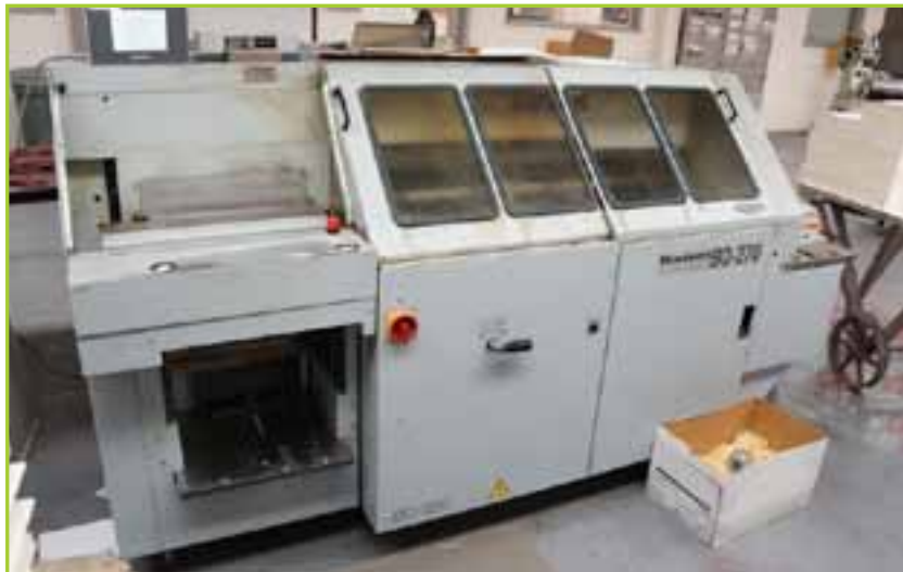
HORIZON INTERNATIONAL BQ-270 PERFECT BINDER MACHINE; 1-50MM THICKNESS, 320 X 320MM MAX. SIZE
