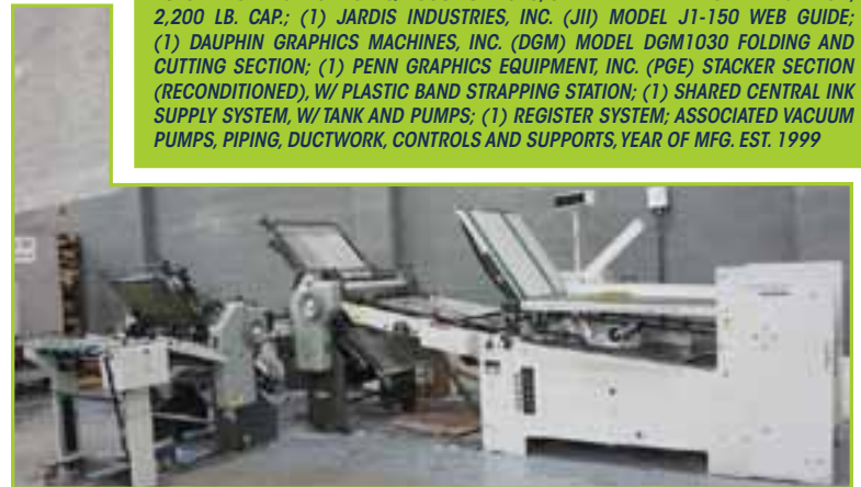
HEIDELBERG/STAHL STAHLFOLDER SERIES 1400 1430A-C-3 16 PAGE CONTINUOUS FEED FOLDING MACHINE, 26" X 40"W/ (3) RIGHT ANGLE ROLL-IN TYPE FOLDERS, MODELS B1430A-4-PAK-3
