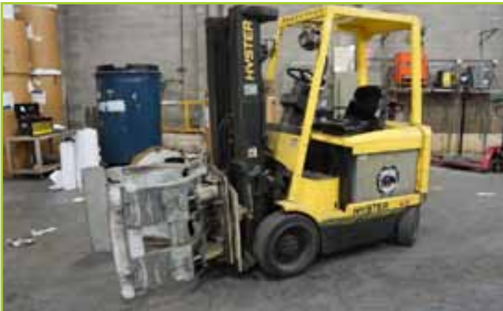
HYSTER E60XM FORKLIFT, 5,750 LB. CAP., ELECTRIC POWERED, 3-STAGE MAST, 193.7" MAX. HEIGHT LIFT CAP., HARD TIRES, OVERHEAD GUARD, W/ CASCADE ROTARY ROLL CLAMP ATTACHMENT, 2,359 HRS.
