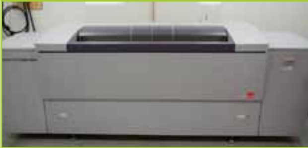
KODAK TRENDSETTER 800 III QUANTUM THERMAL IMAGING PLATE SETTER, 830MM, SEMIAUTOMATIC EXTERNAL DRUM, 450 LPI MAX. LINE SCREEN, W/ ASSOCIATED ACCESSORIES, PIPING, CONTROLS AND SUPPORTS, DELL COMPUTER SYSTEM. AIR FILTRATION MODULE. 1 R INLINE COMPRESSED AIR FILTER.
