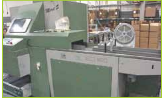
MULLER MARTINI MERIT S 3671 THREE-KNIFE TRIMMER W/ FEED TABLE, APPROX. 6'L. PANELWARE PROGRAMMABLE CONTROLLER, HYTROL MODEL PCX BELT SCRAP CONVEYOR, APPROX. 2'W X 10'L; HYTROL MODEL TA EXIT BELT CONVEYOR SECTION, APPROX. 2'W X 6'L. ASSOCIATED PIPING, SUPPORTS AND CONTROLS YEAR OF MFG. 2000.
