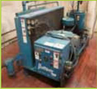
PATTONS (QUINCY) PQ 200A SKID MOUNTED ROTARY SCREW AIR COMPRESSOR, 50 HP
