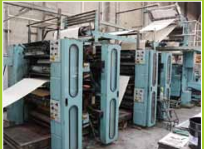
DAUPHIN GRAPHICS MACHINES, INC. (DGM) 435-3 4 COLOR WEB PRINTING PRESS, 36" OFFSET COLD SET, WEB FED, 4-COLOR, 36"W, W/ (2) PRINTING SECTIONS, EACH 2-COLOR, (1) MODEL 430 CONTROL PANEL W/ FINCOR DIGITAL SYSTEM; (2) MARTIN AUTOMATIC 2-ROLL SPLICERS/ ACCUMULATORS, OVERHEAD PAPER ROLL LIFT STATION, 2,200 LB. CAP.; (1) JARDIS INDUSTRIES, INC. (JII) MODEL J1-150 WEB GUIDE; (1) DAUPHIN GRAPHICS MACHINES, INC. (DGM) MODEL DGM1030 FOLDING AND CUTTING SECTION; (1) PENN GRAPHICS EQUIPMENT, INC. (PGE) STACKER SECTION (RECONDITIONED), W/ PLASTIC BAND STRAPPING STATION; (1) SHARED CENTRAL INK SUPPLY SYSTEM, W/ TANK AND PUMPS; (1) REGISTER SYSTEM; ASSOCIATED VACUUM PUMPS, PIPING, DUCTWORK, CONTROLS AND SUPPORTS, YEAR OF MFG. EST. 1999
