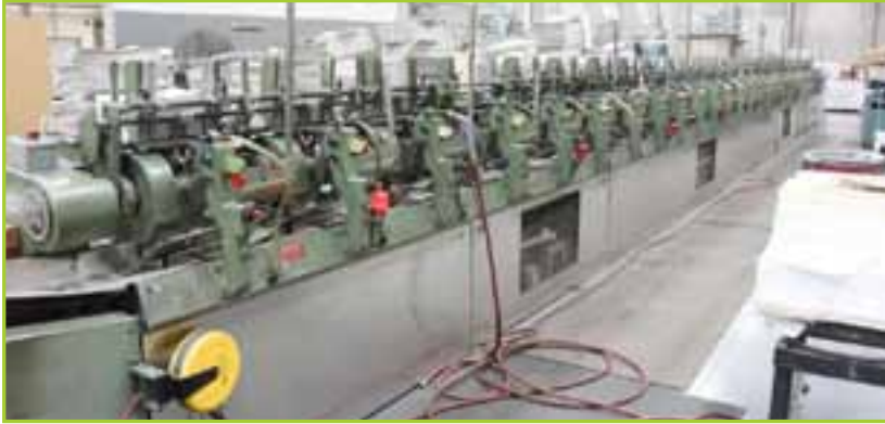
HANS MULLER MARTINI BOOK BINDING LINE R B5, 27-POCKET. INCLUDING BUT NOT LIMITED TO: (1) GRAPH A GATHERER/STACKER, 3-POCKET MODEL 1201 L7, (8) HANS MULLER MARTINI GATHERERS STACKERS, 3 POCKET MODEL 201, (1) HANS MULLER MARTINI TRANSFER CONVEYOR SECTION, APPROX. 10'L; (1) CONTROL CONSOLE, W/ CUTLER-HAMMER/EATON DIGITAL INDICATOR; (1) ROTARY BOOK GRINDER/GLUER MODEL R B5 10-CLAMPS, W/ COVER FEED STATION; STA WARM ADHESIVE MELT POT MODEL 53 CNS, STA WARM ADHESIVE MELT POT MODEL 10CNS. SKIPTRONICS INDUSTRIAL CONTROL CONSOLE (4 CONVEYORS). (1) COOLING TOWER, W/ (5) CONVEYORIZED LEVELS. (1) SPLIT PLASTIC BELT CONVEYOR, APPROX. 2'W X 6'L. (1) ARROWHEAD PLASTIC BELT EXIT CONVEYOR, APPROX. 1'W X 22'L. ASSOCIATED PUMPS, BLOWERS, DUCTWORK, CONTROLS AND SUPPORTS
