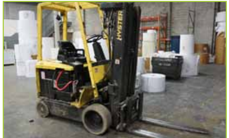
HYSTER E50Z FORKLIFT, 3,450 LB. CAP., ELECTRIC POWERED, 4-STAGE MAST, 196.9" MAX. LIFT CAP., CUSHION TIRES, OVERHEAD GUARD, W/ SIDE SHIFTER, 2,483 HRS., YEAR OF MFG. 2005
