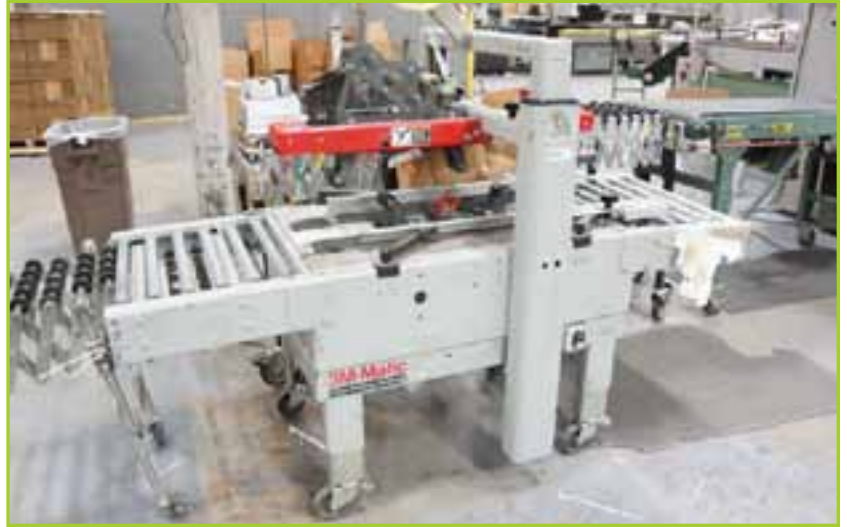
3M-MATIC 200A CASE SEALING SYSTEM, PORTABLE, W/ TOP AND BOTTOM TAPING HEADS YEAR OF MFG. 2004.
