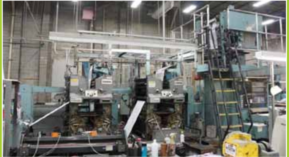
GOSS COMMUNITY IF028936 RC2552 4 COLOR WEB PRINTING PRESS, 32" OFFSET COLD SET, WEB FED, 4-COLOR, 32"W, W/ (2) GOSS MODEL COMMUNITY 2-COLOR PRINTING SECTION, (TAG #00211 & #00212); (2) MARTIN AUTOMATIC, INC. 2-ROLL SPLICERS / ACCUMULATORS, W/ PAPER ROLL LIFT STATION
