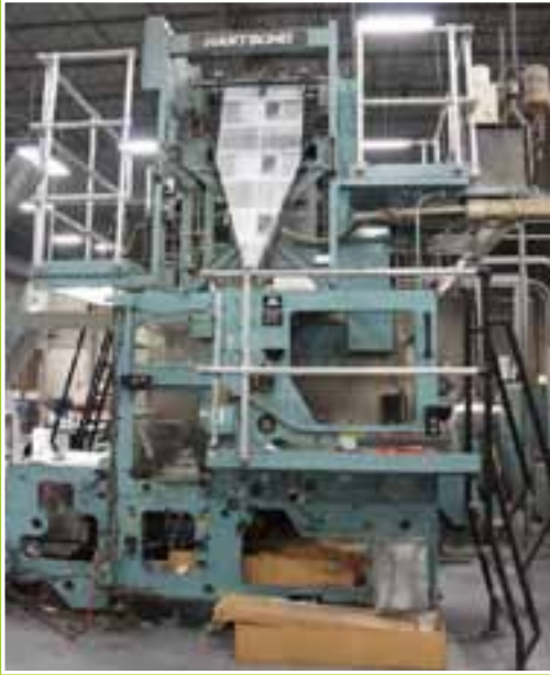
GOSS COMMUNITY IF028936 RC2552 4 COLOR WEB PRINTING PRESS, 32" OFFSET COLD SET, WEB FED, 4-COLOR, 32"W, W/ (2) GOSS MODEL COMMUNITY 2-COLOR PRINTING SECTION, (TAG #00211 & #00212); (2) MARTIN AUTOMATIC, INC. 2-ROLL SPLICERS / ACCUMULATORS, W/ PAPER ROLL LIFT STATION
