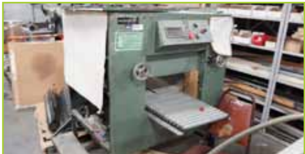
SKIPTRONICS INDUSTRIAL CONTROL THREE-KNIFE TRIMMER
