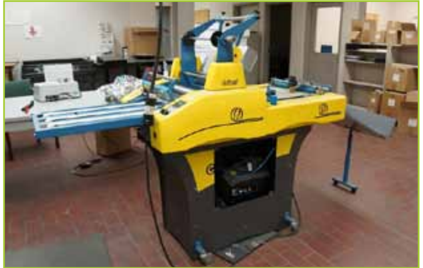
FORMICA FOLIANT GEMINI COMPRESSOR 400S LAMINATOR, SEMIAUTOMATIC HIGH PRESSURE, 380MM MAX. WIDTH, W/ CONTROLS AND ACCESSORIES YEAR OF MFG. 2008
