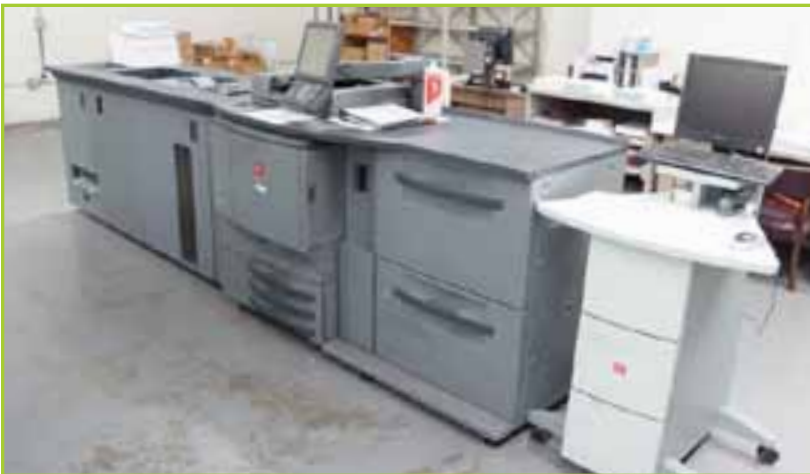
OCE C6500/CS6500 DIGITAL COLOR IMAGING PRINTING SYSTEM. 600 TO 1800 DPI, 65 PPM (8-1/2" X 11"), 36 PPM (11" X 17") PAPER SIZE, W/ FEEDERS, FINISHER, COMPUTER AND ACCESSORIES. YEAR OF MFG. 2006.
