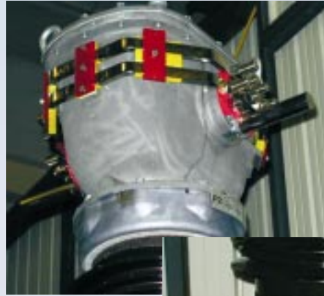
TG 245 Primary connections and high voltage sockets.
