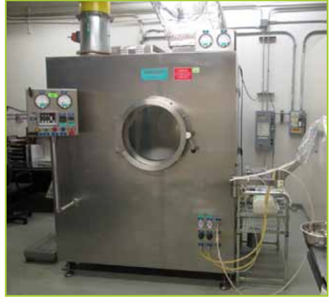
FASTCOAT SYSTEM OHARA TECHNOLOGIES 48FC FASTCOAT SYSTEM, 48 FAST COAT, MFG. 1997, CAPACITY SIZE 150 KG MAX
