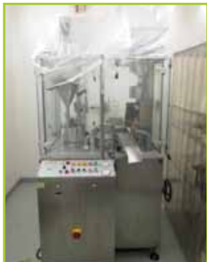
AUTO CAPSULES FILLING MACHINE KWAN DAH ENTERPRISES CO. LTD. KDF- 6 AUTO CAPSULES FILLING MACHINE, 220V, 60 HZ, 5.5 HP, MFG. 1994
