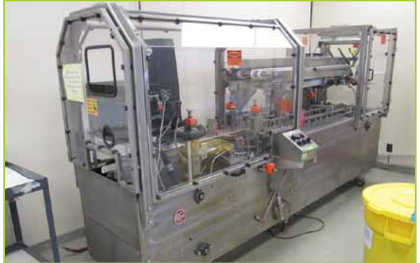
ADCO CARTONER ADCO CARTONER, APPROX. SPEED 1 PER SECOND, FOLDS AND GLUES DOWN ENDS, CODE DATING
