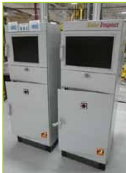
DR. SCHENK SOLAR INSPECT FLAT GLASS EDGE/SHEET INSPECT & MEASUREMENT SYSTEM , YEAR 2012. OVERALL FOOTPRINT 18'LX8'WX8'H --- SHEET WIDTH MAX 1300MM ; IN FEED ALIGNMENT CONVEYOR SECTION WITH TWO PDP LINE HEADS ; OPTICAL INSPECTION STATION WITH LED ILLUMINATORS AND TWO SC3 SMART CAMERAS (CHESS. EDGE GLASS SHEET AND EDGE DEFECT DETECTION & CLASSIFICATION ; SHEET INSPECTION SYSTEM FOR IN/ON GLASS DETECTION & CLASSIFICATION AND SQUARE-NESS ; INSPECTION UP TO 10-MICRONS) ; WITH HYFRA #CHILLY-08-C CHILLER SUPPORT ; WITH EXITING CONVEYOR SECTION. CONTROL CABINETS: (1) CONTROL CABINET WITH DR. SCHENK MAIN CONTROL COMPUTER. ALSO EV4000 WORKSTATION COMPUTER, FOR EDGE INSPECTION, IDENTIFIER AND CAMERA PROCESS. (1) CONTROL CABINET WITH DR. SCHENK EV4000 WORKSTATION COMPUTER , FOR SHEET INSPECTION. (1) CONTROLLER BOX WITH MITSUBISHI GOT-1000 OPERATOR TERMINAL, FOR ALIGNMENT/CENTERING CONVEYOR PROCESS. BLDG-ZV,FLR2,NORTH,PIF LINE.
