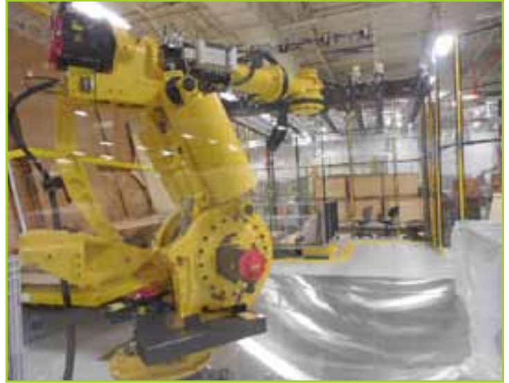
FANUC R-2000IB/210F INDUSTRIAL ROBOT (6-AXIS ; WRIST CAPACITY UP TO 210 KG ; REACH 2.60 M ; ON STAND 3'H), WITH R-30IA CONTROLLER AND I- PENDANT [ROBOT S/N-R11602214 ; CONTROLLER S/N-E11601112 ; SYS ID#F109940 ; SYS YEAR 2011]. WITH GLASS-SHEET-HANDLING URETHANE-CUPS END EFFECTOR TOOL (TOOL FOOTPRINT 5'LX4.5'W). ALSO INCLUDED: [CRATE PALLET-TURNTABLE (TURNTABLE PLC CONTROLLER NOT INCLUDED). PLATFORM FOOTPRINT 11'L TOTAL X 7'WX2'H, AND ATTACHED FENCING PANELS 12'H. WITH QTY-2 HEGLA BEIGE METAL CRATE HOLDER RACKS, 6.5'LX4.5'WX 6'H] [TROAX WIRE MESH FENCING WITH 3-DOORS. 110-LINEAR FEET @ 7'H ; 17-LINEAR FEET @ 12'H]
