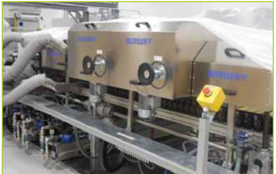
BENTELER WM4516C.01-2T0-11111-333 HORIZONTAL FLAT GLASS WASHING & DRYING SYSTEM [ YEAR 2011 ; ORDER#30-254 ; OVERALL SYSTEM FLOOR AREA FOOTPRINT 36'LX25W ; CLOSED-LOOP-SYSTEM ; SPEED 5 - 15 M/MIN FOR 0.7MM AND OVER 500X500MM PRODUCT ; 60°C HOT WATER AND DETERGENT CLEANING CAPABILITY TO REMOVE STAIN AND RESIDUE ; DI WATER INTERNAL RECYCLING CAPABILITY ; CLEAN TRANSITION INTO INSPECTION STATION], WITH EQUIPMENT: (IN FEED CONVEYOR) (QTY-48 DISK BRUSHES FOR DETERGENT WASH, WITH QTY-4 SIEMENS MOTORS ) (ROLLER BRUSHES AND SHOWER FOR DI WATER RINSE) (QTY-10 AIR KNIFE UNITS FOR DRYING) (BLOWER UNIT ON RAISED PLATFORM, OVERALL HEIGHT 15") (EXIT CONVEYOR) (INTERNAL TANKS: QTY-9 WASHING TANKS) (EXTERNAL SUPPORT: WATER POLISHING TANK SYSTEM ; FLOW VALVE ASSEMBLY RACK WITH G-MAR HEAT EXCHANGER ; H2O2 CLEANER SUPPLY TANK WITH METERING PUMP ; DETERGENT TANK WITH METERING PUMP) (REMOTE STATION: 3-SKID DI WATER FILTRATION & RECYCLING STATION WITH QTY-2 SS TANKS & QTY-2-TOTAL GRUNDFOS. TOTAL FOOTPRINT 15'LX3'W). WITH PLC CONTROL CABINET: (FOOTPRINT 14'LX7'H ; SIEMENS SEMATIC S7-300 PLC SYSTEM;SIEMENS SINAMICS A5E/6SL-SERIES DRIVES ;SIEMENS SIRIUS INDUSTRIAL CONTROLLERS ; ASSORTED RELAYS. ALSO INCLUDES QTY-1 SIEMENS TOUCH MULTI PANEL STATION)
