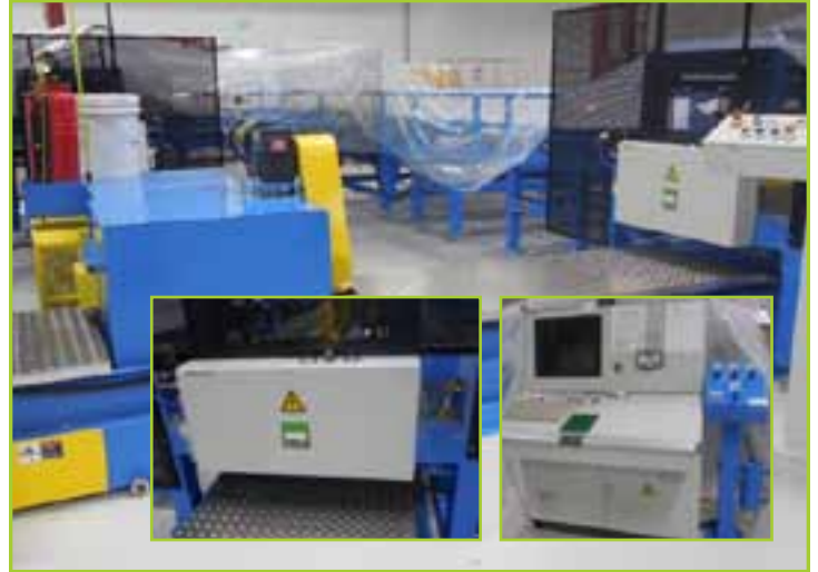
ENDURAVEYOR REJECT GLASS CULLET CRUSHER & CONVEYOR SYSTEM. [ QTY-2 IN FEED 29"W HINGED STEEL-BELT CONVEYOR TRACKS ; TRACKS APPROX. 17'L ] (GLASS CULLET CRUSHER APPARATUS 24" BELT WIDTH ; 1-HP MOTOR GEAR DRIVE AT 20'/MIN ; FOOTPRINT CRUSHER 6'LX2.5'WX2'H) (2.5 PITCH HINGED STEEL-BELT GLASS CULLET ELEVATOR CONVEYOR WITH END DISCHARGE CHUTE ; CONVEYOR 11'L ).
