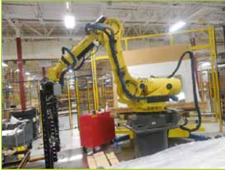
FANUC R-2000IB/210F INDUSTRIAL ROBOT (6-AXIS ; WRIST CAPACITY UP TO 210 KG ; REACH 2.60 M ; ON STAND 3'H), WITH R-30IA CONTROLLER AND I- PENDANT [ROBOT S/N-R11602213 ; CONTROLLER S/N-E11601111 ; SYS ID#F109939 ; SYS YEAR 2011]. WITH GLASS-SHEET-HANDLING URETHANE-CUPS END EFFECTOR TOOL (TOOL FOOTPRINT 5'LX4.5'W). ALSO INCLUDED: [CRATE PALLET-TURNTABLE (TURNTABLE PLC CONTROLLER NOT INCLUDED). PLATFORM FOOTPRINT 11'L TOTAL X 7'WX2'H, AND ATTACHED FENCING PANELS 12'H. WITH QTY-2 HEGLA BEIGE METAL CRATE HOLDER RACKS, 6.5'LX4.5'WX 6'H] [TROAX WIRE MESH FENCING WITH 3-DOORS. 75-LINEAR FEET @ 7'H ; 17-LINEAR FEET @ 12'H] [STAINLESS STEEL PANEL FLOOR COVER 12'LX10'W]
