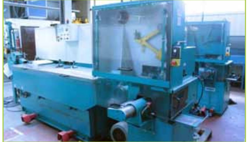
KIESELSTEIN WGTU100/25 & SM251 VARIABLE SPEED DRIVE (3-16 M/SEC). 25 DRAWING STEPS: 23 STEPS FOR 1,7 MM IN TO 0,3 MM OUT, 25 STEPS FOR 1,6 MM IN TO 0,26 MM OUT, 25 STEPS FOR 0,85 MM IN TO 0,14 MM OUT. MACHINE CURRENTLY SET FOR SS WIRE AT 1,2 MM IN TO 0,54 MM OUT. TOTAL RECORDED HOURS: 16,152 HR
