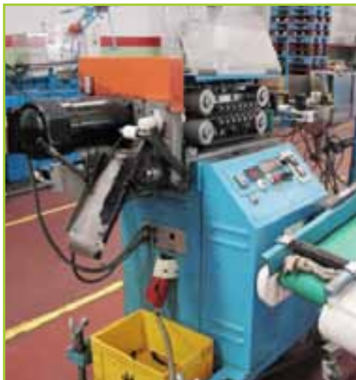
PICOMAT RAM 400 MOBILE BELT TYPE CABLE/TUBE TENSION CONVEYOR ROLLERS, WITH MOTORISED CUT MACHINE AND PHOTOELECTRIC DIAMETER MEASURING DEVICE
