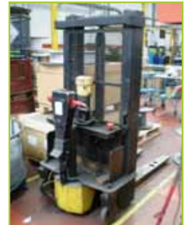
BATTERY ELECTRIC PEDESTRIAN FORK LIFT TRUCK WITH CHARGER
