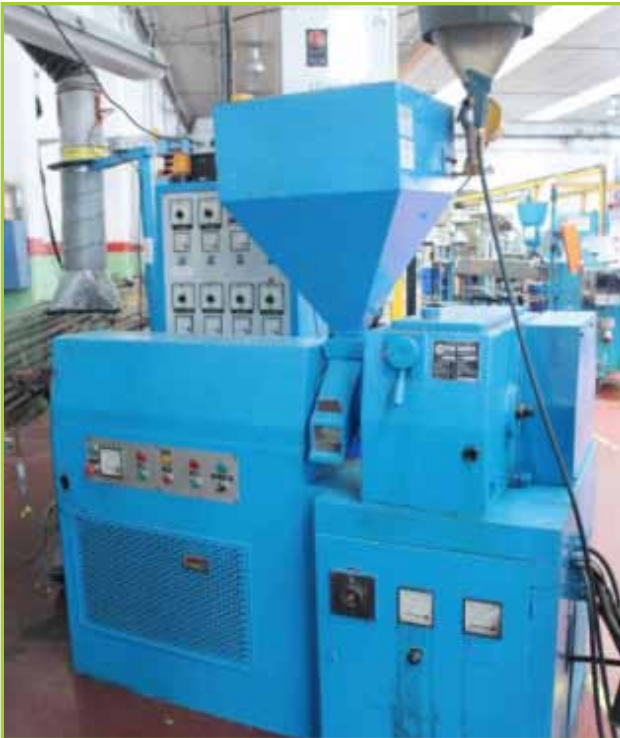
BANDERA PLASTIC TUBE EXTRUSION MACHINE. WITH HOPPER FEED, MATERIAL FEED REGULATOR AND CONTROL PANEL
