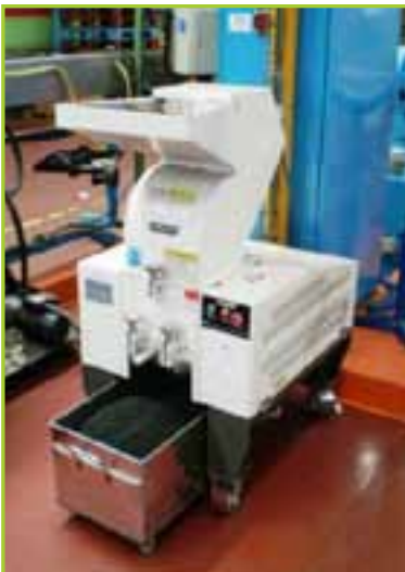
MING LEE ML SC5 111 MOBILE PLASTIC GRANULATING MACHINE 4KW/240X150MM FEED CHUTE & CONTROLS
