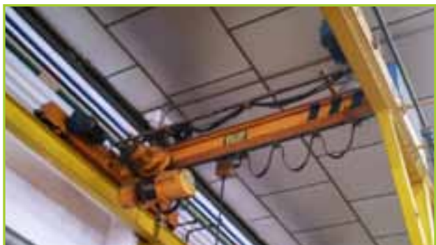
VILLOP 500KG SWL UNDERSLUNG OVER HEAD TRAVELLING CRANE
