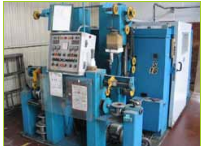
SKET MSDC 2/7X190 SECTION 1: 6+1 WIRES (CURRENTLY AT 1X0,18 + 6X0,165 FOR GALVANISED), 28,254 TOTAL RECORDED HOURS. SECTION 2: 6+1 WIRES (CURRENTLY AT 1X0,345 + 6X0,33 FOR SS), 27,573 TOTAL RECORDED HOURS. SPEED: 8000 RPM. WITH VARIABLE SPEED DRIVE. POWER: 65 KW. WEIGHT: 5785 KG. REF NO. 9. YEAR: 1998
