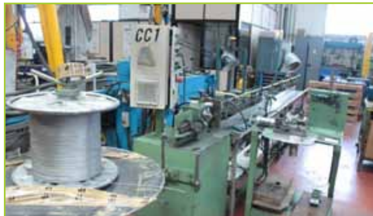
CUT TO LENGTH MACHINE CUTTING LENGTH: 4000 MM. WITH STRAIGHTENER
