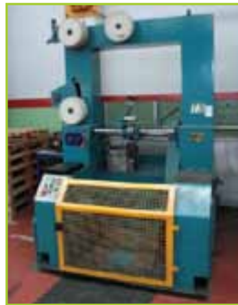
BMS BHSD 700 WIRE PULL: 20-50 KG. MAX WORKING SPEED: 3 M/S. WIRE RANGE: 1-4MM. WITH PNEUMATIC DISC BRAKE AND CONTROLS
