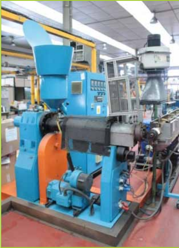
KUHNE K45-24D SCREW DIA: 48 MM. SCREW SPEED: 13-134 RPM. WITH FEED HOPPER, AND FEED AND CONTROL PANELS
