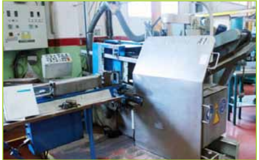
FRECH DAW 20 A SBC 20-TON HOT CHAMBER DIE CASTING MACHINE, WITH 240KN CLAMPING FORCE, 40KN INJECTION FORCE, 250MM X 250MM BETWEEN TIE BARS, 380MM X 380MM PLATEN, 180MM OPENING DISTANCE, SBC 3 CONTROLS, DISCHARGE CHUTE, RODANT MODEL OR-05 MOTORISED INCLINED STEEL BELT & SLAT FEEDER CONVEYOR 300MM WIDE ON BELT, FUME EXTRACTION FAN, FITTED WITH 12 SECTION CABLE DIE DIE AND 12 SECTION SIDE CABLE INSERTING ATTACHMENT
