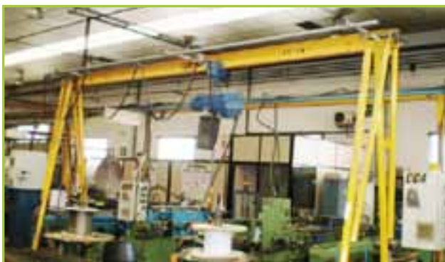
KOLI 500KG SWL A-FRAME LIFTING GANTRY 4MTR WIDE X 2.8MTR HIGH WITH KOLI 500KG SWL ELECTRIC CHAIN HOIST AND PENDANT CONTROL.
