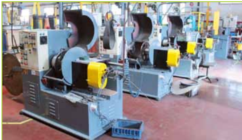
LUCKY WINSUN EAW-1 L ENDLESS AUTO WIRE WINDING MACHINE, WITH CONTROL PANEL, FEED REEL HOLDER, AND MOTORISED SWING ARM SPOOL CHANGE HOIST
