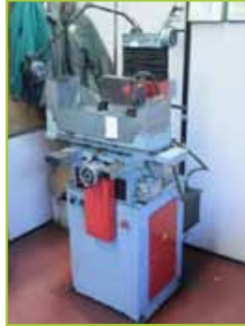
SAIM METAL 5100 2H MAGNETIC CHUCK: 300 X 150 MM. COOLANT PUMP, TANK AND CONTROLS
