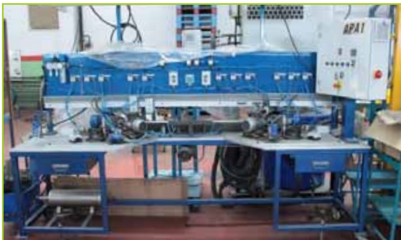
SPECIAL PURPOSE ELECTRO/PNEUMATIC 4-HEAD GRINDING AND DRILLING CABLE FINISHING RIG WITH PNEUMATIC CLAMPS, CONTROL PANEL AND ON ALLOY-TOP BENCH 2.8MTR X 0.65MTR.
