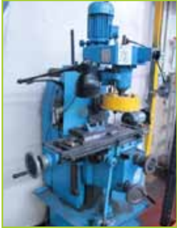
LAGUN F-900 VERTICAL MILLING/SURFACE GRINDING MACHINE. TABLE: 650X170 MM
