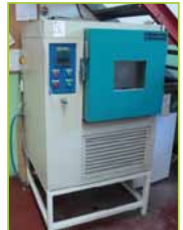
DYCOMETAL CCK SINGLE DOOR FAN ASSISTED CLIMATIC TEST CHAMBER, YEAR: 2009
