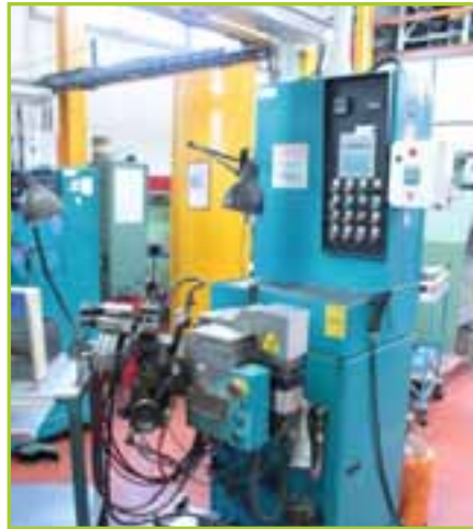
FISHERTECH AM46-K2CZ SEMI-AUTOMATIC HORIZONTAL CABLE INJECTED METAL ASSEMBLY DIE CASTING SYSTEM, MAX INJECTION CAPACITY WITH 3/4 INCH DIA INJECTION UNIT CAN INJECT 5CM 3 (0.3INCHES 3) OF ALLOY, WITH 1INCH DIA INJECTION UNIT CAN INJECT 8CM 3 (0.5INCHES 3) OF ALLOY, WITH ALLEN BRADLEY PANEL COMM CONTROLS AND FEED STAND
