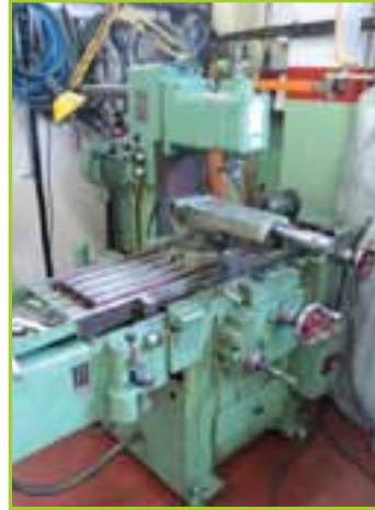
SOMUA Z1C VERTICAL MILLING MACHINE. TABLE: 1200X300 MM.
