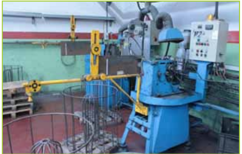
FLATTENING AND WINDING MACHINE, ROMERO CONTROLS UPDATED BETWEEN 2008-2009
