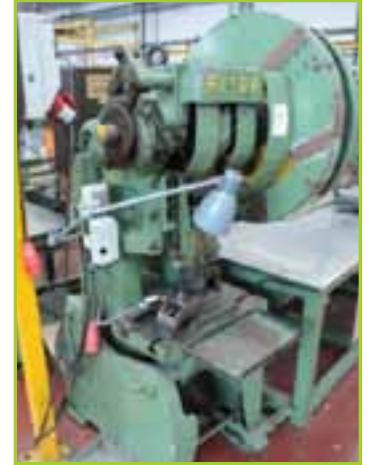
AITOR JMM 25 TON CAPACITY OPEN ENDED INCLINABLE POWER PRESS
