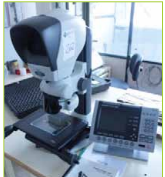
VISION KESTREL MONO DYNASCOPE 2-AXIS NON-CONTACT MEASURING SYSTEM WITH DYNASCOPE, STAGE GLASS, WITH METRONICS QUADRA-CHEK 200 CONTROL. REF NO. 262. YEAR: 2004
