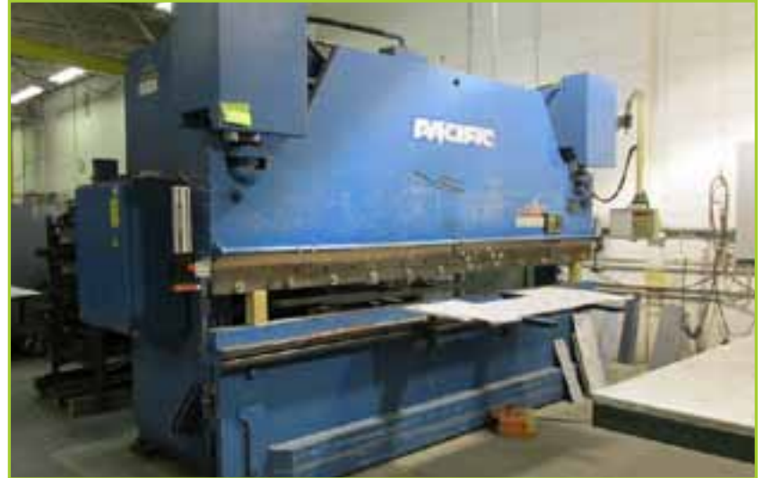
PACIFIC J230-12 CNC HYDRAULIC PRESS BRAKE ,AUTOMEC CNC 99 CONTROLS, MAX CAP 5/16". MS.PL.X10'-0"-.LG.
