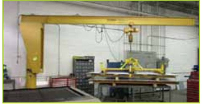
GORBEL 1/2-TON FREE STANDING 1/2-TON JIB CRANE, W/ HARRINGTON 1/2-TON CHAIN HOIST
