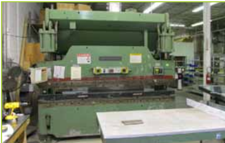
CINCINNATI 135CB X 8' CNC HYDRAULIC PRESS BRAKE AUTOMEC CNC 99 CONTROLS, 8" STROKE, 135-TON
