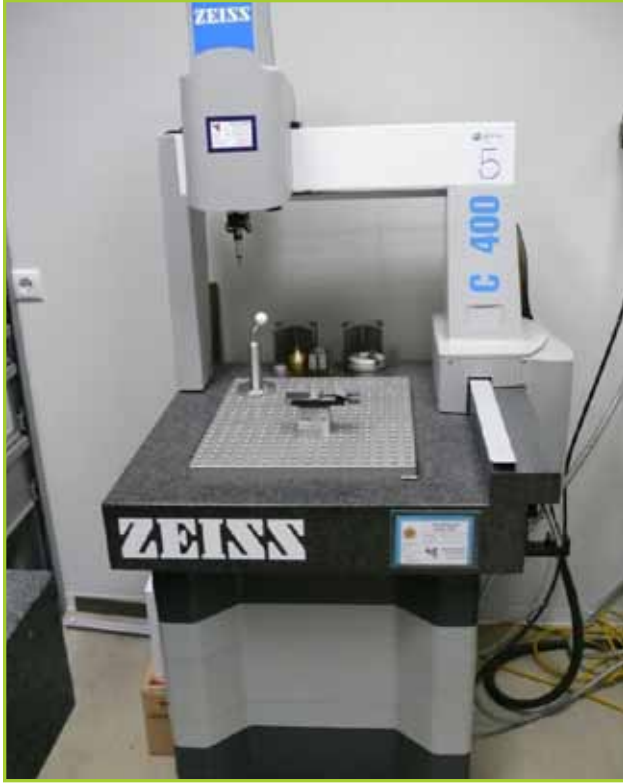
ZEISS C400 TABLE SIZE: 700X800 MM. WITH ZEISS C90HP CONTROLLER, UNBRANDED TOWER COMPUTER, DELL FLAT SCREEN MONITOR, KEYBOARD AND MOUSE. S/N 950702672 .YEAR: 1995
