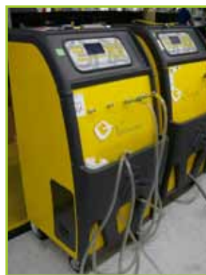
GALILEO PO 028/4 REFRIGERANT VACUUM PUMP AND CHARGER UNIT. YEAR: 2011
