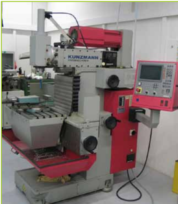
KUNZMANN WF478 X AXIS TRAVEL 400MM, Y AXIS TRAVEL 320MM AND Z AXIS TRAVEL 400MM. HEIDENHAIN CONTROL. WITH HAHNE & KOLB 6-INCH MACHINE VICE. S/N 344069 .YEAR: 2002
