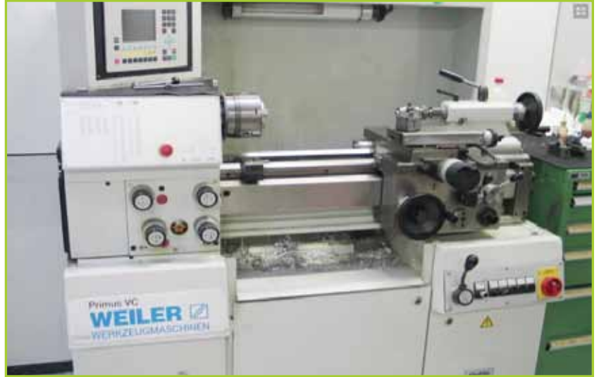
WEILER PRIMUS VC 500MM BETWEEN CENTRES, 280MM SWING OVER BED, FITTED 3 JAW CHUCK, QUICK CHANGE TOOLPOST WITH 3 AXIS SIEMENS SICOMP IMC05 CONTROL. S/N 141 .YEAR: 1999.
