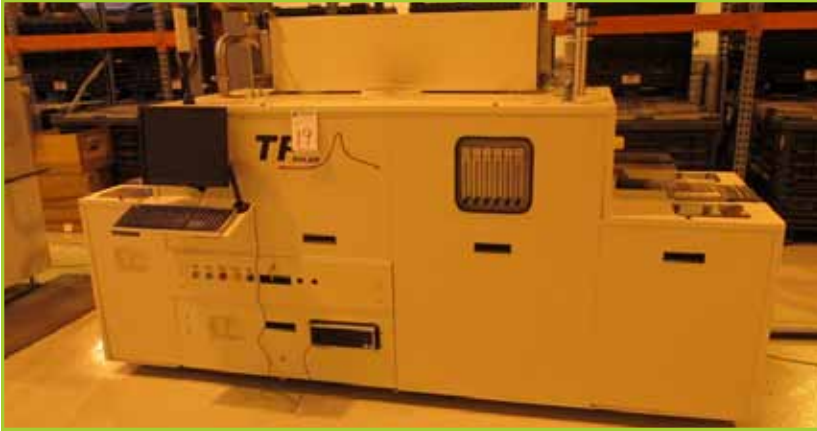
TP SOLAR D-225 INFRARED FURNACE , 480V 3 WIRE/NEUTRAL/GROUND, 50/60 HZ, 40 KW, 75 PSI, PROCESS EXHAUST 350 SCFH, CABINET EXHAUST 500 SCFH, 10" X 110" WIRE CONVEYOR, W/TP SOLAR VOC CONDENSER . SN# 2011190. YEAR: 2010
