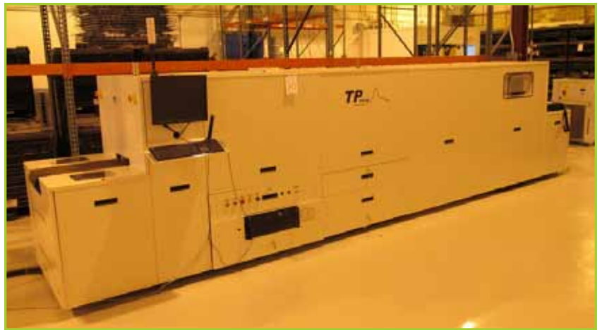
TP SOLAR D-225L INFRARED FURNACE , 480V 3 WIRE/NEUTRAL/GROUND, 50/60 HZ, 85 KW, 101 AMPS, 75 PSI, 19 LPM@ 4 BAR, 1500 SCFH, PROCESS EXHAUST 350 SCFH, CABINET EXHAUST 500 SCFH, 10" X 238" WIRE CONVEYOR. SN# 2011189. YEAR: 2010
