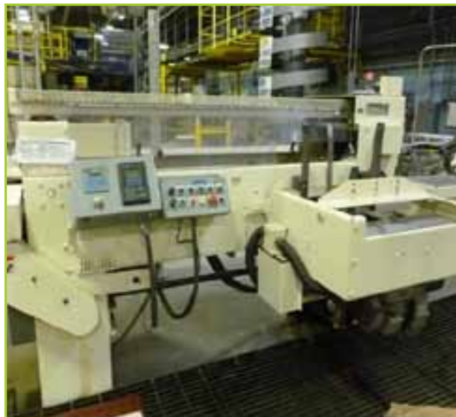
KAYAT TRAY LOADER, MODEL: TP70RFI, WITH NORDSON PROBLUE 10
