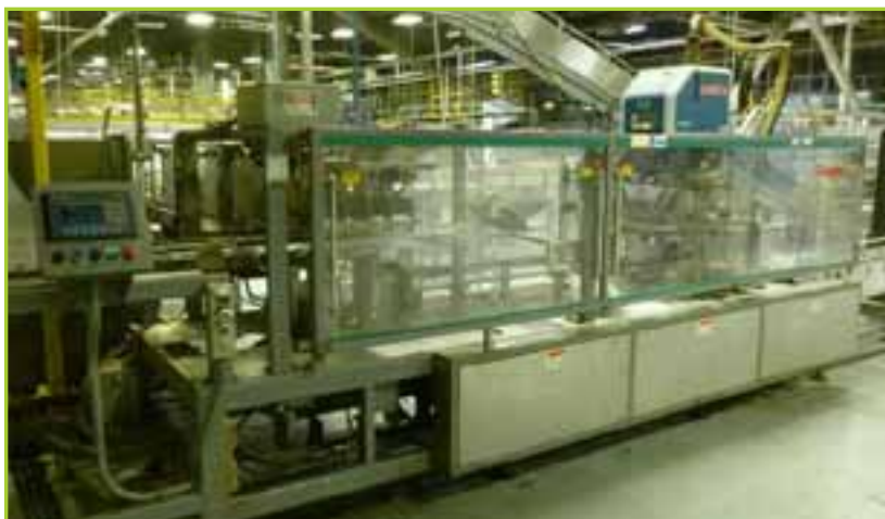
KAYAT PTF-28 CASE PACKER WITH NORDSON DURABLU 16 GLUER, ALLEN-BRADLEY 5/04 PLC CONTROLS
