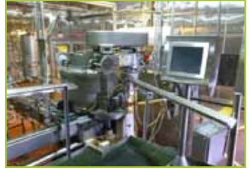
REBUILT 2007 - BEVCORP 72-VALVE CAN FILLER, REBUILT BY CCMC, WITH ANGELUS 120L CAN SEAMER, S/N: 7073368, WITH SETUP FOR 202 BEVERAGE CANS, UNDERCOVER GASSING FOR CO2 OR NITROGEN, CONTROL PANEL WITH ALLEN BRADLEY PROLOGIX PLC
