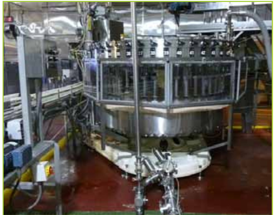
CROWN/BEVCORP 45-VALVE MONOBLOCK PET FILLER, WITH 2007 AROL 10-HEAD SCREW CAPPER, 28 & 38 MM FOGG CAP ELEVATOR/ HOPPER
