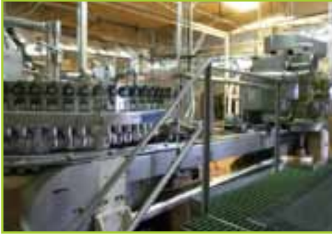
REBUILT 2007 - BEVCORP 72-VALVE CAN FILLER, REBUILT BY CCMC, WITH ANGELUS 120L CAN SEAMER, S/N: 7073368, WITH SETUP FOR 202 BEVERAGE CANS, UNDERCOVER GASSING FOR CO2 OR NITROGEN, CONTROL PANEL WITH ALLEN BRADLEY PROLOGIX PLC
