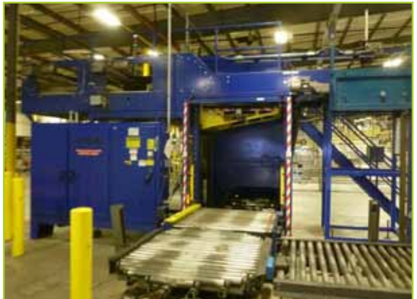
SENTRY BOTTLE DEPALLETIZER, MODEL: 7727, S/N: 1780, WITH ALLEN-BRADLEY CONTROLS, SLC 5/04 PLC, AND PANELVIEW 1000 HMI
