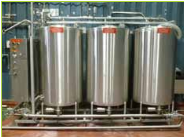
SANI-MATIC 3-TANK SKID MOUNTED CIP SYSTEM
