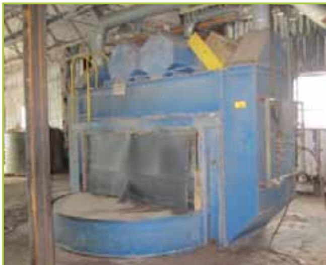
96" DIAMETER TABLE SAND BLAST MACHINE
