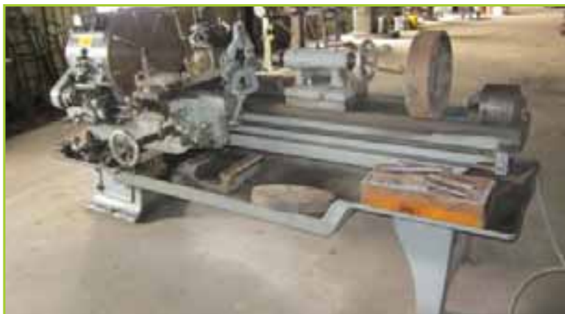
LATHE WITH 12" GAP, 20-670 RPM SPINDLE SPEEDS, 20" FACE PLATE, TOOL POST, TAPER ATTACHMENT, THREADING DIAL, TAIL STOCK
