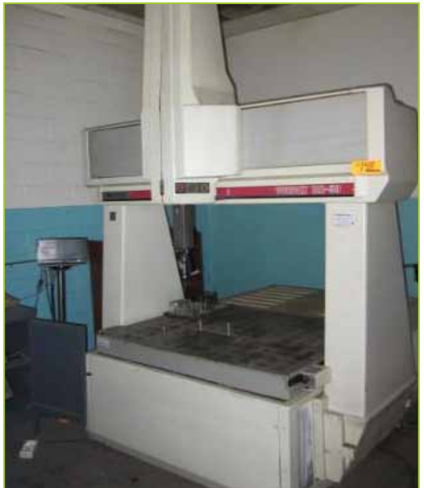
COORDINATE MEASURING MACHINE WITH 51"X43"X6" DRILLED & TAPPED WORK TABLE, TRAVELS: X-AXIS 60", Y-AXIS 54", Z-AXIS 7" SHEFFIELD MEASUREMENT PROCESSOR, 3-AXIS READOUT, HEWLETT PACKARD MDL. 86B CPU, MONITOR & KEYBOARD MODEL# RM-50
