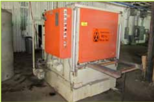
46"X40" OPENING HYDRAULIC DOOR, 7.5 HP PUMP, 100 GALLON TANK 45HP HYDRAULIC SYSTEM 91-425 MODEL# 1000
