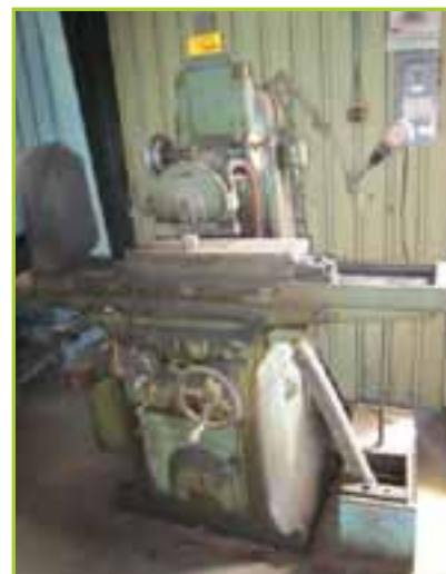
GRINDER MODEL# 3B WITH 8"X24" PERMANENT MAGNETIC CHUCK, COOLANT TANK, HYDRAULIC SYSTEM
