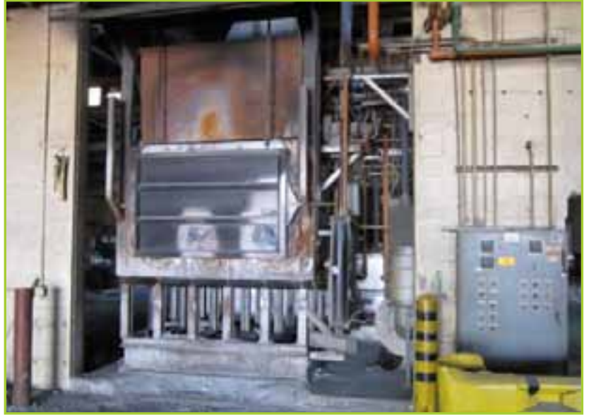
HEARTH ALUMINUM MELTING FURNACE WITH 15HP BLOWER (3) BURNERS,GAS SYSTEM AIR DOORS,WET PUMP SYSTEM,RATED AT 2000# PER HOUR
