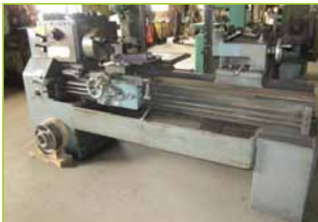
SOUTHBEND MDL.A ENGINE LATHE WITH 25-1000 RPM SPINDLE SPEEDS, 10" DIAMETER 3 JAW CHUCK, TOOL POST, CROSS SLIDE, TAPER ATTACHMENT, TAIL STOCK, 4 JAW CHUCK
