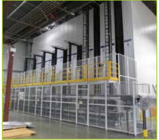
DAIFUKU/ESKAY 9Y-SRC-1 (7) MINI-LOAD F SERIES TWIN MAST AUTOMATIC STORAGE AND RETRIEVAL SYSTEM
