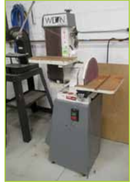
WILTON 4200 HEAVY DUTY BELT/DISK SANDER,6" BELT FINISHER, SPEED 2850 SFPM, TABLE TILTS 45° OUT AND 20° IN
