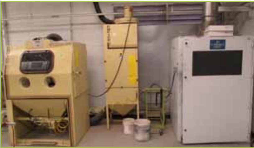
EMPIRE PF-3648 PRO FINISH SAND BLAST CABINET, WITH DUST COLLECTOR DCM-80A, 48 X 48 72" PAINTING CABINET
