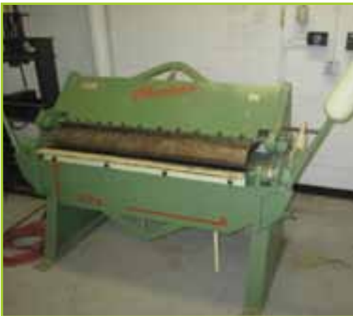
CHICAGO BPU 412-6 BENDING LENGTH: 4', CAPACITY: 12 GAUGE MILD STEEL (.105"), 10 GAUGE SOFT ALUMINUM (.135"), 16 GAUGE
