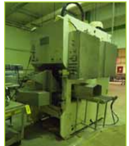
PEARSE EQUIPMENT BLOCK PRESS MODEL: BSP-55-3 WITH DIES AND INFEED CONVEYOR
