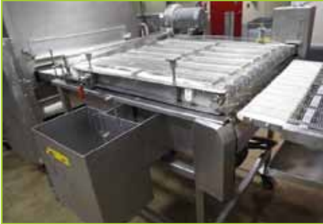
STAINLESS BREADING MACHINE WITH RECKER ELECTRONIC 38 IN. X 7 FT. ELECTRIC MOTOR
