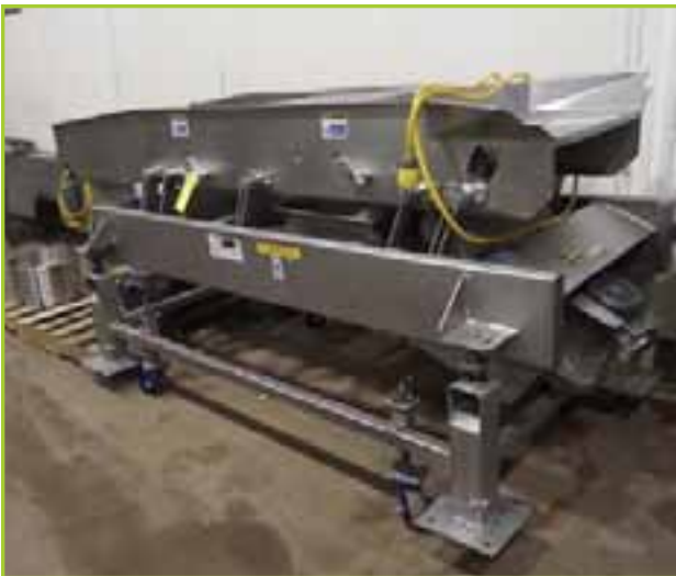
KEY ISO FLO VIBRATORY CONVEYOR ON CASTERS, ELECTRIC MOTOR
