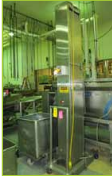
MTC BUCKET LIFT DUMPER MODEL H-LC-01 , 400 LB
