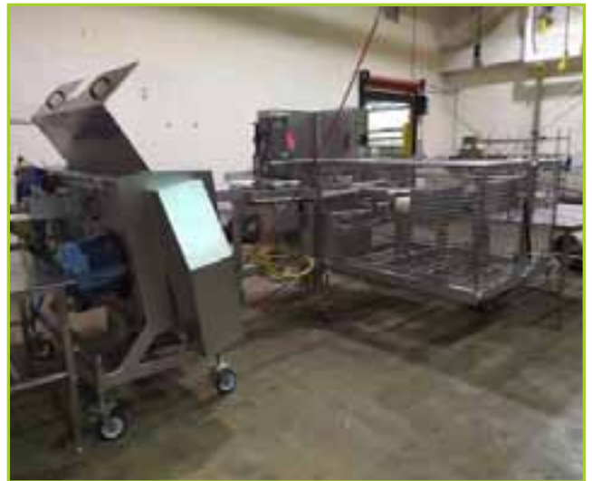
NORFLO LOG CUTTER WITH AUTO FEED SYSTEM TO AUTO SAW/MITER SAW CUTTING STATION WITH 6 BLADES, TYPE 797.45.201, NO. 45.144.ABB MOTOR WITH DRIVE DRUMS
