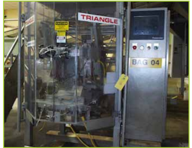
TRIANGLE BAGGER MODEL B3PFT4 , 08 VOLTS, 36 AMPS, SINGLE PHASE, 60 HERTZ, ADVANTAGE T-ZIP
