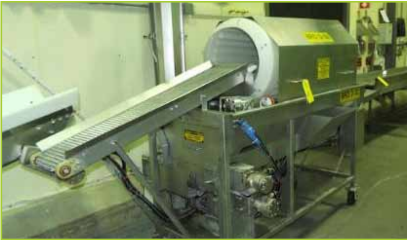
ROTARY COATING DRUM WITH APPLICATOR FEEDER , 23 IN. DIA. X 53 FT. LONG, DRUM INFEED AND OUTFEED CONVEYOR, ON CASTERS & HYDRAULIC MOTORS
