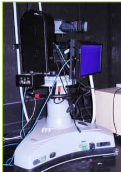
(4) VINTEN 14 ROBOTIC STUDIO SYSTEM: VINTEN HS-2010, SONY BVP-E30WS, SONY CA-570, SONY BVF-55, FUJI A18X7.6 BDERM-M48, EPD-2CA, FUJI ERD ZOOM CONTROL, QTV 15" TELEPROMPTER, VINTEN TRIPOD W/DOLLY, VINTEN AM-CSI-200, VINTEN AM-ACS-DJP, SONY RM-B150, SONY CCU-550D
