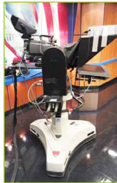
(4) VINTEN 14 ROBOTIC STUDIO SYSTEM: VINTEN HS-2010, SONY BVP-E30WS, SONY CA-570, SONY BVF-55, FUJI A18X7.6 BDERM-M48, EPD-2CA, FUJI ERD ZOOM CONTROL, QTV 15" TELEPROMPTER, VINTEN TRIPOD W/DOLLY, VINTEN AM-CSI-200, VINTEN AM-ACS-DJP, SONY RM-B150, SONY CCU-550D
