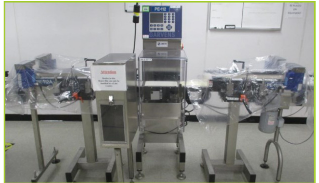
GARVENS E3 CHECKWEIGHTER WITH AUTO REJECTER WITH INFEEED SIDE TRANSFER BELTS FOR STABLE TRANSFER OF BOTTLES OR TALL UNSTABLE PRODUCT, SIDE BELTS ARE 2 INCHES WIDE X 27 INCHES LONG, OUTFEED SIDE TRANSFER BELTS FOR STABLE TRANSFER FROM WEIGH BELT TO DOWNSTREAM SYSTEM, WEIGHS PRODUCT UP TO 300 GRAMS
