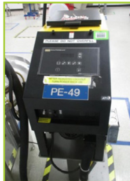
AUTOMATE AM-250 AUTOMATIC AIR-COOLED INDUCTION FOIL CAP SEALER , CAN RUN UP TO APPROXIMATELY 100 BOTTLES PER MINUTE
