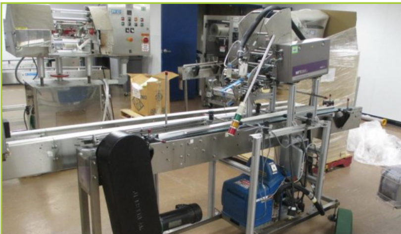
MFT 250IP FRICTION FEEDER , MINIMUM PRODUCT SIZE 25MM(W) X 38MM(L), MAX PRODUCT WIDTH 200MM(W), MINIMUM PRODUCT THICKNESS 0.05MM, MAX PRODUCT THICKNESS 25MM, MAX BELT SPEED 200,000 MM/MIN [656 FEET/MIN] WITH CONVEYOR AND NORDSON PROBLUE 4 ADHESIVE MELTER
