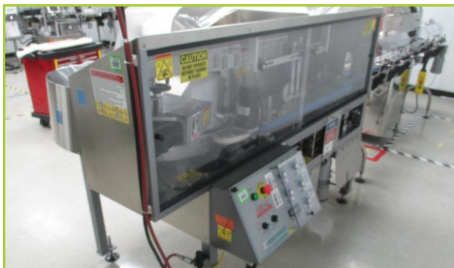
KAPS-ALL AU-3C STAINLESS STEEL AUTOMATIC BOTTLE UNSCRAMBLER , S/N 6391 WITH ELEVATOR/HOPPER ASSEMBLY, 30 CU FT HOPPER, 36" PRE-FEEDER BOWL, IONIZED AIR CLEANER WITH VACUUM, AND INTEGRATED CONTROL PANEL, 30CC TO 750CC BOTTLE CAP.
