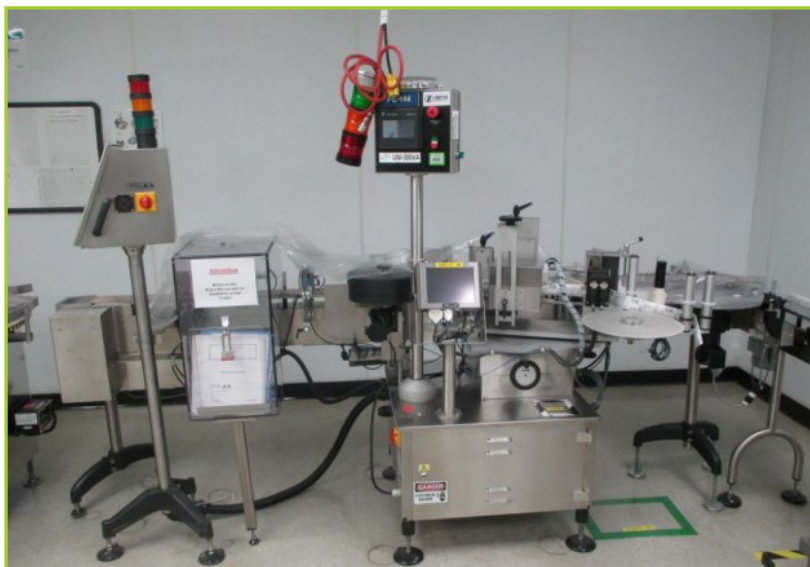
NJM/CLI UNI300VA-S023 ANALOG PRESSURE SENSITIVE PRINT/APPLY/INSPECT SYSTEM W/OPTEL VISION SYSTEM, VIDEOJET THERMAL TRANSFER AND UV DETECTOR, S/N 20120-1, RATED FOR 90 BOTTLES A MIN, (SETUP FOR ROUND BOTTLES ONLY)
