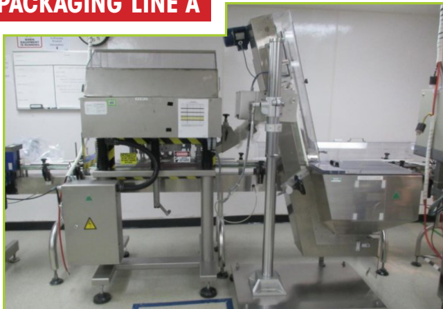
CVC CVC1204 STAINLESS STEEL 6 SPINDLE CAPPER , S/N 312454, WITH LARGE CAPACITY FLOOR LEVEL STAINLESS STEEL CAP HOPPER AND APPROX. 79" H CAP CONVEYOR FEEDER. CAN ACCOMMODATE BOTH ROUND AND IRREGULAR BOTTLES AND CONTAINERS WITH HEIGHTS BETWEEN 60 AND 250 MM, AND DIAMETERS BETWEEN 22 AND 120 MM, AND CAP DIAMETER: 22 TO 66 MM. SPEEDS TO 120 BOTTLES/MIN
