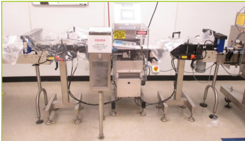
METTLER-TOLEDO XE3 HIGH SPEED CHECKWEIGHER , CHECK WEIGHING RANGE UP TO 6000G, THROUGHPUT (PCS./MINUTE) MAX. 200 WITH AUTO REJECT
