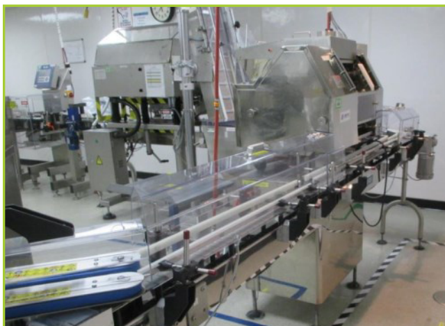
KING SC4 AUTOMATED SLAT COUNTER/FILLER , S/N 202803, WITH CONTROL PANEL, STAINLESS STEEL, RATED UP TO 60 BOTTLE/MINUTE OF A 100 COUNT FILL, SLAT COMES WITH A 133" L X 4" W BELT CONVEYOR
