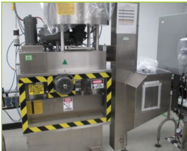
KAPS-ALL E4 PORTABLE SPINDLE CAPPER . MACHINE HAS 4-ROTARY SPINDLES FOR SPEEDS UP TO 80 CONTAINERS PER MINUTE (DEPENDING ON CONTAINER AND CAP SIZE). HAS A SIZE RANGE VARYING FROM VIALS UP TO 2-1/2 GALLON CONTAINERS. HAND CRANK SIZE ADJUSTMENTS. TOP-MOUNTED SORTING BOWL, S/N 4337 WITH VERTICAL CAP FEEDER CONVEYOR AND TOP-MOUNTED SORTING BOWL
