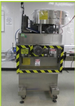
KAPS-ALL E4 PORTABLE SPINDLE CAPPER . MACHINE HAS 4-ROTARY SPINDLES FOR SPEEDS UP TO 80 CONTAINERS PER MINUTE
