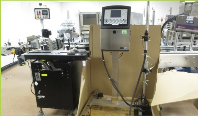
VIDEOJET 1520 CONTINUOUS INK JET PRINTER (NEVER USED) , MAX LINES OF PRINT 5, MAX LINE SPEED 279 M/MIN (914 FT./MIN) S/N 1230678C22ZH WITH 37" L X 2-1/2" W CONTROL PRINT CONVEYOR SIDE BELT TRANSFER MODEL M400TRANS, S/N 209495. RATED 50 TO 250 CONTAINERS PER MINUTE, 1" TO 7"
