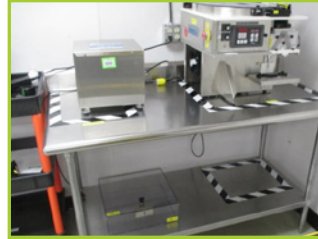
KING SC4 AUTOMATED SLAT COUNTER/FILLER , S/N 202801, WITH CONTROL PANEL, STAINLESS STEEL, RATED UP TO 60 BOTTLE/MINUTE OF A 100 COUNT FILL, SLAT COMES WITH A 133"L X 4"W BELT CONVEYOR
