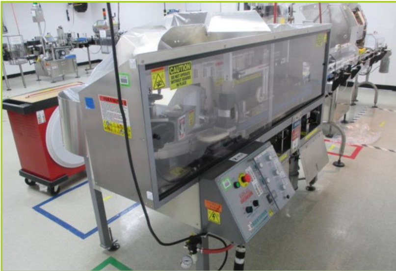
KAPS-ALL AU-3C STAINLESS STEEL AUTOMATIC BOTTLE UNSCRAMBLER , S/N 6392 WITH ELEVATOR/HOPPER ASSEMBLY, 30 CU FT HOPPER, 36" PRE-FEEDER BOWL, IONIZED AIR CLEANER WITH VACUUM, AND INTEGRATED CONTROL PANEL, 30CC TO 750CC BOTTLE CAPABILITY
