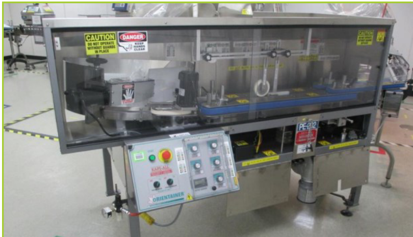
KAPS-ALL AU-3C STAINLESS STEEL AUTOMATIC BOTTLE UNSCRAMBLER , S/N 6730 WITH ELEVATOR/HOPPER ASSEMBLY, 30 CU FT HOPPER, 36" PRE-FEEDER BOWL, IONIZED AIR CLEANER WITH VACUUM, AND INTEGRATED CONTROL PANEL, 30CC TO 750CC BOTTLE CAP
