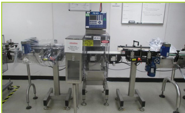
GARVENS E3 CHECKWEIGHER , S/N 332739 WITH INFEEED SIDE TRANSFER BELTS FOR STABLE TRANSFER OF BOTTLES OR TALL UNSTABLE PRODUCT, SIDE BELTS ARE 2 INCHES WIDE X 27 INCHES LONG, OUTFEED SIDE TRANSFER BELTS FOR STABLE TRANSFER FROM WEIGH BELT TO DOWNSTREAM SYSTEM, WEIGHS PRODUCT UP TO 300 GRAMS
