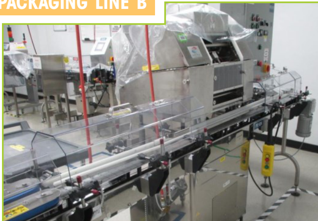
KING SC4 AUTOMATED SLAT COUNTER/FILLER , S/N 75, WITH CONTROL PANEL, STAINLESS STEEL, RATED UP TO 60 BOTTLE/MINUTE OF A 100 COUNT FILL, SLAT COMES WITH A 133" L X 4" W BELT CONVEYOR
