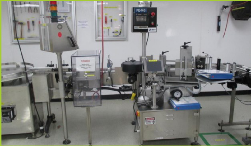
NJM/CLI UNI300VA PRESSURE SENSITIVE DIGITAL PRINT/APPLY/INSPECT SYSTEM W/OPTEL VISION SYSTEM, VIDEOJET THERMAL TRANSFER AND UV DETECTOR, S/N 23971-01, SETUP RATED FOR 90 BOTTLES A MIN
