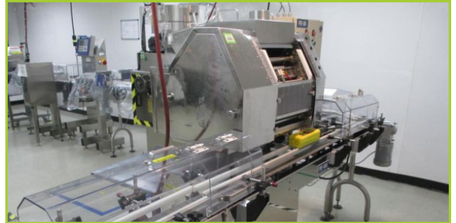
KING SC4 AUTOMATED SLAT COUNTER/FILLER , S/N 202801, WITH CONTROL PANEL, STAINLESS STEEL, RATED UP TO 60 BOTTLE/MINUTE OF A 100 COUNT FILL, SLAT COMES WITH A 133"L X 4"W BELT CONVEYOR
