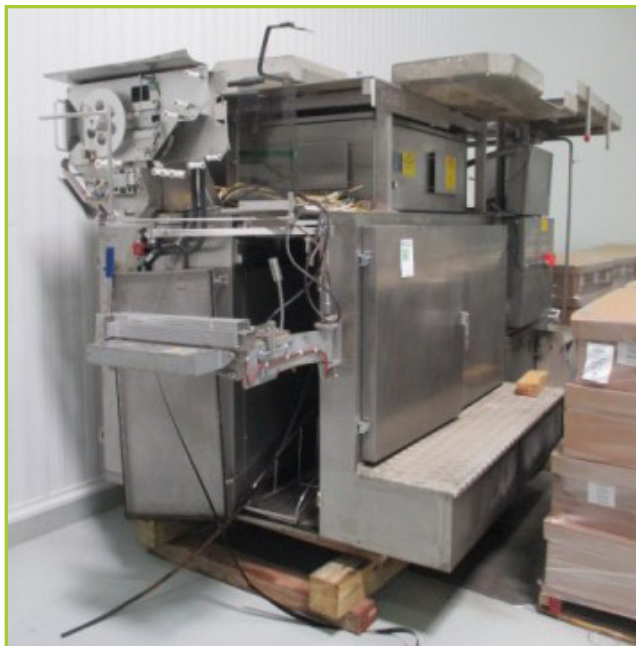
JAGENBURG 105-1U STRAIGHT LINE GLUER , LINE SPEED 1.300 BFPM, CARTON RANGE LENGTH 3" TO 48.25", CARTON RANGE WIDTH 2" TO 48.25". YEAR 1989
