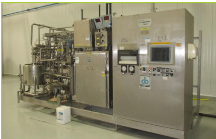
CHERRY-BURRELL 750 SKID-MOUNTED HTST ASEPTIC PASTEURIZER 25-GPM , WITH ALLEN BRADLEY CONTROLS (FOOTPRINT 22' LX 8' W). WITH ONLY SHELL & TUBE HEAT EXCHANGER.
