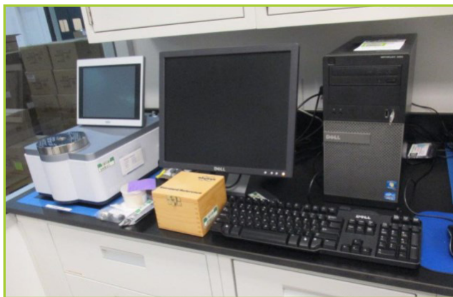
FOURIER TRANSFORM NEAR-INFRARED SPECTROMETER (S/N-200266 ; P/N-1014812/20). WITH ACCESSORIES: BRUKER STANDARD REFERENCE ; BRUKER SPARE LAMP ; BRUKER REFLECTIVE STAMP (LIQUIDS). WITH FT-NIR USB DONGLE KEY ; DELL OPTIPLEX-390 DESKTOP COMPUTER WITH HARD DISK DRIVE ; DELL 17" MONITOR.
