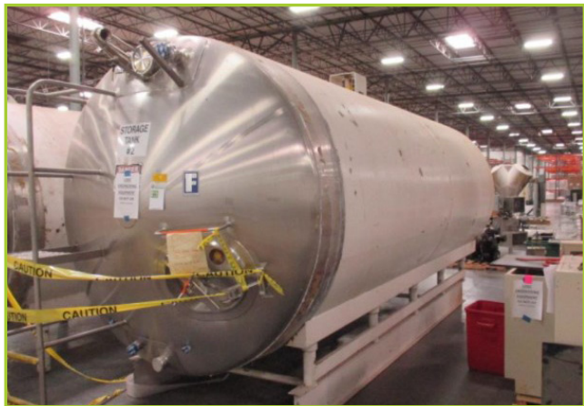
FELDMER A-865-0 5000-GALLON JACKETED TANK (HORIZONTAL ; ON I-BEAM SKID ; OVERALL FOOTPRINT 23.5'LX8'WX11'H ; TANK ID#2)
