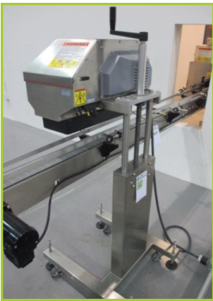
AUTO MATE AM-250 INDUCTION SEALER W/LARGE PROFILE HEAD
