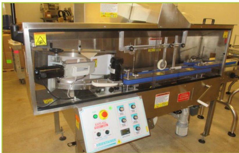
KAPS-ALL AU-3C/ORIENTAINER UNSCRAMBLER-CLEANER [NOTES: MAX 3" DIAMETER / MAX 6" TALL / MAX 300BPM]
