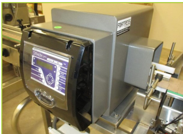
FORTRESS STEALTH METAL DETECTOR [NOTES: REJECT STATION]
