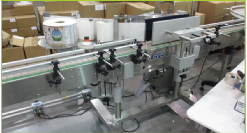
CVC CVC310C6 LABELER [NOTES: VACUUM WRAP STATION / MAX 160BPM]. WITH VIDEOJET DATAFLEX 6420 PRINT CODER [NOTES: PRINT ON LABEL]. WITH SLAT TOP CONVEYOR 6"WX1'1'L. WITH DOCUMENTATION
