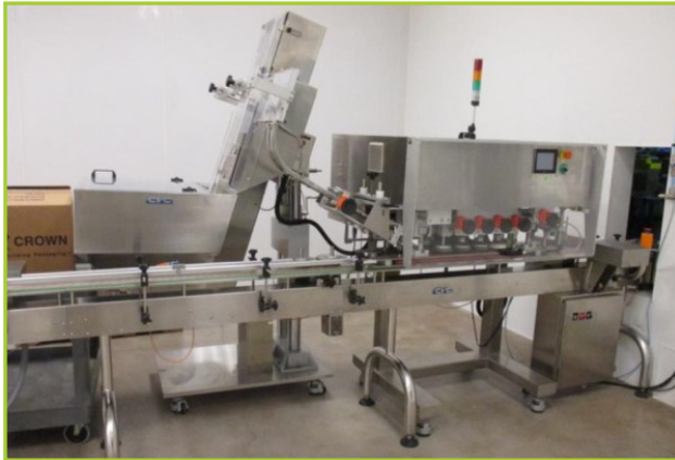
CVC CVC-1205 CAPPER. WITH CVC 1200W ELEVATOR FEEDER [NOTES: CAP TYPE: PLASTIC, METAL, OR CRC / CAP RANGE: 25MM - 77MM / BOTTLE HEIGHT: 2" - 8.5"; BOTTLE DIAMETER 1.25" - 4.5" / MAX 120BPM]. WITH SLAT TOP CONVEYOR SECTION (APPROX 4.5"W X 29'L).
