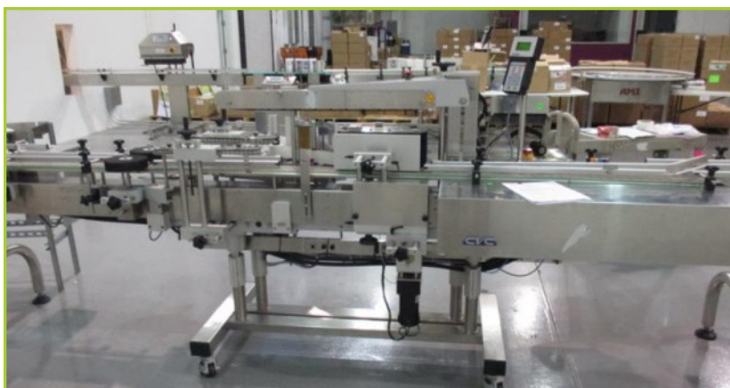
CVC CVC-430CS WRAP LABELER [NOTES: MAX 175BPM]. WITH VIDEOJET 8.4-CLARITY/DATAFLEX-6420 PRINT CODER [NOTES: CODE ON LABEL]. WITH SLAT TOP CONVEYOR SECTION (APPROX 4.25"W X 11'L).
