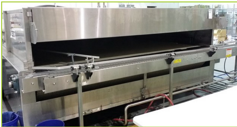
COOLING TUNNEL, CHILLED WATER ; 10'X25' INTERLOX TYPE BELT WITH CONTROLS AND HEAT EXCHANGER
