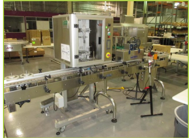
UNIQUSEAL TE-100 SHRINK NECK BANDS MACHINE [NOTES: BUTTERFLY FOR 38MM, 45MM, 53MM / MAX 80BPM]. WITH MARBURG GR-6000 SHRINK TUNNEL. WITH SLAT TOP CONVEYOR SECTION (APPROX 4.25"W X 19'L)
