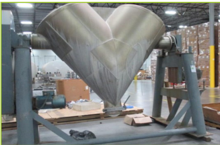
PATTERSON KELLEY 60-CUFT V-SHELL BLENDER, WITH CONTROL CABINE
