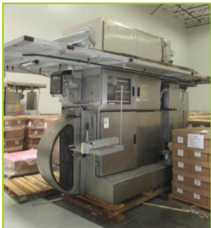
TETRA PAK TBA/19-250B ASEPTIC TETRA PAK BRIK FILLER LINE [BRIK FILLER ; STRAW APPLICATOR ; CARDBOARD PACKER ; TRAY CAPPER ; MARKEM CODERS]. BRIK FILLER S/N-20274-82734 YEAR-1996
