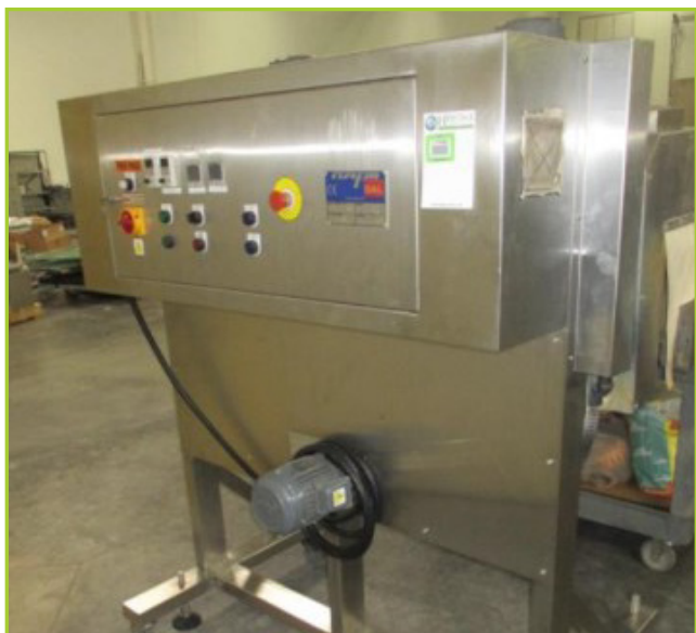
NAFM-OAL OES-200 RADIANT HEAT TUNNEL (FOOTPRINT 5'LX4'W)
