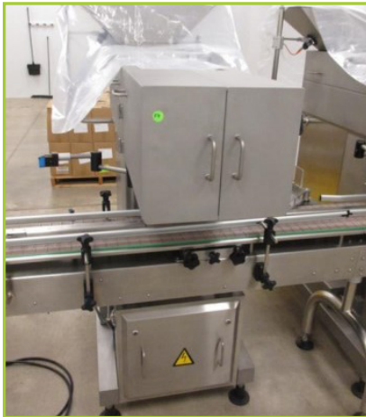
CVC CVC1220 CAPSULE COUNTER#1, YEAR-2013 [NOTES: MAX 55BPM ON A COUNT UP TO 100]. WITH CVC 1101 ELEVATOR FEEDER
