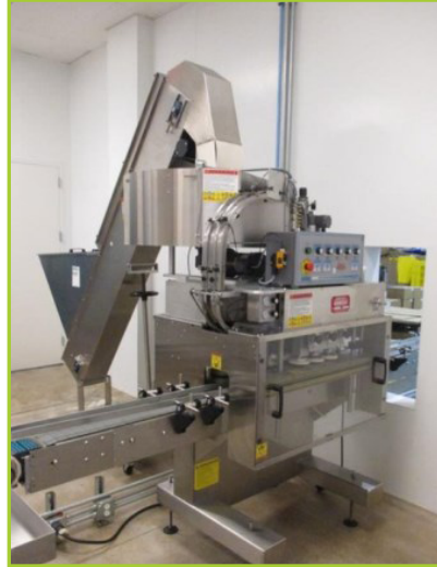
KAPS-ALL A6 LARGE PROFILE CAPPER [NOTES: 120MM MAX CLOSURE]. WITH KAPS-ALL FS-B CAPPER ELEVATOR FEED STATION S/N-7697-B. WITH SLAT TOP CONVEYOR SECTION 5.5"W X 16.5'L.
