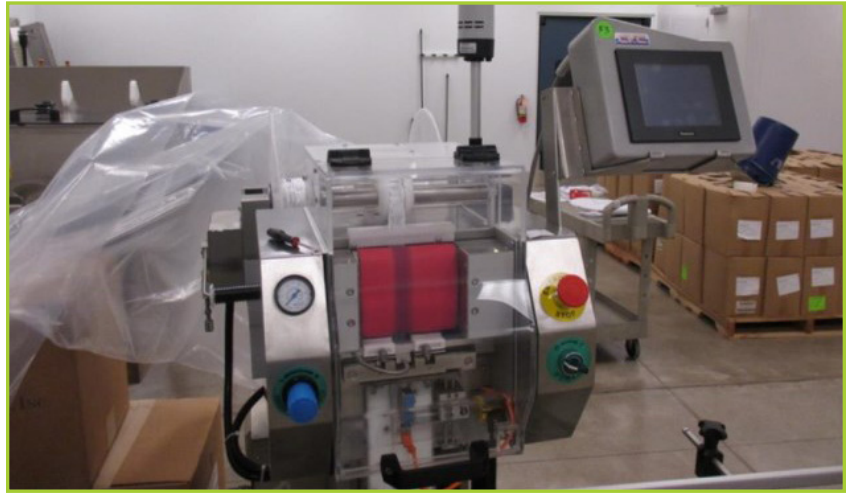
CVC CVC1103-R DESICCANT FEEDER, [NOTES: 1 GRAM DESICCANT @ MAX 120BPM]
