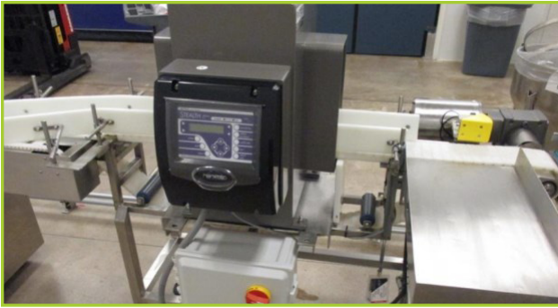
FORTRESS STEALTH METAL DETECTOR S/N-018399 [NOTES: 5"W X 11.5"H OPENING], WITH CONVEYOR 5.75"WX6'L. WITH DOCUMENTATION
