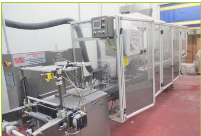
BARTELT / SOUTHERN PACKAGING POWER-POUCH-PLUS/IMF-7-14 HORIZONTAL FORM FILL SEAL MACHINE (FUNNEL POUCH MAKER/FILLER CONVEYOR), YEAR-1997
