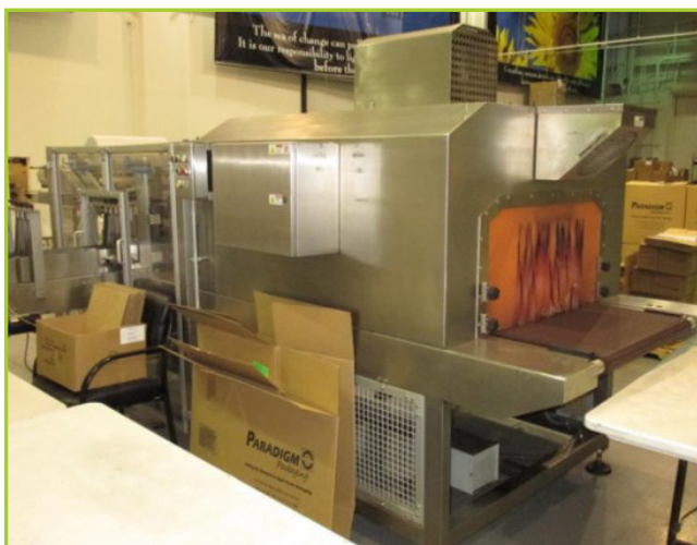
TEKKRA SYSTEMST-230-60 SHRINK BUNDLER SYSTEM [NOTES: 3-PACK 75CC BOTTLES / 12-PACK SQUARE DAIRY / 3-PACK 200CC]. WITH ALLEN BRADLEY PANELVIEW PLUS-400 CONTROL PANEL. WITH CONVEYOR BELT APPROX 28"WIDE
