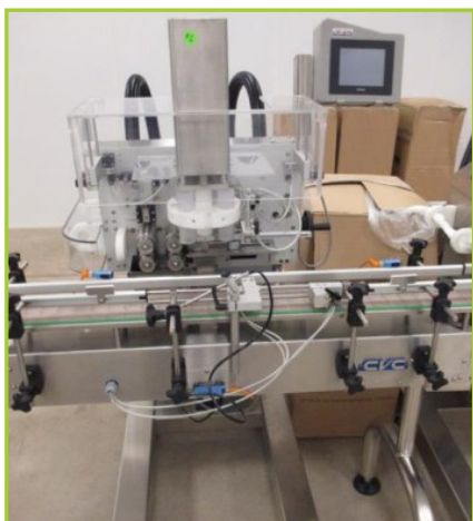
CVC CVC-1117 COTTON INSERTER#1 , [NOTES: MAX 60BPM WITH SINGLE INSERTION]
