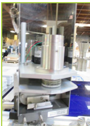
CAPSUGEL XCELODOSE 600 MICRO FILLING SYSTEM WITH POWER UNIT, XCELOTABLE AND SIZE CHANGE PARTS AND PRODUCT CHANGE PARTS
