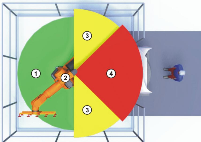
Fig. 3-3: Example of axis range A1
