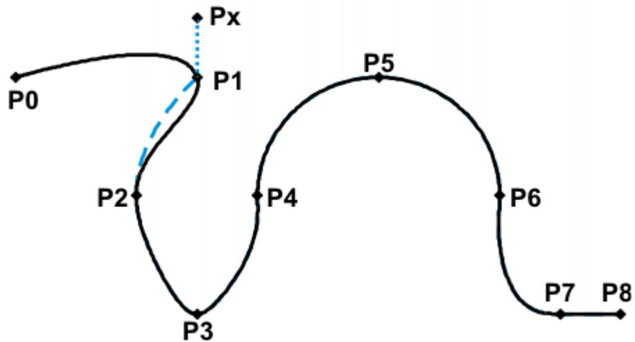
Fig. 7-8: Example: modified path in the case of block selection to P1
