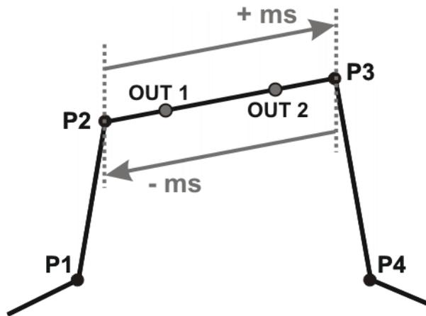
OUT 1 and OUT 2 specify approximate positions at which switching is to occur. The dotted lines indicate the switching limits.
