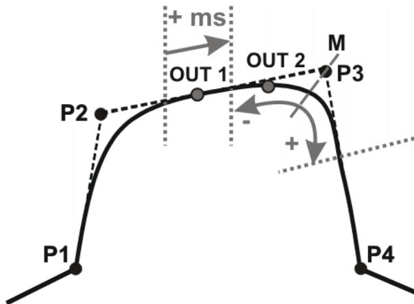
OUT 1 and OUT 2 specify approximate positions at which switching is to occur. The dotted lines indicate the switching limits. M = middle of the approximate positioning range.
