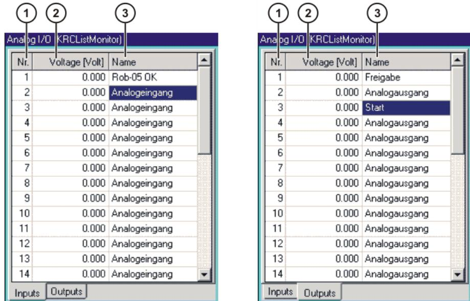
Fig. 4-26: Analog inputs/outputs
