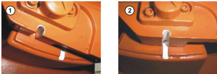
**Fig. 5-3: Moving an axis to the pre-mastering position**
