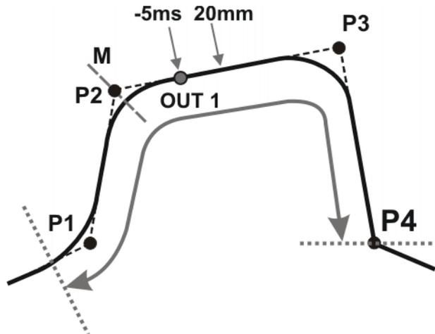
OUT 1 specifies the approximate position at which switching is to occur. The dotted lines indicate the switching limits. M = middle of the approximate positioning range.
