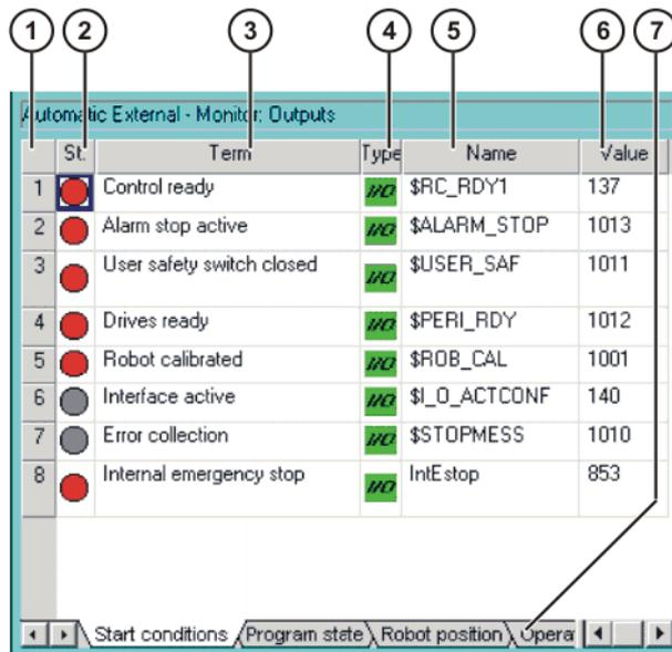
Fig. 4-28: Automatic External outputs (detail view)
