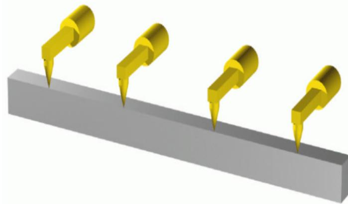
Fig. 7-17: Orientation control - Constant
