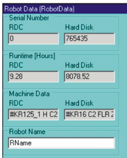
Fig. 4-30: Robot data – data on RDC and hard drive are not identical
