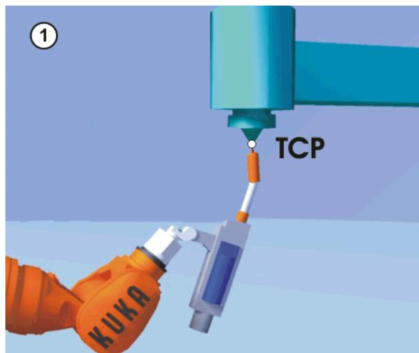
Fig. 5-13: Moving to the external TCP
