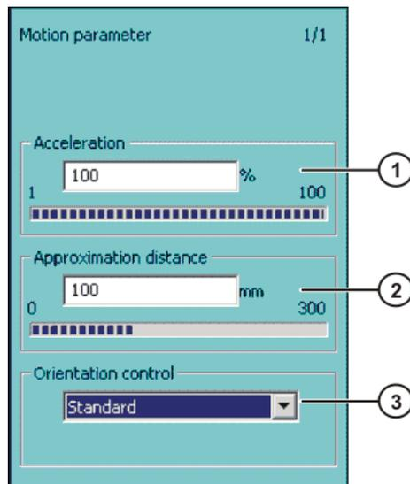
Fig. 8-6: Option window "Motion parameter" (CP motion)
