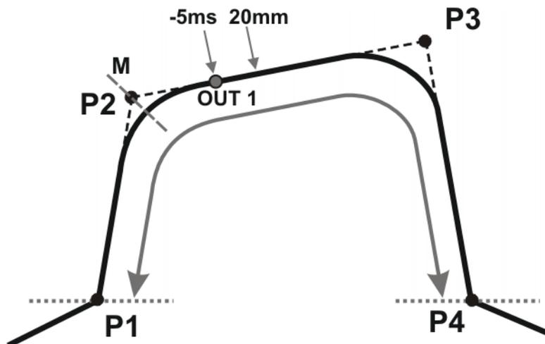
OUT 1 specifies the approximate position at which switching is to occur. The dotted lines indicate the switching limits. M = middle of the approximate positioning range.
