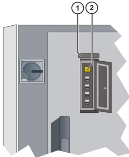
Fig. 4-5: KCP coupler LEDs and request button
