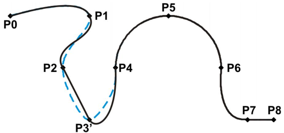
Fig. 7-11: Example 1: segment type changed
