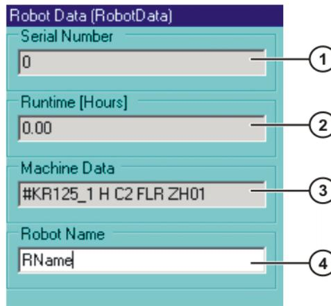
Fig. 4-29: Robot data – data on RDC and hard drive are identical
