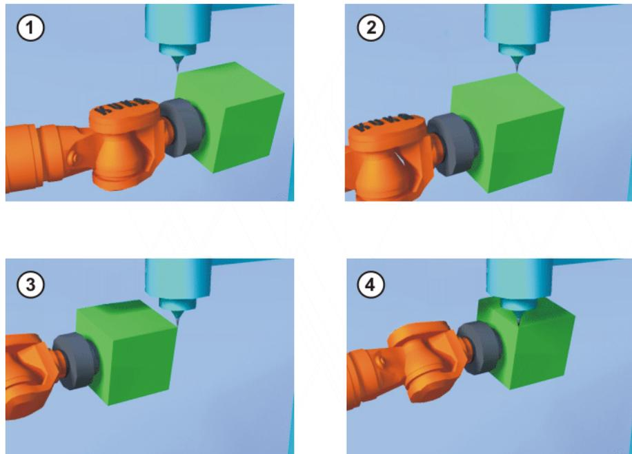
**Fig. 5-16: Workpiece calibration: indirect method**
