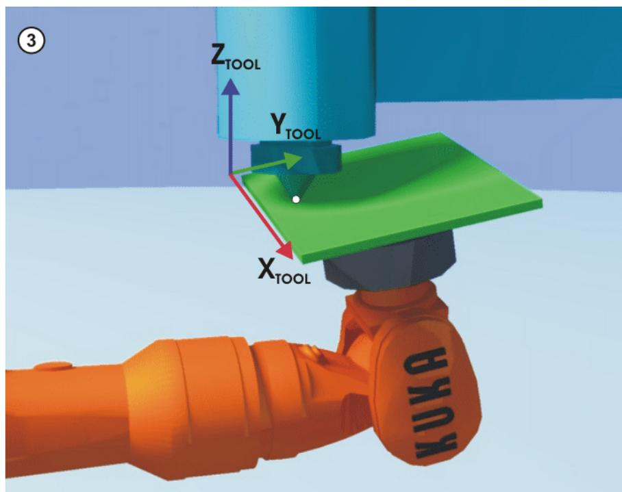
**Fig. 5-15: Workpiece calibration: direct method**
