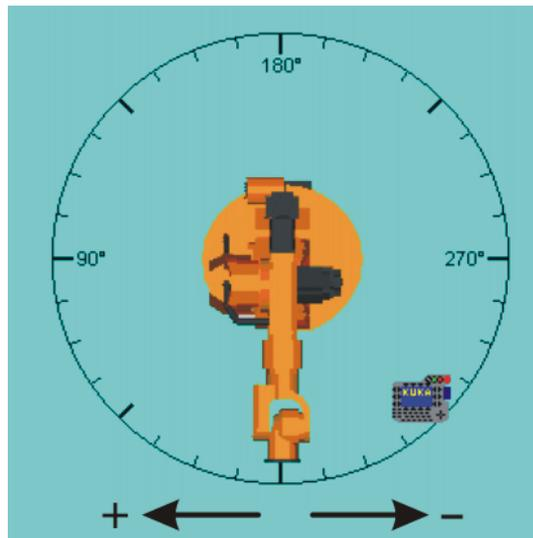
**Fig. 4-23: Option window for aligning the Space Mouse**
