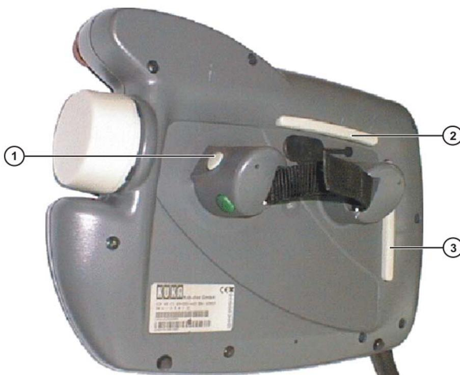
**Fig. 3-5: Enabling switches on the KCP**
