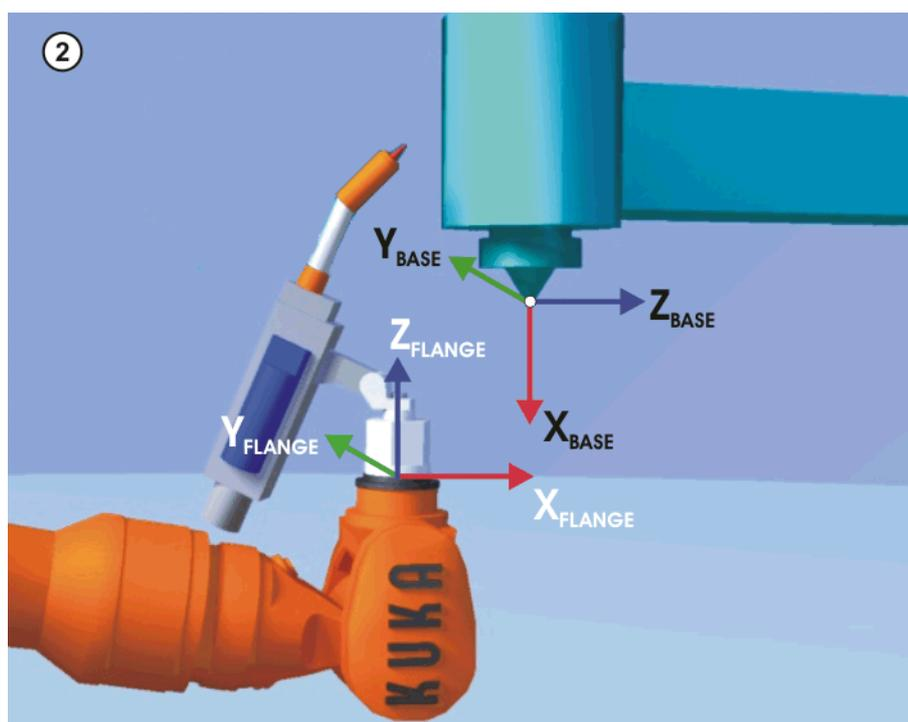
Fig. 5-14: Aligning the coordinate systems parallel to one another
