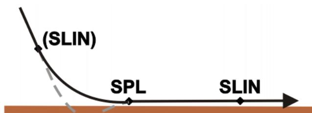
Fig. 8-8: Avoiding a collision with the work surface
