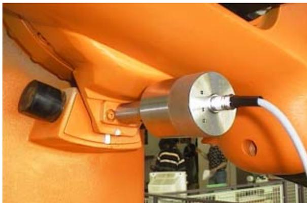
**Fig. 5-5: Electronic measuring tool**
