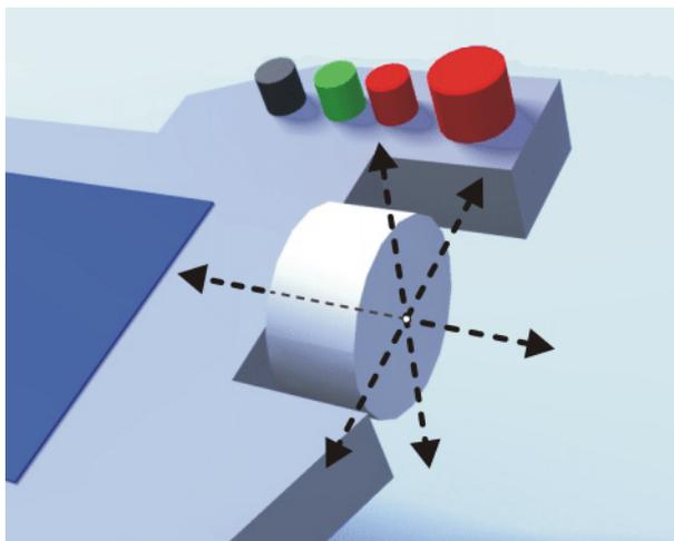
**Fig. 4-20: Pushing and pulling the Space Mouse**
