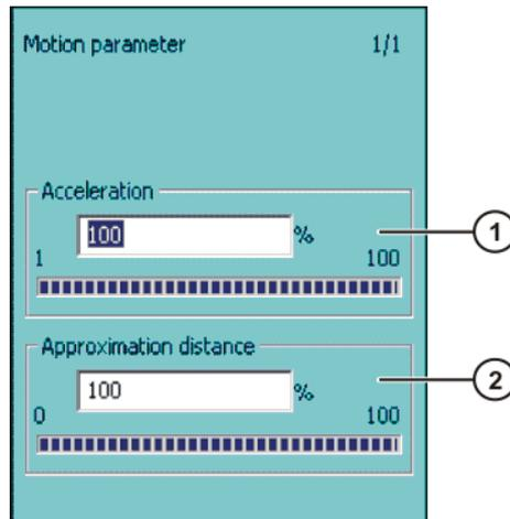
Fig. 8-5: Option window "Motion parameter" (PTP motion)
