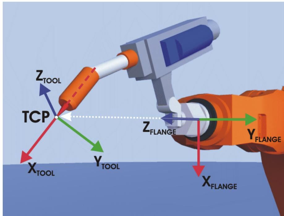
Fig. 5-8: TCP calibration principle
