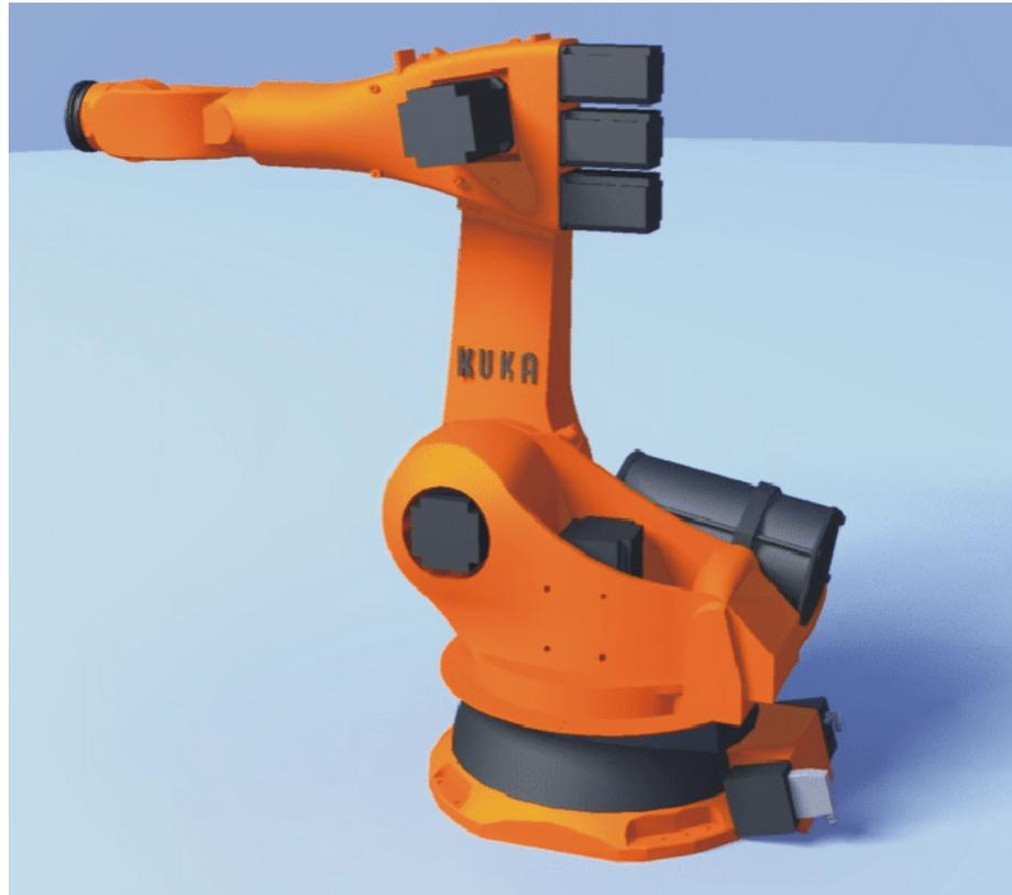
**Fig. 5-2: Mastering position – approximate position**
