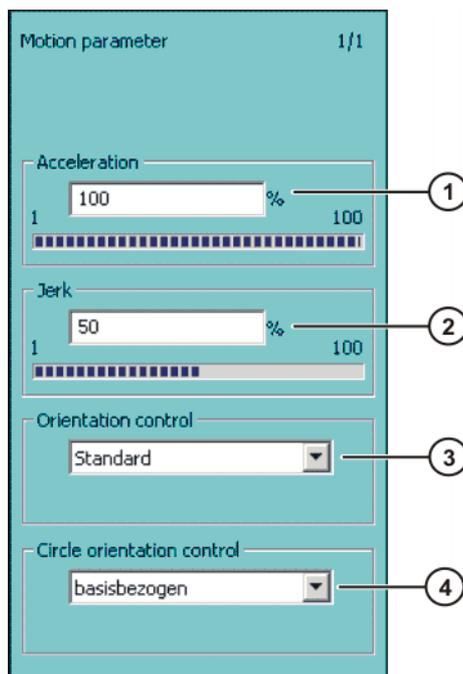
Fig. 8-10: Option window "Motion parameter" (spline motion)
