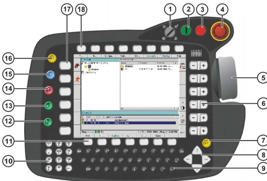
Fig. 4-1: Front view of KCP
