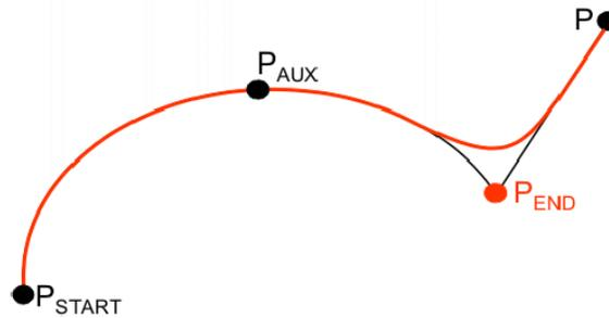
Fig. 7-16: CIRC motion,  $P_{END}$  is approximated
