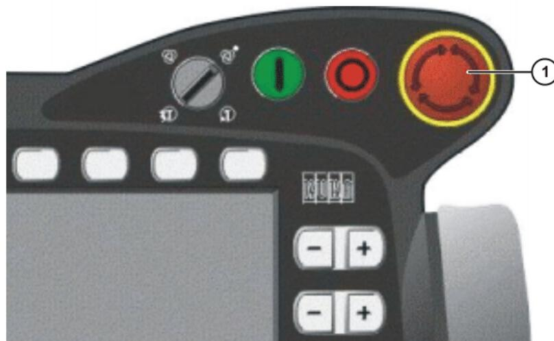
Fig. 3-4: EMERGENCY STOP button on the KCP
