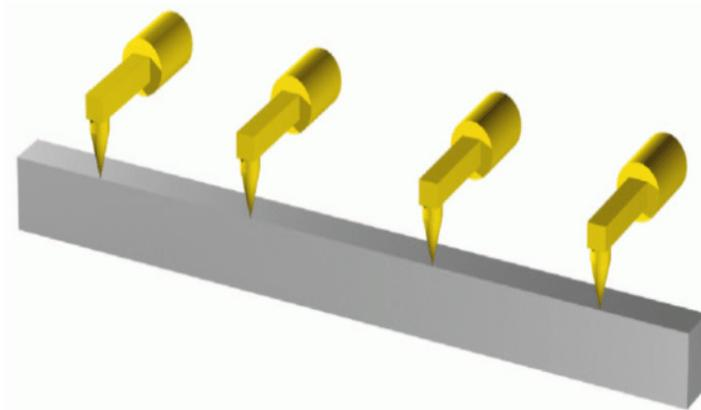
Fig. 7-19: Orientation control - Constant
