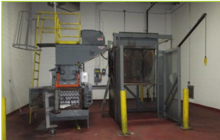
HARMONY SSBH-R BOTTLE-CAN CRUSHER & BAILER WITH TOTE LIFT/DUMPER, S/N-SSHB-R-0028. OVERALL FOOTPRINT 16'L X 15'W X 13'H ; WITH ALLEN BRADLEY C1000 PANELVIEW MONITOR/CONTROL ; METER AT 06120-HRS
