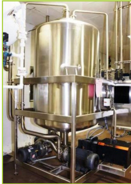
BEVCORP LLC MICRO BLEND VACUUM DEAERATOR WITH SINGLE VFD. WITH MICRO BLEND INTERFACE POWER DISTRIBUTION
