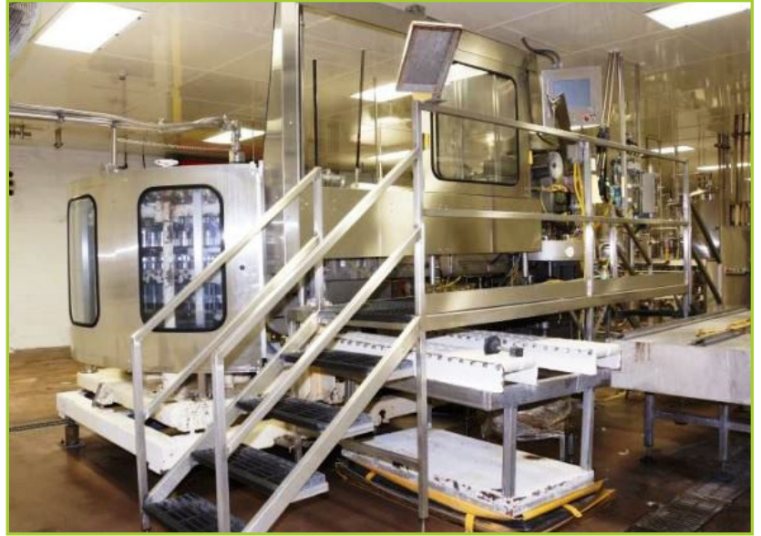
CROWN UB72-FTCF 72-VALVE CAN FILLER. 1280 CANS PER MIN. INCLUDES LUB SYSTEM, UNDER CONVEYOR, INFEED CAN DRYER BLOWER. S/N-GF 72FTCUB11
