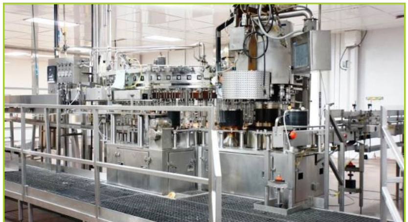
H&K DELTA 600-66-11 66-VALVE FILLER WITH 11-HEAD CAPPER. NEW MAIN BUSHING ON MAIN SPINDLE, NEW GEAR BOX. FILLER NEW BULL GEAR. S/N-VF66-84-71
