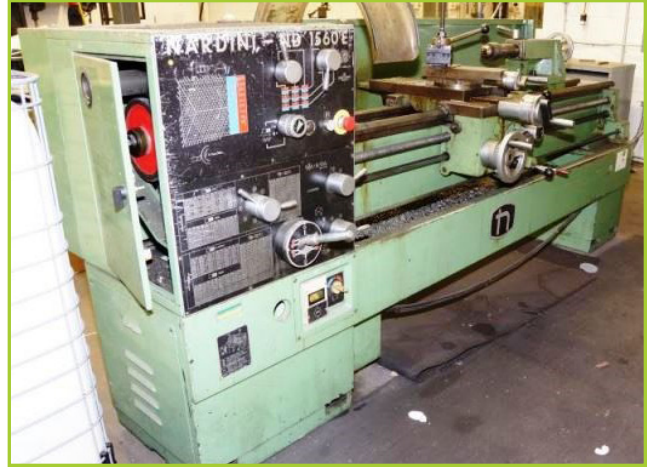
NARDINI ND 1560E 15" X 60" ENGINE LATHE. 54 MM SPINDLE BORE. D-6 SPINDLE MOUNT. 3 & 4 JAW CHUCKS. 5 C COLLETS AND PULLER. TOOL POST. TAIL STOCK. STEADY AND FOLLOW RESTS. 18 SPINDLE SPEEDS 25 TO 2,000 RPM. CARRIAGE STOP
