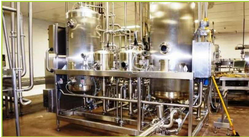
MICROBLEND MIX PROCESS SYSTEM. (2) WALKER 316 L STAINLESS STEEL JACKETED PRESSURE VESSELS. (4) PUMPS. (1) 30 HP AND (3) 7.5 HP ASSORTED BLENDING VALVES AND CONTROLS. YEAR OF MFG. 2003 AND 2004
