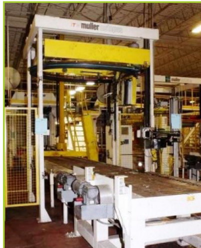
MULLER 404-OCTOPUS ORBITAL STYLE STRETCH WRAPPER. CAPY 4' WIDE BY 6' HIGH
