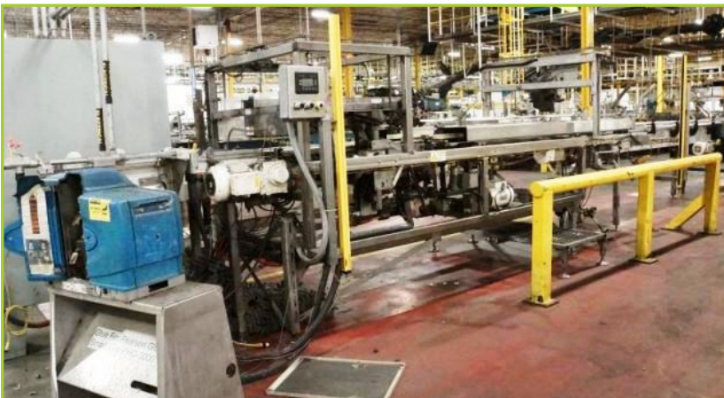
RA PEARSON C2240 FRIDGE PACK CARTON COMBINER. NORDSON HOT MELT GLUE MACHINE
