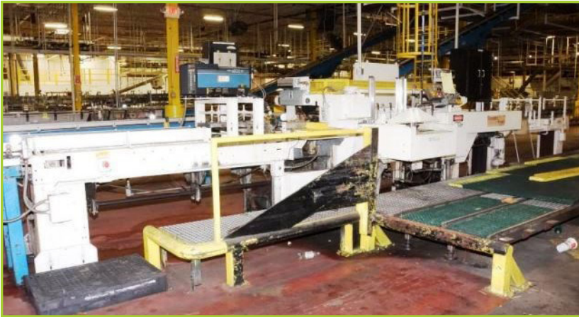
STANDARD KNAPP 263 24 CAN TRAY LOADER PACKER. NORDSON 3500 V HOT MELT GLUE SYSTEM
