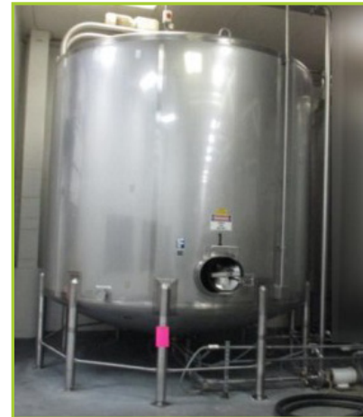
FELDMEIER 10,000-GALLON TOP AGITATED MIXING TANK. [TANK ID# 1 ; S/N-A-023-00 ; YEAR 2000. STAINLESS STEEL ; APPROX 128" STRAIGHTSIDE X 144" DIAMETER. WITH 7.5-HP MIXER ; WITH FRISTAM/BALDOR 3-HP CENTRIFUGAL PUMP]
